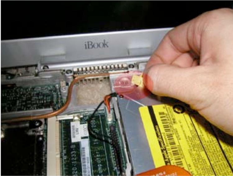
Flip the unit back over. If you have not removed the display, Locate the cd drive, and remove the yellow strip of tape holding the backlight cable to the drive.
