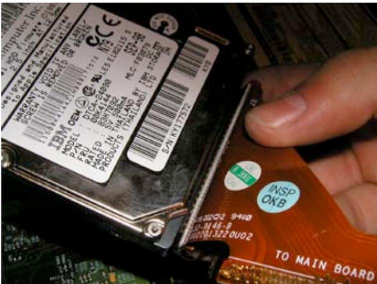
Remove the orange cable from the hard drive as shown. Pull the cable directly out or you risk bending the pins on the hard drive. Note that the cable for the hard drive says “TO HDD”
