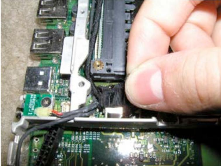
First, locate the hard drive, and undo the black strip of tape holding the microphone cable in place.
