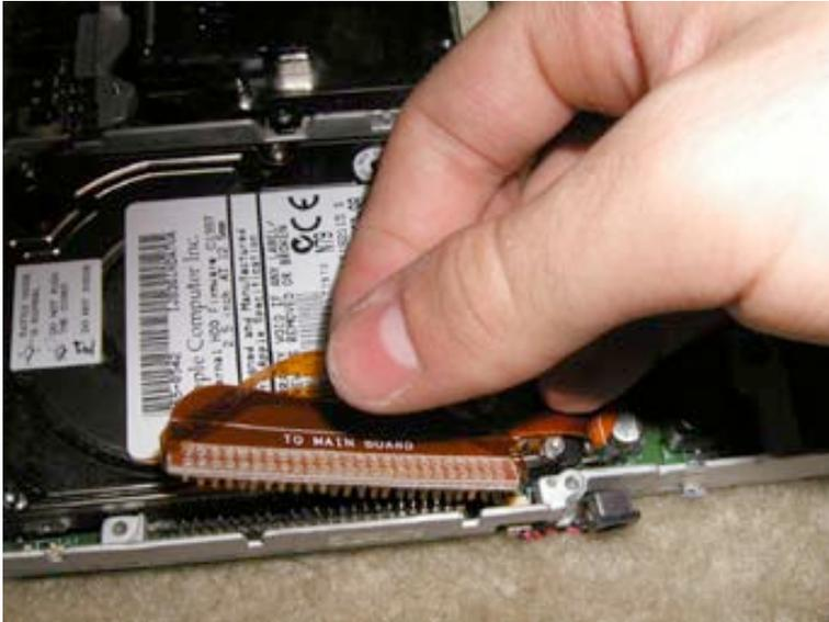
Disconnect the orange cable from the logic board as shown. Note that this cable says “To Main Board” on it.
