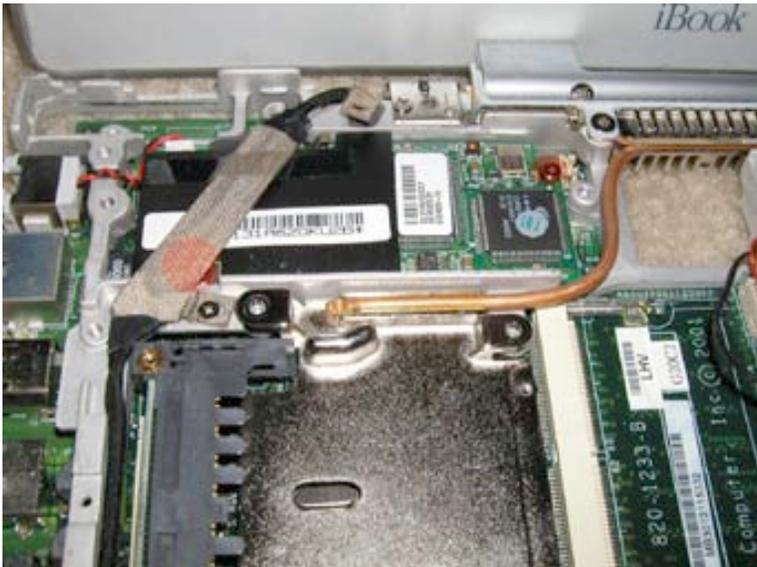
Remove the two Philips head screws as shown. (The red dot is shown on top of the cable, but the screw is underneath the cable.)
