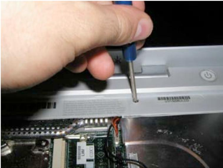
This will reveal another Philips head screw. Remove the screw as shown.
