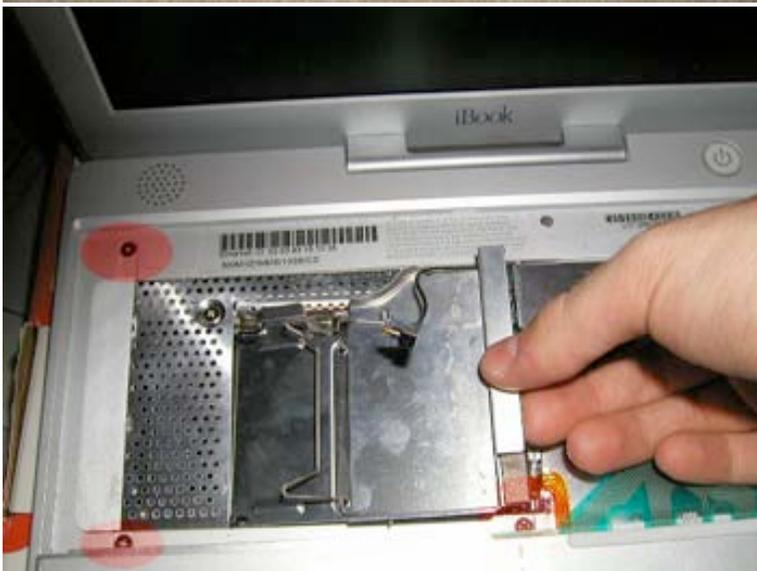
Remove the 3 philips head screws shown in red. (Ignore the hand in the picture.)
