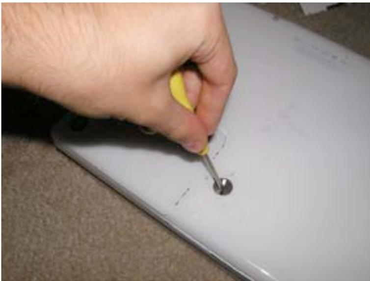
Using either a flat head screwdriver or a coin (anything with a flat surface) turn the security latch to the left as shown. Turn it until the notch is facing the “unlock graphic.”
