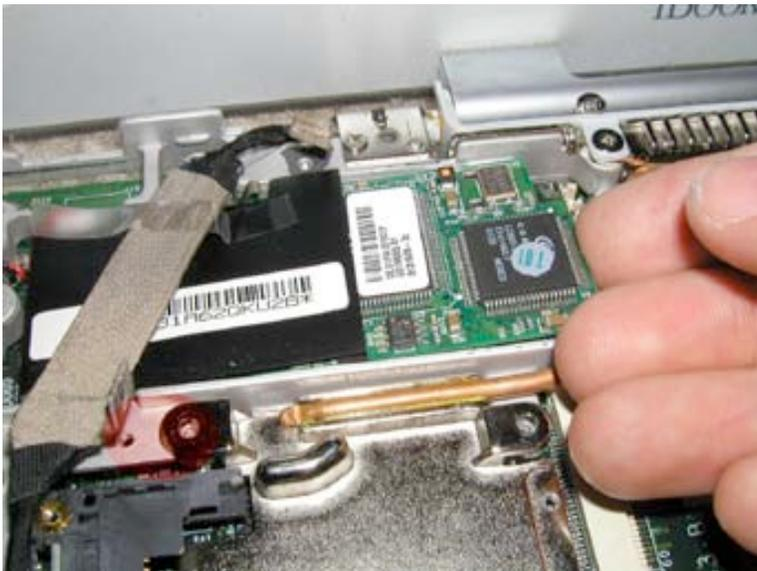
If you have not done so in a previous step, remove the Philips head screw in the location shown. Also, if you have not done so already, remove the piece of tape connecting the display cable to the modem. (See modem removal for more information.)
