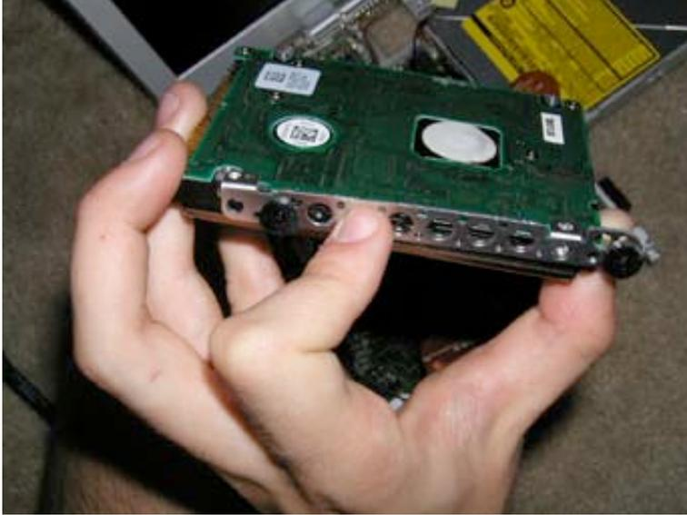
On the side of the drive is a metal plate with two rubber washers. This is on both sides. Make sure to transfer these pieces to the new hard drive you are installing. (The rubber ends go over the black screws on both sides.)
