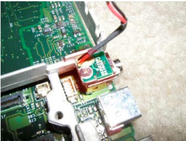
Locate the reset button next the USB and firewire ports. Remove the Philips head screw from the top of the rest button., and disconnect the cable from the logic board.
