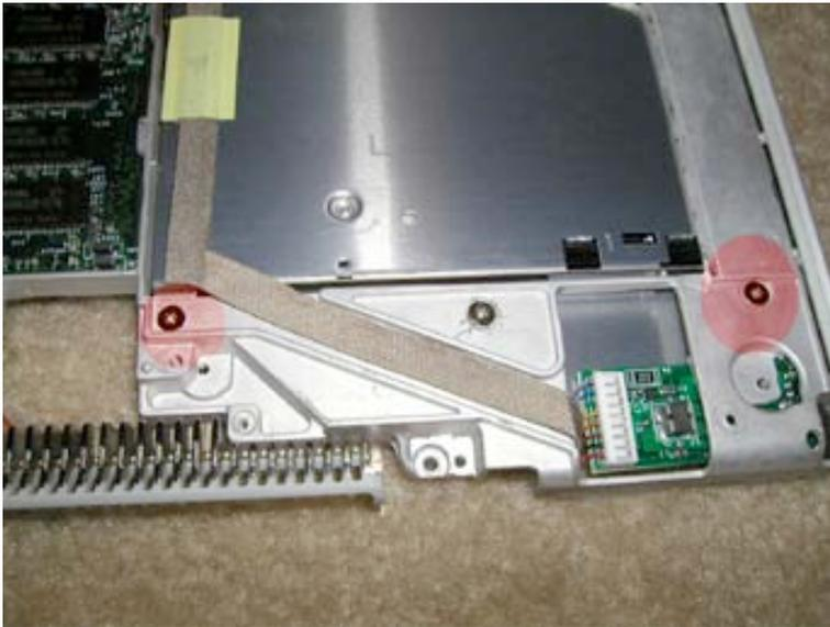
Flip the unit over and locate your cd drive. Locate the two Philips head screws shown in red, and remove them.
