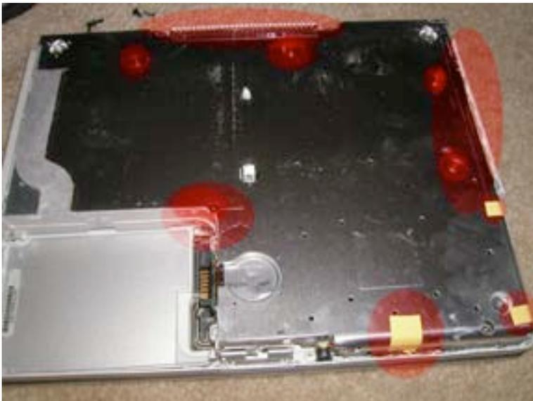
The bottom shield is held on with two long strips of grey tape, 3 pieces of yellow tape, and 5 philips head screws. Their locations are shown in the picture. Remove all of these pieces.
