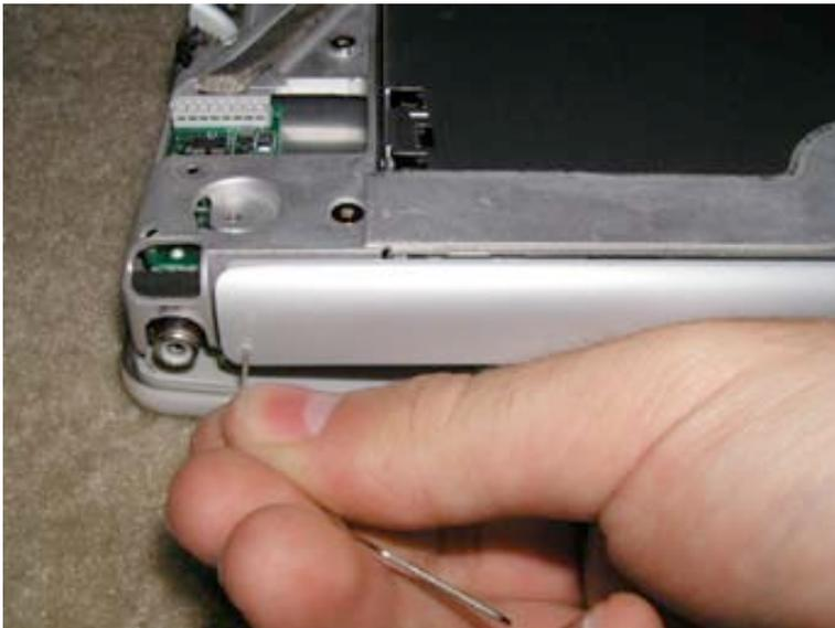
Flip your unit over now, and locate your cd or dvd drive. Use a paper clip to manually open the drive as shown. (Just stick the paper clip into the hole, and the drive will pop out.)
