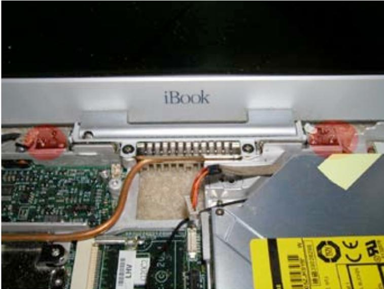
Remove the two Philips head screws in the location shown. Hold the monitor while you do this to prevent damage.
