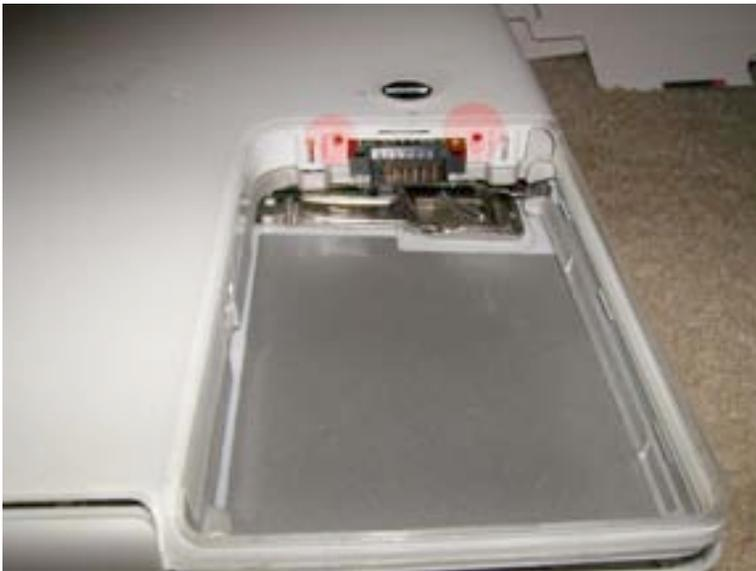
Locate two Philips head screws inside the battery bay, and remove them. The location is shown in the picture.
