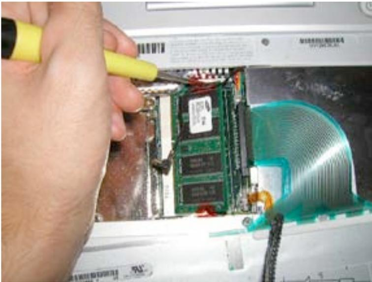
This step does not require removal of the keyboard. To remove ram, gently pry back the two metal connectors on each side of the ram chip as shown. (Only one side is shown, but it is easier if both are pried back at the same time.) The ram chip will “pop” up. Grasp it, and gently pull it out of its socket.
