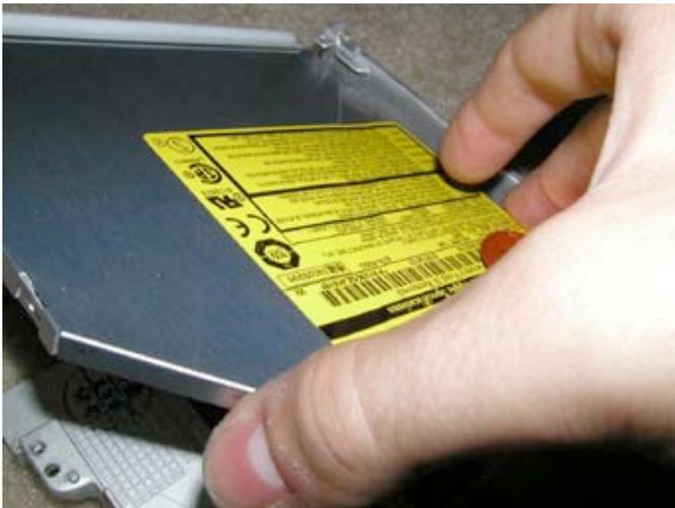
Grab the drive by the sides ONLY as shown. Tilt the drive up and then out.
