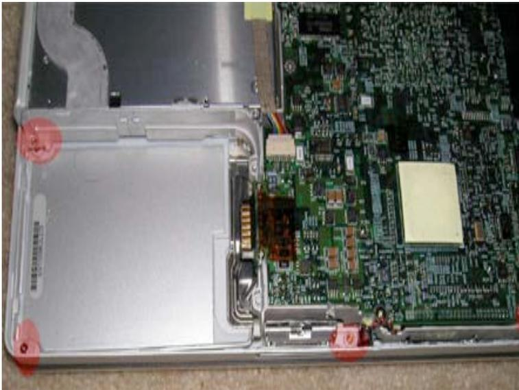
Note: You do not have to remove the bottom shield or fan to remove the top case.
