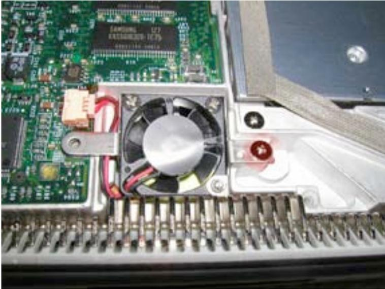
Locate the internal fan. (It is near the cd drive) Remove the one Philips head screw as shown. Lift the fan up and out, and then remove the fan cable from its connector.
