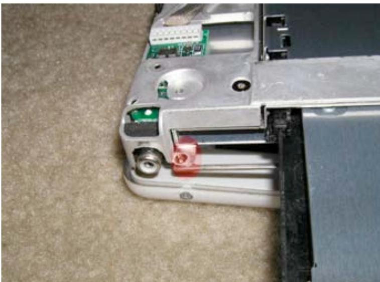
On both sides of the drive will be a small Philips head screw. Remove both screws. (The picture only shows one, but both need to be removed.)
