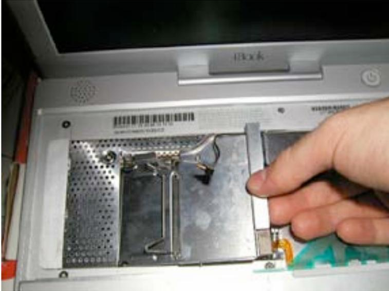
Lift the airport card holder up and out of the frame as shown.
