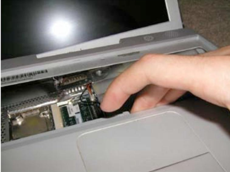
The top case will now be loose to lift up. (You won't be removing the trackpad yet.) Start on the top right hand corner near the AC input and DVD drive, and gently lift the case up.
