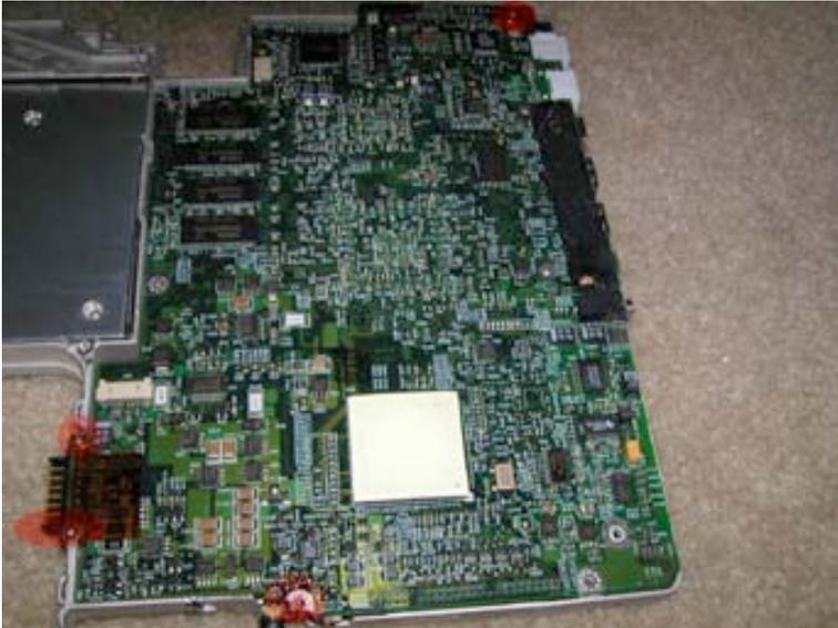
Turn the laptop over, and remove the four Philips head screws from the locations shown.
