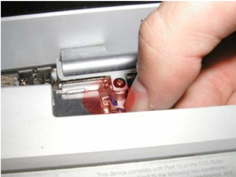
Undo the power button cord (the blue and white cable) from the logic board.)
