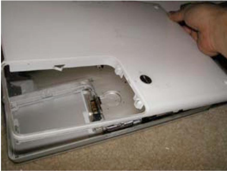
Gently work your way around the case. In some parts you may have to use a flathead screwdriver to release the tension around the case. The bottom does not come out easily, and you may have to work at it for a while.
