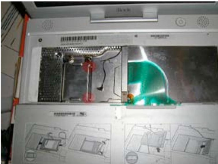
Remove the two Philips head screws as shown. (Note – If an airport card is installed, it will have to be removed first. )
