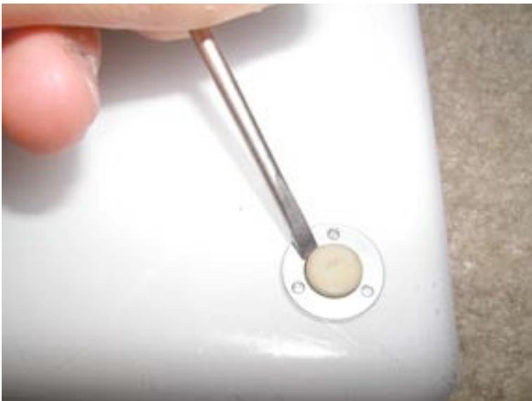
Around the corner of the case, you will notice the bottom feet. Pry up these feet (plastic part only as shown) using a flat head screwdriver. Do not do this to the foot on the battery. Only do this to the 3 feet on the corners of the iBook.
