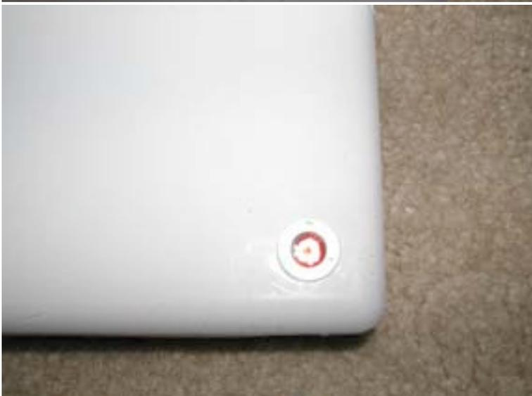
Remove the 3 philips head screws located under each of the feet.
