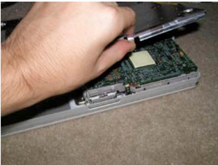
You can then lift the bottom shield up and off of the unit as shown.
