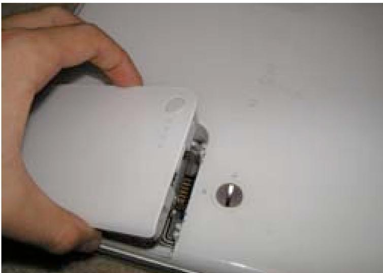
The battery will then pop up slightly. Grasp the battery as shown, and pull it up and out of the computer.
