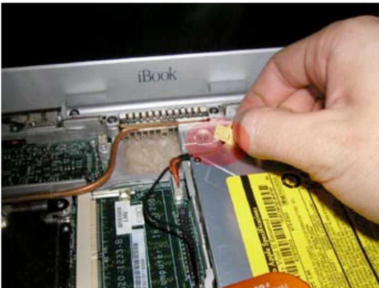
Locate the cd drive, and remove the yellow strip of tape holding the backlight cable to the drive.
