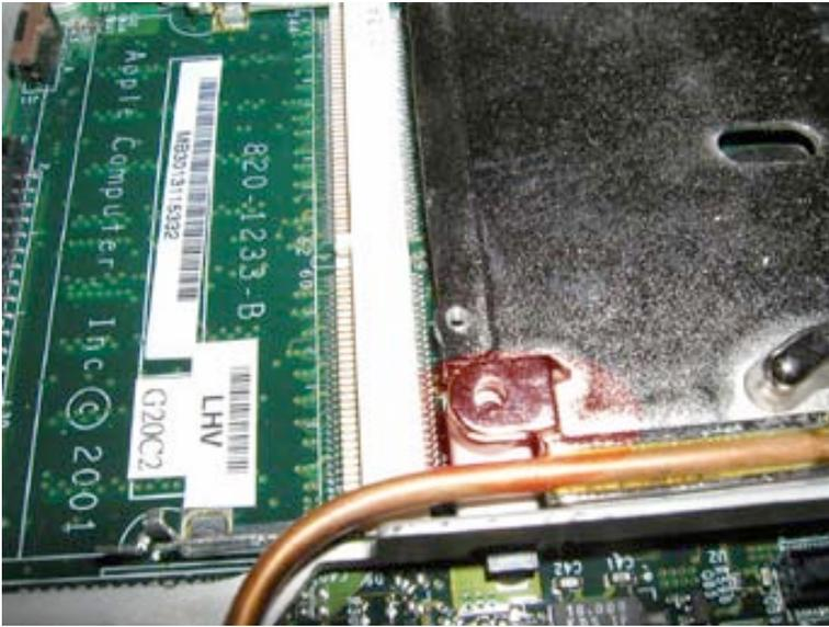
Remove the last screw from the heat spreader as shown.
