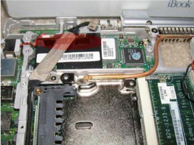
Remove the strip of tape holding the display cable to the modem. Be extremely careful with the display cable. You do not want to put this cable under a lot of stress.
