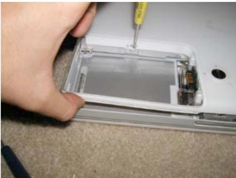
In the battery bay there is a plastic latch which holds the casing on. Use a flathead screwdriver to gently pry this out, and pull up from the corner at the same time. Do not use excessive force or you will break your case! Be careful!
