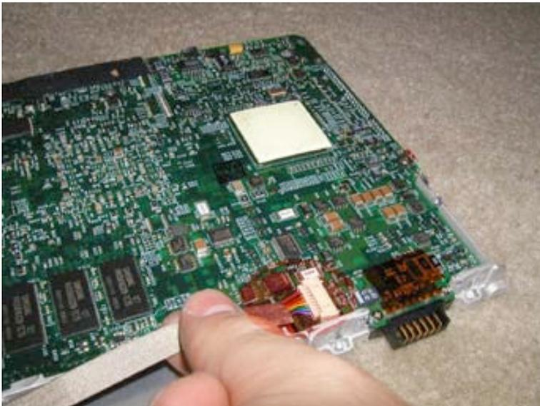
Turn the unit back over, and remove the DC board cable from its connector as show. (It is the multi colored wire that was previously taped to the CD/DVD drive.)
