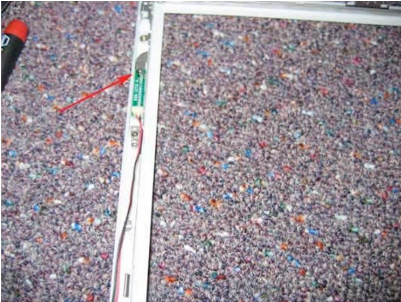
Begin by removing the Philips head screw in the location shown.
