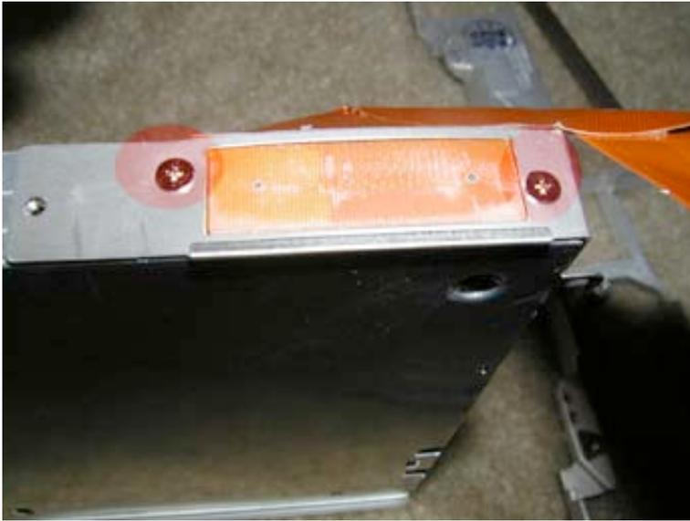
On the back of the drive, locate the two Philips head screws shown in red and remove them. Disconnect the cable, and note that the cable says “TO CD ROM” This is so you don’t confuse it in reassembly.
