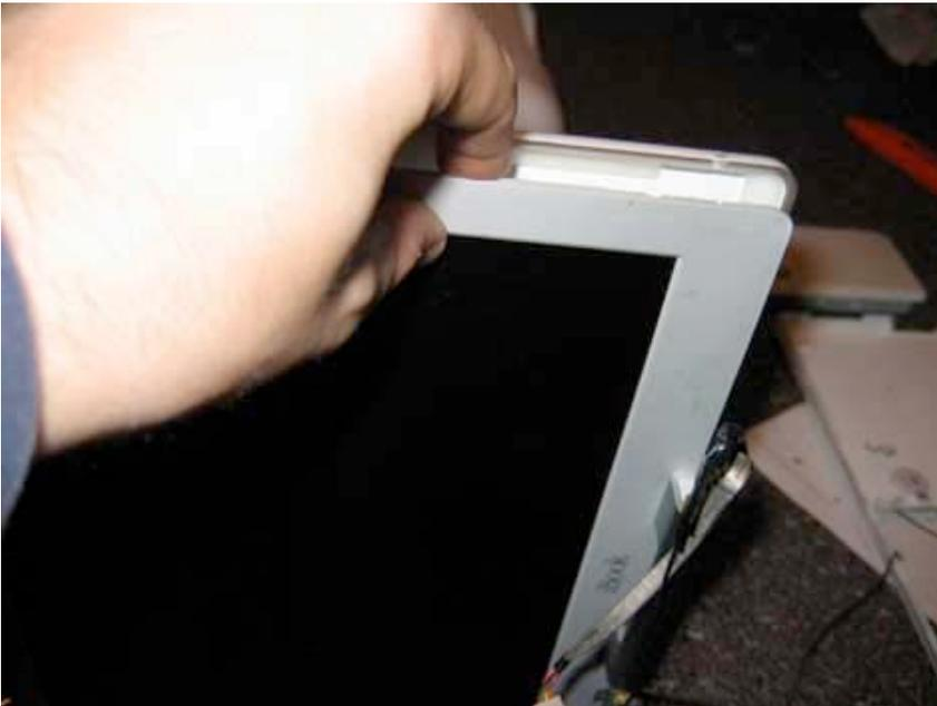
Next, you will need to pry the back panel (case with Apple logo) off. It is best to start at a corner as shown, and pull the casing in the opposite direction as the LCD. You may need to use a flat too to help you at first. After you get started, the casing will come off easily.
