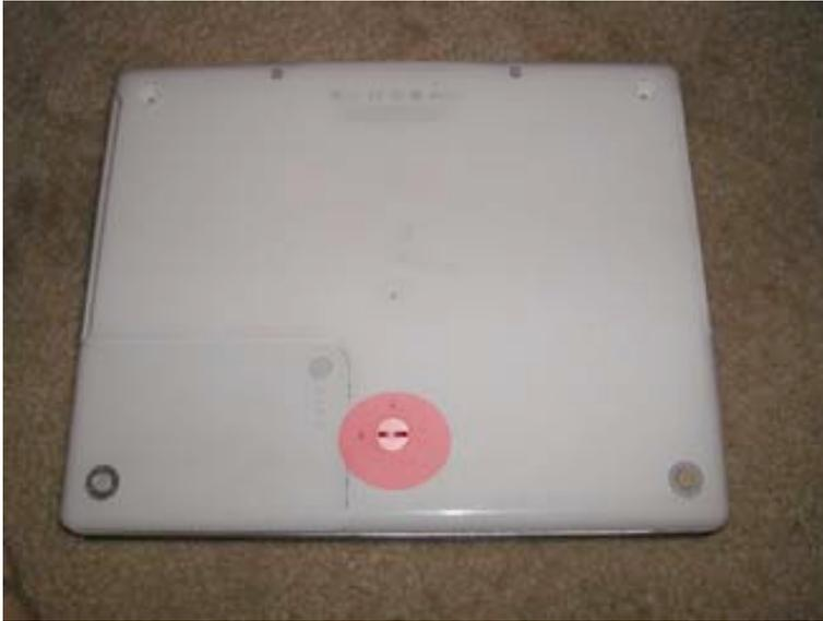
Removing the battery is the first step of any repair. First, unplug your unit. Then, close the display (if open) and turn the unit over. Locate the battery lock as shown in red in the picture.
