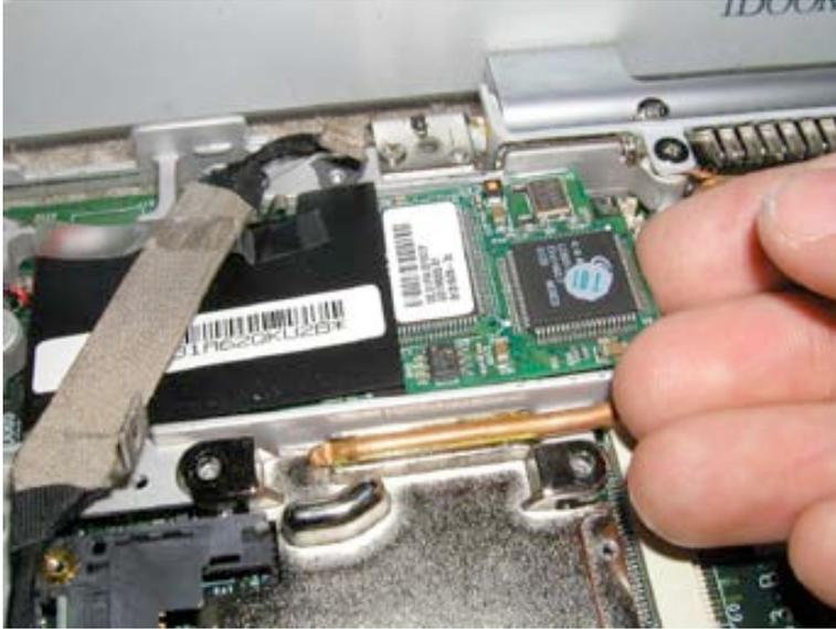
Tilt the modem up and out as shown.
