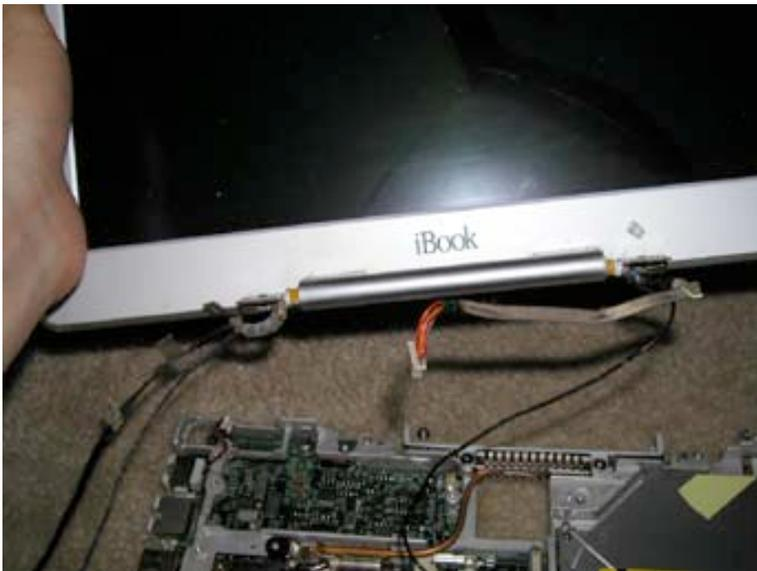
Lift the display module up and out of the computer. If a cable is stuck, do not pull on it, gently work it up and out. Never pull!
