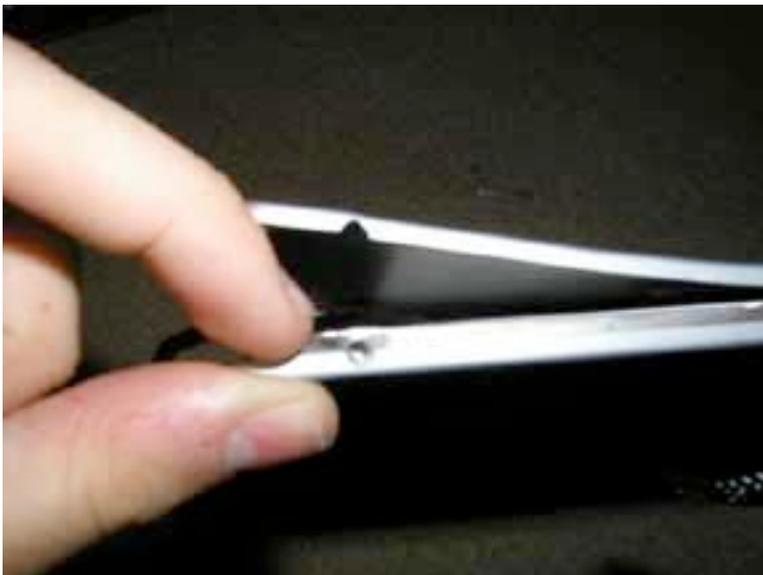
A lot of times, you will damage the thin piece of metal that connects the top casing to the bottom casing. When you close your display back, it will normally go back into position, but you may have to prod it in certain places with a flat head screwdriver to allow the casing to close correctly.
