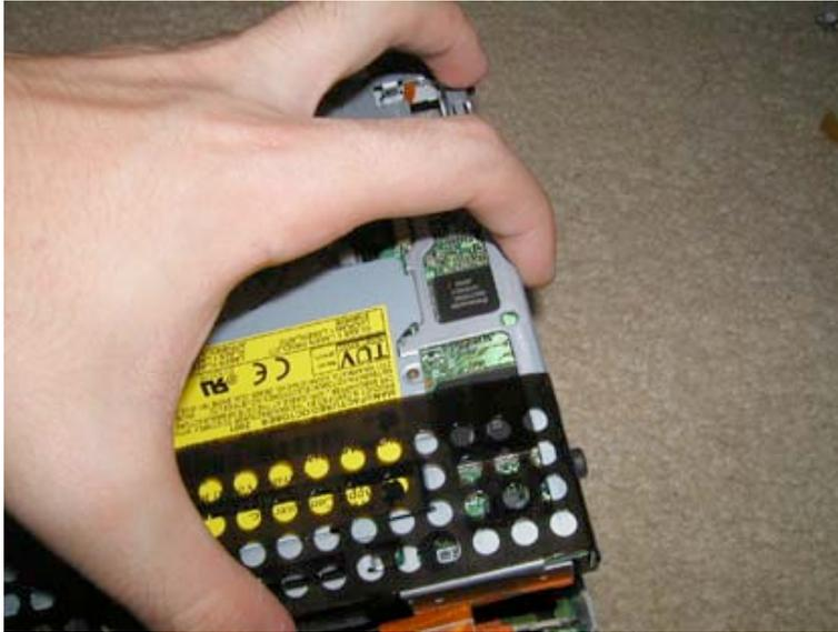
Grabbing the drive from the sides only, lift the drive up and out.
