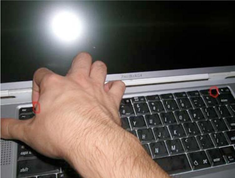
After you have removed the battery, turn the computer over and open up the display. Then, depress the two keyboard tabs as shown in the picture. Holding the tabs in, flip the keyboard up and towards you. (If the keyboard does not easily come out, check to make sure you have not locked the keyboard.)
