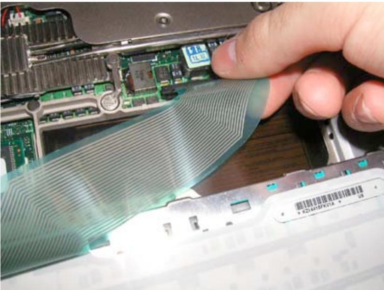
To remove the keyboard connector, grasp the cable as shown and gently pull up. You can gently wiggle the cable from side to side if it doesn't come off easily. Do not use much force. It should come off relatively easily.
