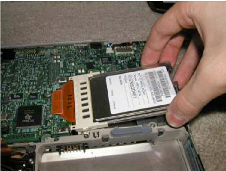
Lift up on the card as shown. Then pull the card out of its connector. (You may gently rock the card side to side to ease it out of the connector.)
