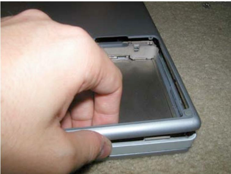
Gently lift up on the case as shown. Do not use much force at all or you will break the trackpad casing. Gently work your way around the casing.
