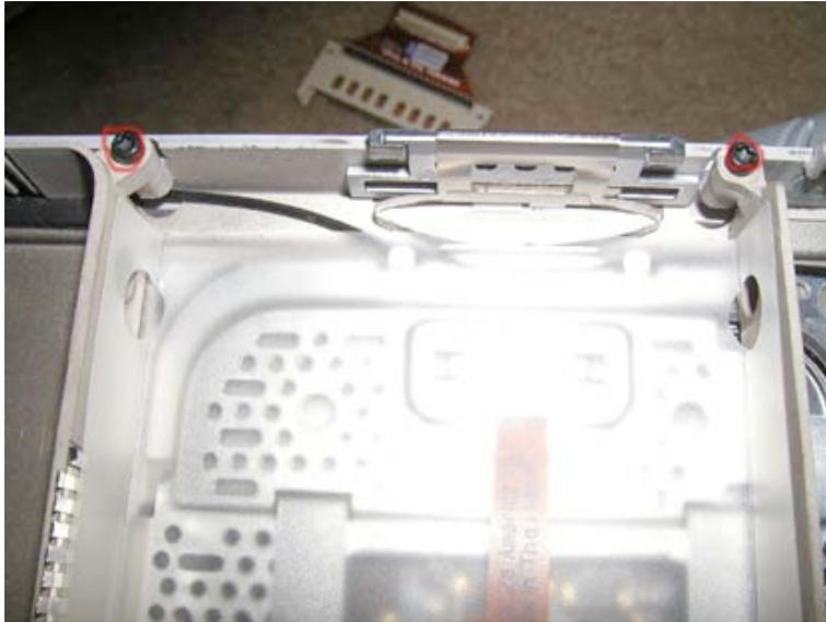
Along the rib frame there are 4 small torx T8 screws. The two shown to the left are in the hard drive cage. The one in the picture below is under the airport cable near where the airport card goes. The last picture is hard to tell, but it is near the inverter board on the left hand side of the casing.
