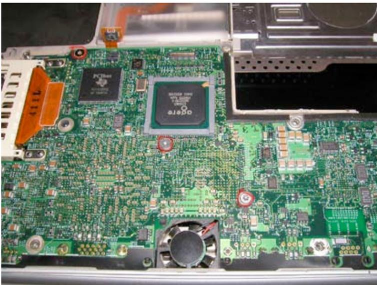
Remove the three Torx T8 screws as shown.
