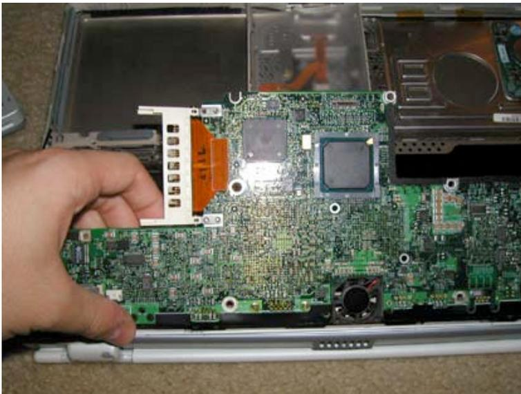
Grasp the logic board as shown and gently pull up. Then gently pull the board out and place it on an anti-static surface.
