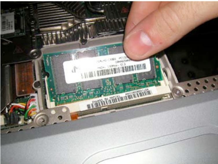
The ram chip will pop up. Just slide out to remove it. To install a new chip, just align the new chip in the grooves, press in, and then press down until the fasteners clip on both sides.
