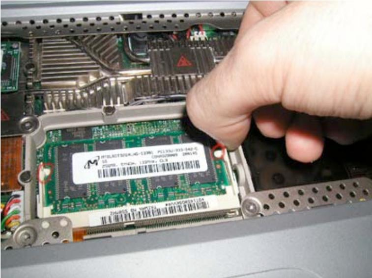
To remove currently installed ram, pry back the metal or plastic fasteners holding in the ram as shown. Do this on each side. It's easier if you do them at the same time.
