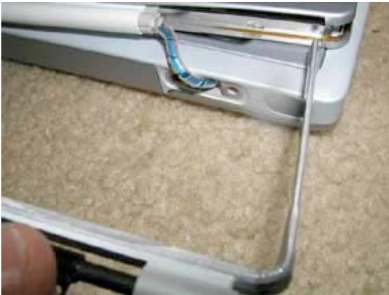
Line the epoxied hinge up with the hinge hole.
