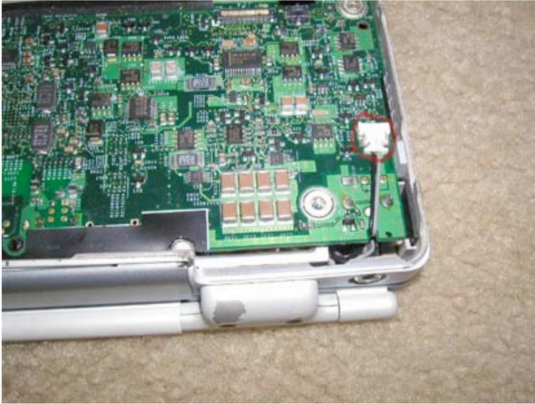
Remove the orange piece of tape covering the black and grey cable on the right hand side of the logic board.
