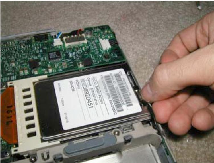
To remove the airport card, locate the metal clip that holds the cable connector in place. Gently pry this back with your finger and pull up on the cable to release it from the connector.
