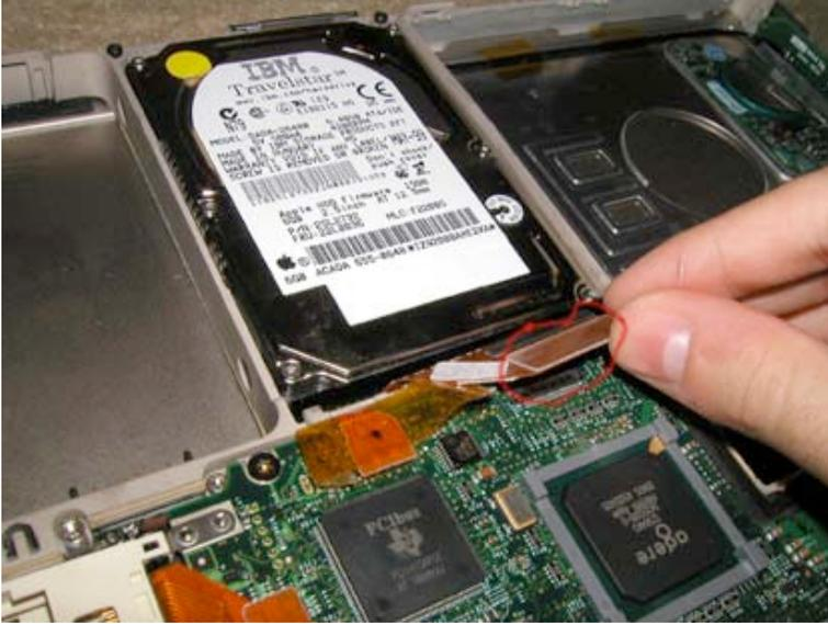
Disconnect the orange hard drive cable from the motherboard as shown.
