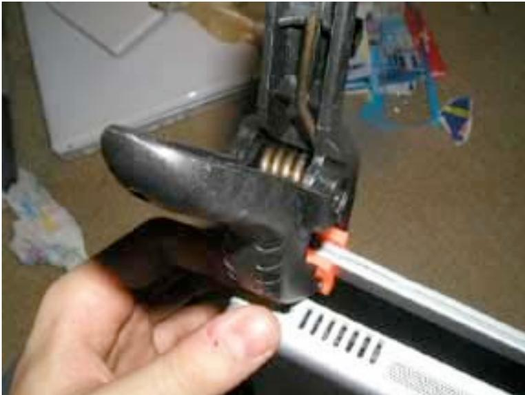
Use a strong spring clamp (available at Wal-mart) to clamp the display shut. Only clamp the edge of the display! Do not put the clamp on the actual LCD or you will break it. Let the epoxy sit for 24 hours or as the instructions say. 24 hours is a good time to let the epoxy sit however.
