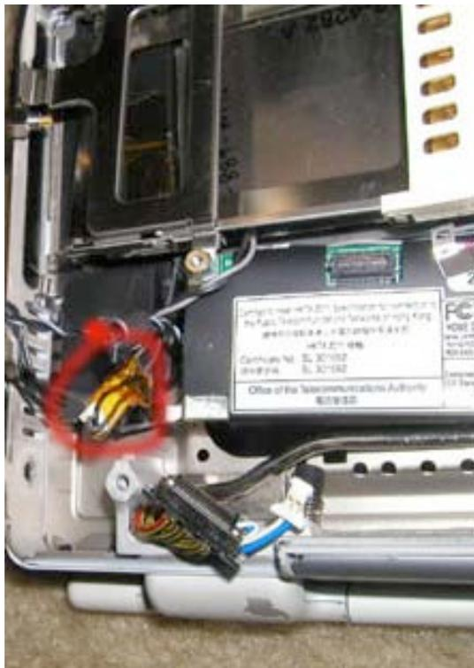
Disconnect the audio cable on the left hand side and right hand side of the unit. If it is wrapped in orange tape, remove the orange tape.
