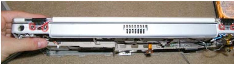
Now, remove the 4 Torx T8 head screws at the locations shown. Do not remove the black screws on the black hinge. \*Be very careful around the cables.
