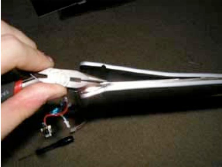
Use a pair of needle nose pliers to extract the hinge when it is loose enough to be pulled out.
