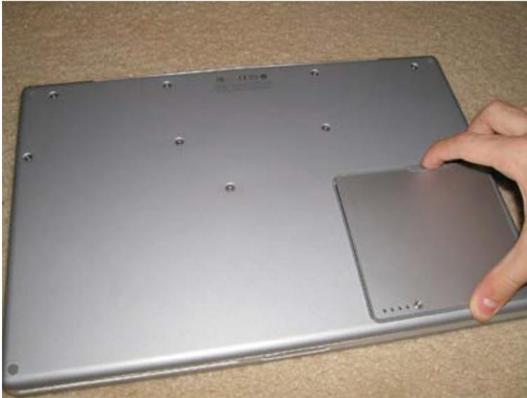
Turn the computer over with the bottom up as shown. Push the battery latch to the right as shown. The battery will then “pop” up and you will be able to remove it from the laptop as shown in the second picture.
