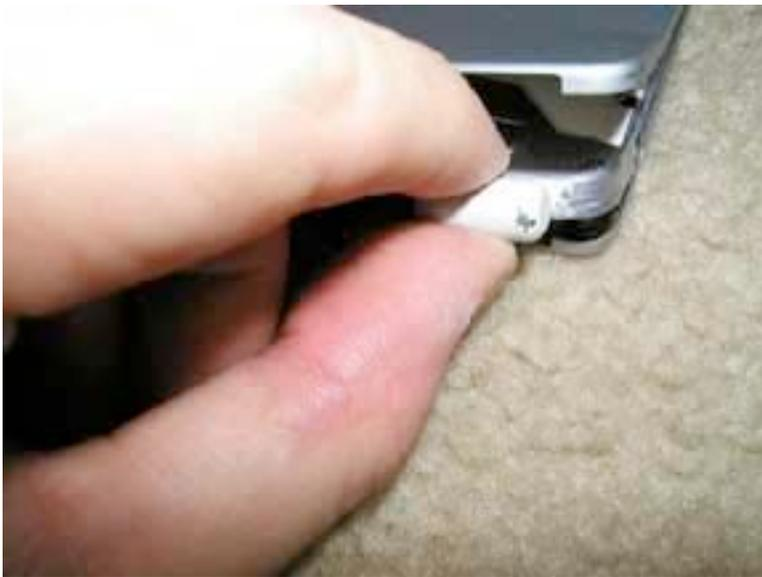
If you haven't done so already, follow the instructions above to break the bond on about 3-4" of the casing on the side of the casing of the hinge you need to replace.
