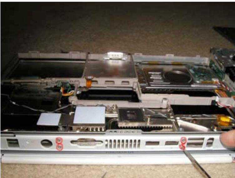
Remove the 4 Torx T6 Screws near the ports as shown.
