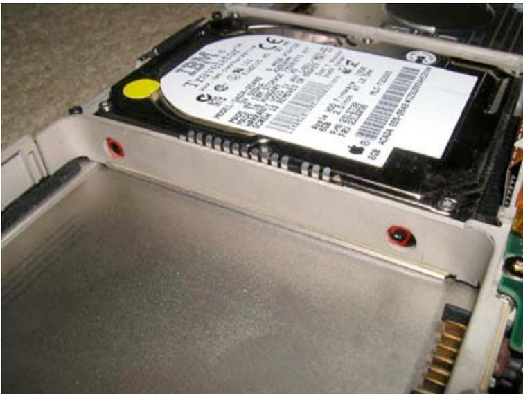
Remove the two Torx T8 screws shown in red. These are located in the battery bay. Note – There are two rubber washers, if they fall out remember to put them back in when installing a new drive.
