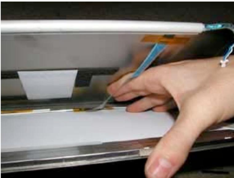
From the base of the display, open the display as shown. You'll notice there is an orange piece of tape holding the display cable to the display connector. You will need to remove this piece of tape as well as the piece holding the cable on closer to the bottom of the display. You will then be able to remove the cable from its connector.
