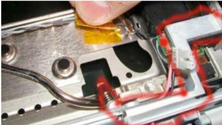
On both sides of the casing is the piece shown in red. This piece pivots up and “folds” over. On the side with the display cable and white and blue wire, lift this piece up, and then, carefully guide the display cable and blue and white cable through the hole. You will have to turn the display data cable to get it properly go through the hole. Be very careful with the cables!
