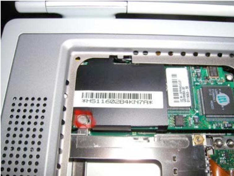
To remove the modem you will need either a pair of pliers or a 5mm hex nut screwdriver or wrench. Undo the hex nut in the location shown. Then pull the modem up to disconnect it from the motherboard. Lastly remove the cable connected to the modem.
