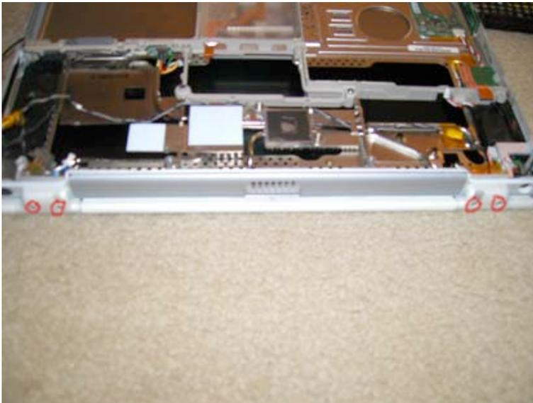
Remove the 4 Torx T8 screws on the clutch covers as shown.
