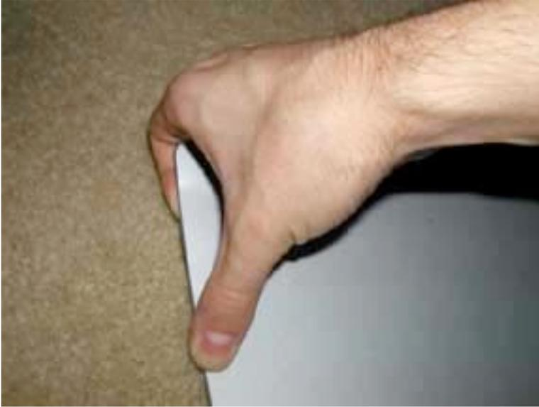
After the initial bond is broken, you need to work your way around the display to break the bond. Do this slowly. If you try to do too much at one time you'll dent your display casing. Again, only grasp from the sides. If you are performing the hinge repair only break the bond up to about 3-4" along the side...you want to break the bond as little as possible as it will be a cleaner repair when you are done.
