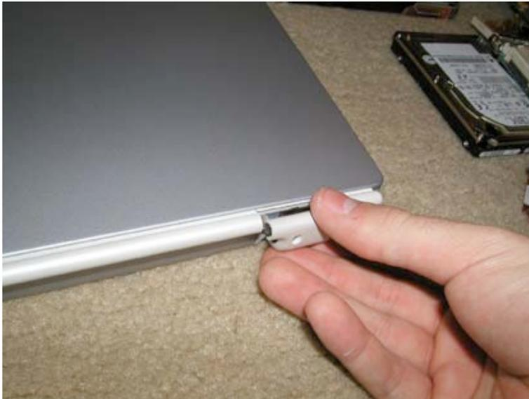
Gently pry the clutch covers off of the frame. If you use a flathead screwdriver be sure not to chip your paint. They should come off easily.
