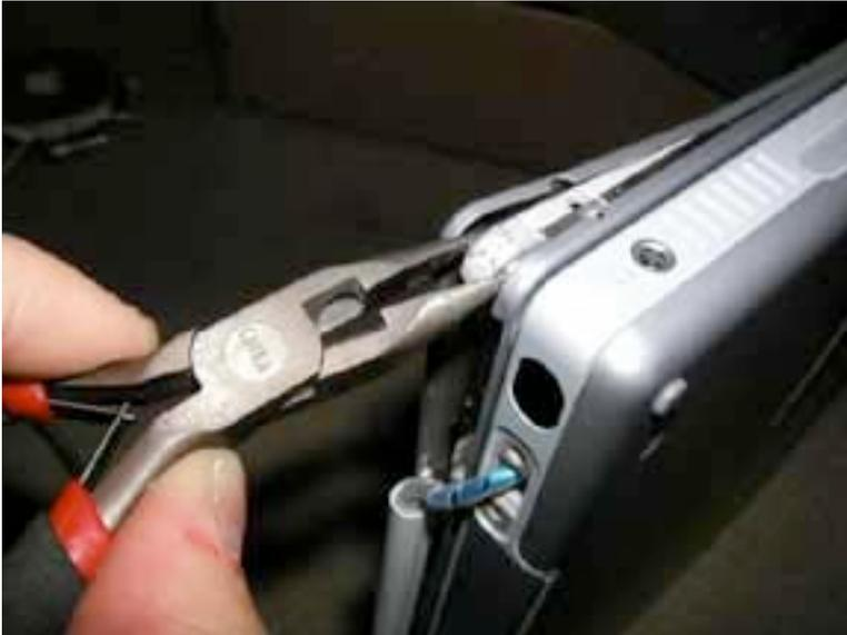
Use a pair of need nose pliers to pull the hinge towards you and out. Note: Do not use much force. You want the hinge to come out easily. If you use too much force the hinge will break and extraction will be much more difficult.
