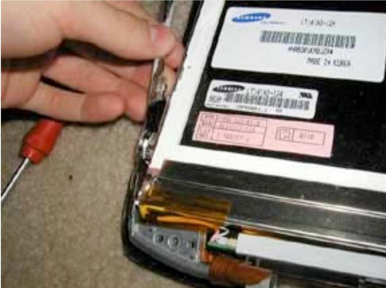
Guide the hinge to the left from under the display, then lift it up and free from the casing as shown.
