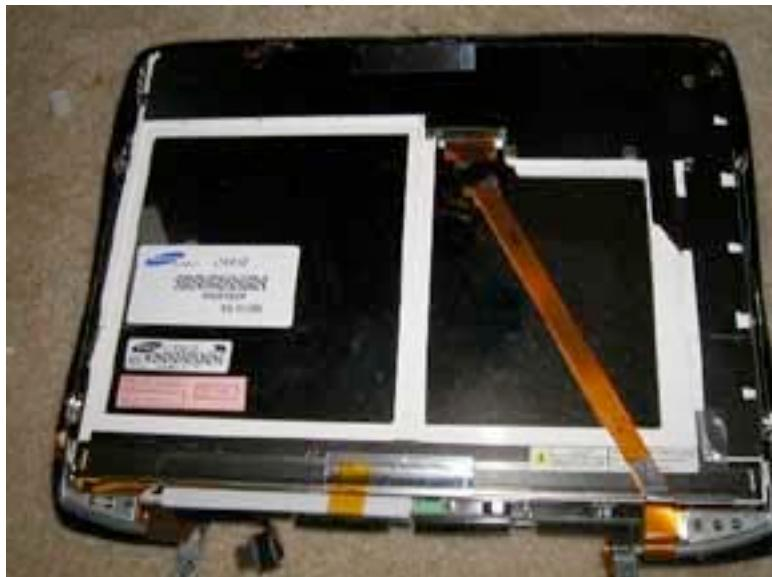
This is what you should be looking at after removing the back case.
