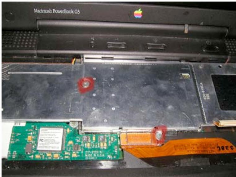
Remove the one Philips head screw as shown. Being careful again not to strip the screw.
