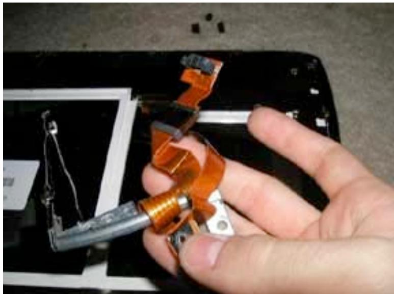
The display cable is wound around the hinge. You will need to unwind it from the hinge to remove it. When you replace the hinge or display cable, make sure to wind it back around the hinge.
