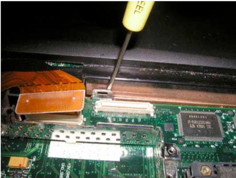
If the trackpad is having problems coming off, make sure it is not caught on the latch next to the PMU cable as shown. (It is in front of the processor near the trackpad. If it is caught, use a flat head screw driver to undo the latch, and pull up on the trackpad.
