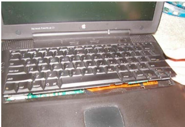
Lift the keyboard up and pull towards you to free the metal locks on the top of the keyboard. Then flip the keyboard out towards you.
