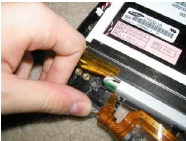
The inverter cable is held onto the hinge by two little holes with a small metal rod. Simply pull this part of the cable off of the hinge as shown in the picture.
