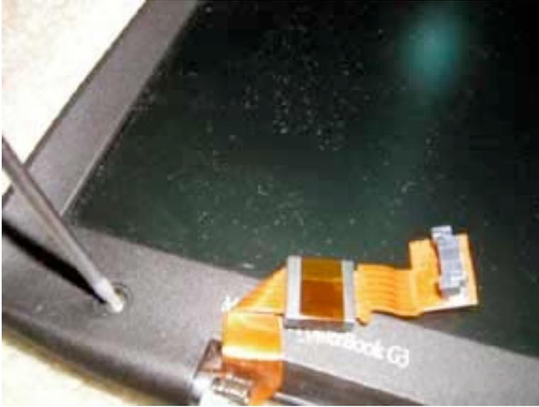
Remove the 6 torx screws at each of the 6 locations you have removed the cover from using your Torx T8 screwdriver. (Available from [Powerbookmedic.com](http://Powerbookmedic.com))
