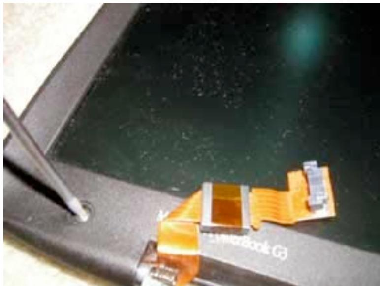
Remove the 6 torx screws at each of the 6 locations you have removed the cover from using your Torx T8 scredriver. (Available from Powerbookmedic.com)
