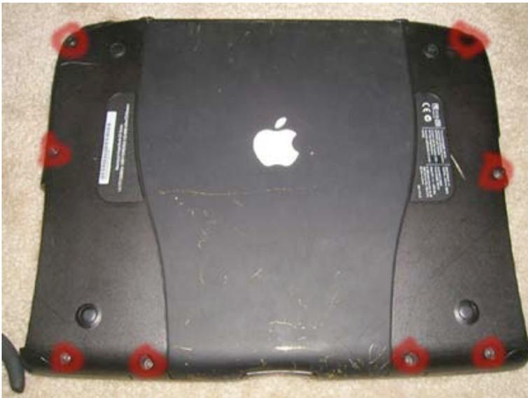
Turn the unit over, and remove the 8 torx screws as shown from the bottom casing.
