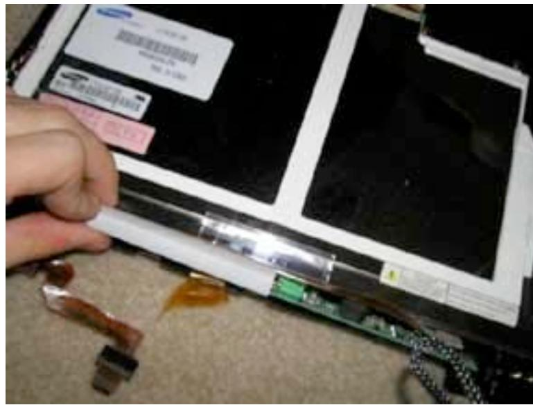
Now lift the inverter board up and out.
