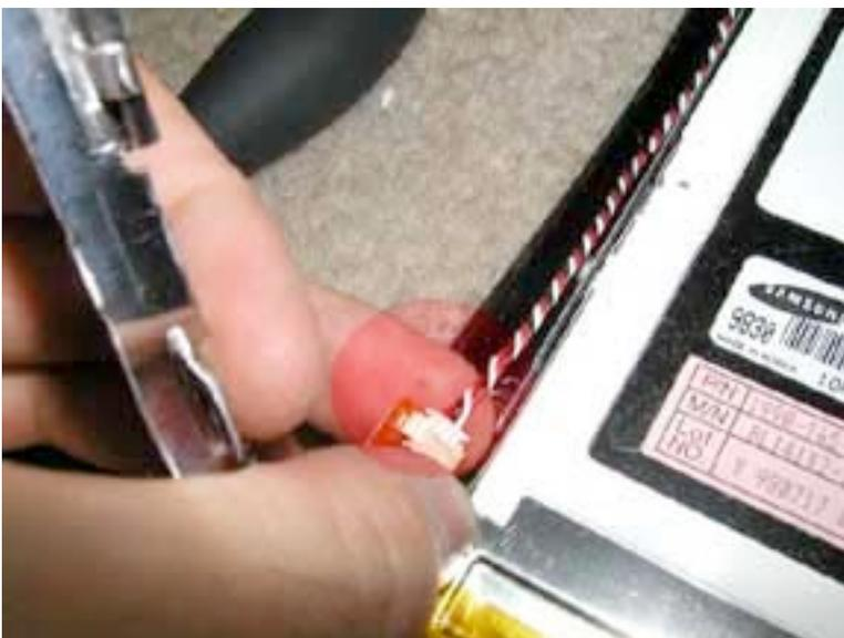
Remove the orange and white mic cable from the inverter cable as shown.
