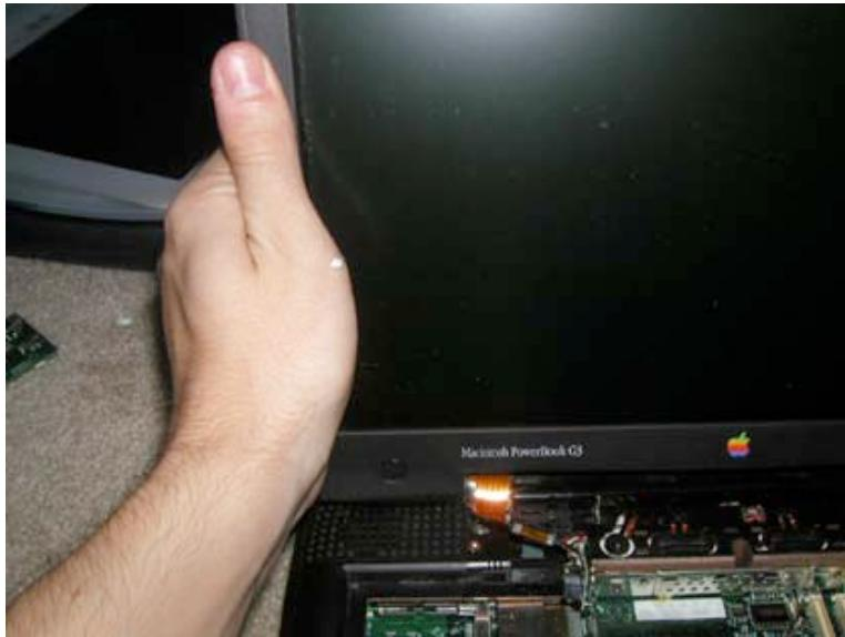
Now, pull the display back up so it is perfectly vertical. Place your hands on the right hand and left hand side of the monitor, and lift the display out of the casing.
