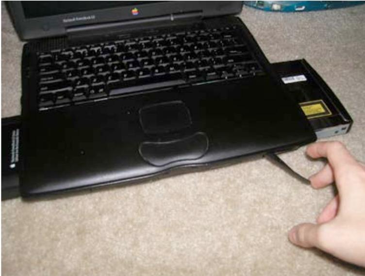
Begin by removing any expansion bays you have installed. Simply pull the expansion bay lever towards you to eject the device. Then pull the device out so the bays are completely empty.
