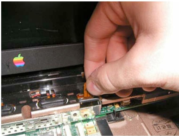
Grasp the orange display cable on the right of the laptop as shown. Gently pull up to undo it from the motherboard.
