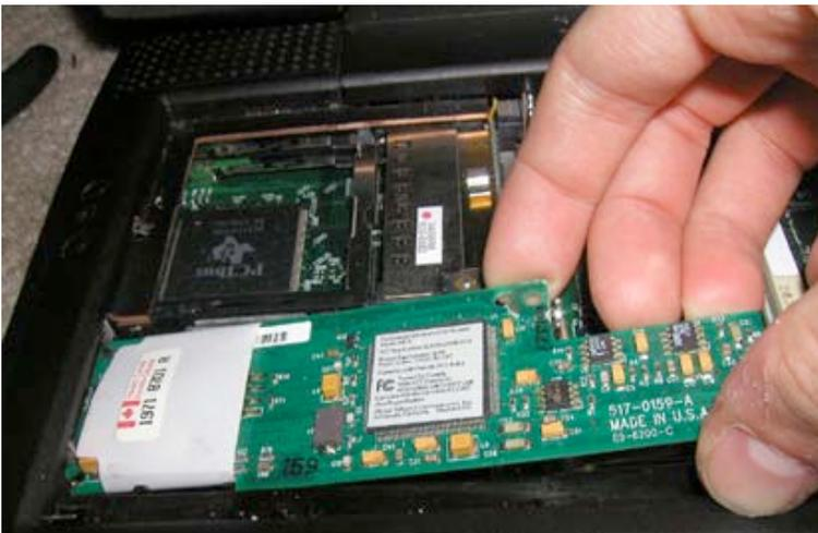
Lift the modem up and out as shown.
