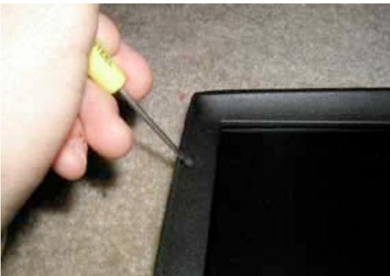
After removing the coverings on the bottom, remove the 4 rubber inserts simply inserting a flat head tool and prying up. The inserts should come out easily. Remove all 4 and then continue.
