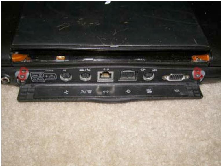
Using a Torx T8 screwdriver (available from [www.powerbookmedic.com](http://www.powerbookmedic.com)) , remove the four flathead torx screws on the back of the unit as shown. (Replacement Note: These four screws have flat heads, not the rounded heads like the other torx screws, do not get them confused.)
