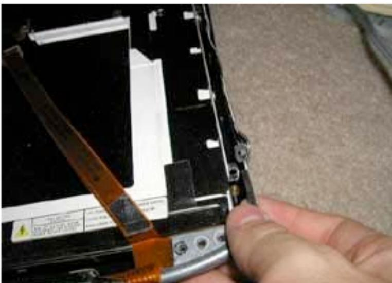
Guide the hinge to the right from under the display, then lift it up and free from the casing as shown.
