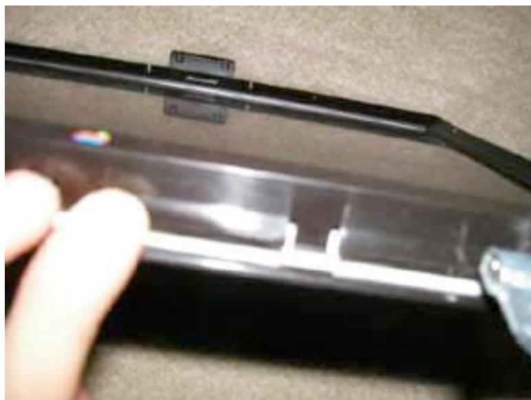
You now have to separate the back casing from the display. You will have to pry the casing free. It is easiest if you start from the spot right under the apple logo.
