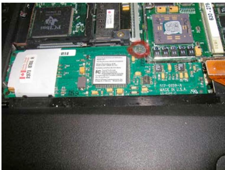
Lift the modem up and out as shown.
