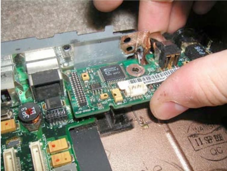
(Remove keyboard, heat sync, modem, processor, hard drive, display, and trackpad first)
