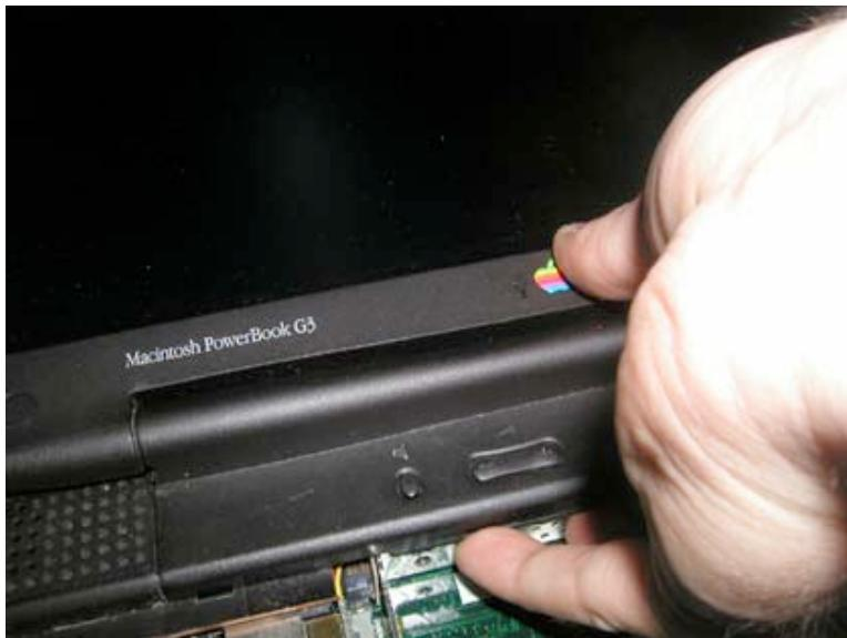
(Remove keyboard, heat sync, processor, and hard drive (optional) first )
