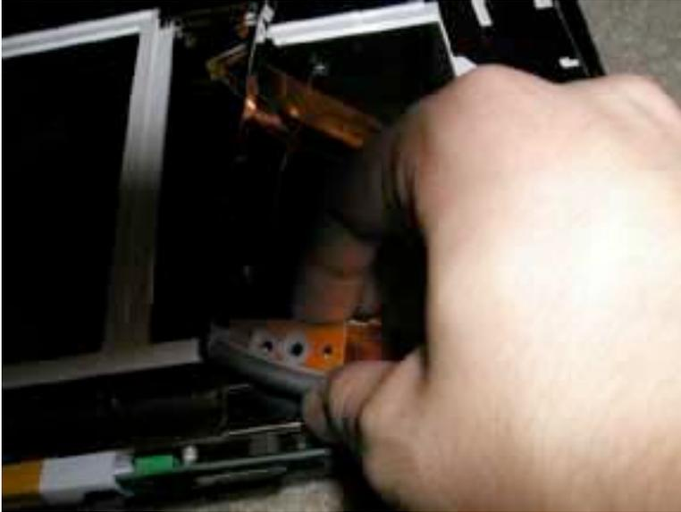
The display cable is held onto the hinge by two little holes with a small metal rod. Simply pull this part of the cable off of the hinge as shown in the picture.
