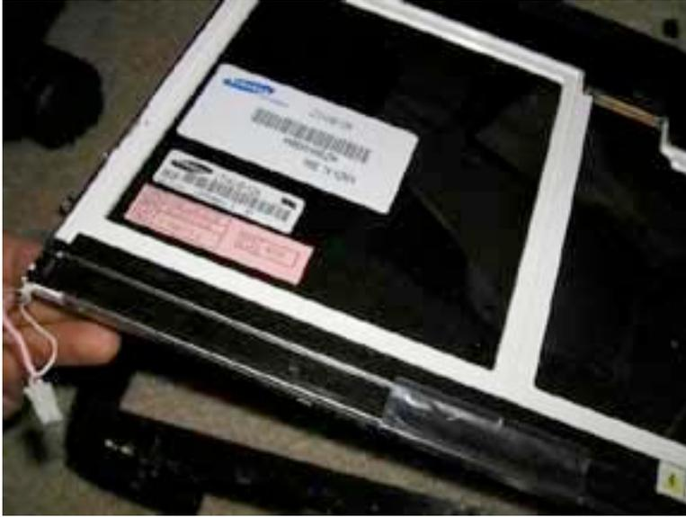
The LCD will now lift up and out of the front display bezel. To replace, simply place the new LCD with backlight into the display bezel, and follow the directions in reverse.
