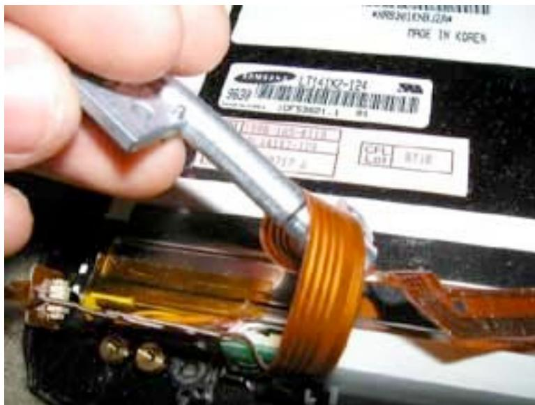
The inverter cable is wound around the hinge. You will need to unwind it from the hinge to remove it. When you replace the hinge or display cable, make sure to wind it back around the hinge.
