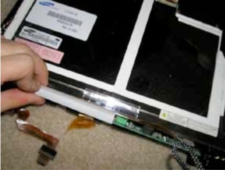
Now lift the inverter board up and out.
