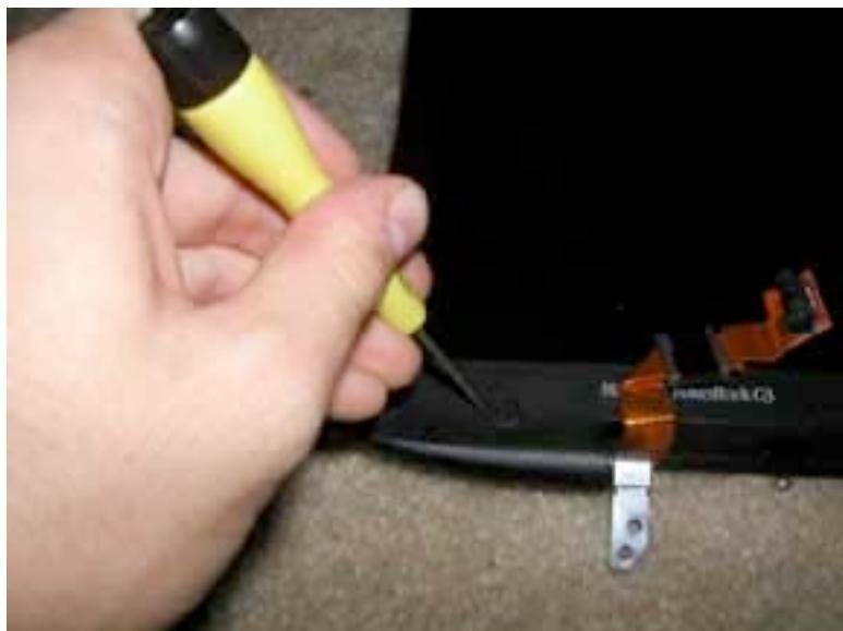
Using a flat head tool, pry up the flat plastic covering on the bottom of the display on either side of the cables. The left side is shown in the picture.
