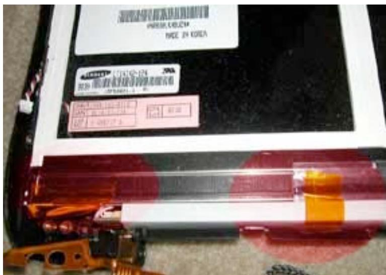
To remove the inverter cable, you will first need to remove the inverter board. Undo the two pieces of orange tape holding the inverter board to the LCD as shown.
