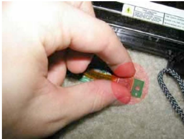
Undo the inverter cable from the inverter board as shown.
