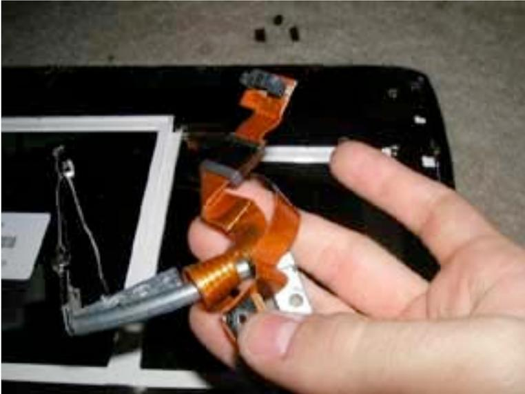
The display cable is wound around the hinge. You will need to unwind it from the hinge to remove it. When you replace the hinge or display cable, make your to wind it back around the hinge.
