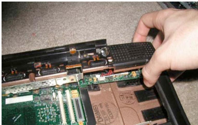
Starting at the top right hand corner, lift up to begin separating the trackpad.
