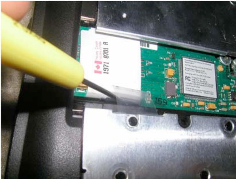
Undo the clear plastic tabs on the left and right side of the keyboard by sticking a flat head screwdriver behind the plastic while pulling up on the plastic. They should come out easily. (Replacement note – The clear tabs simply slide back into the groove. After you slide them in, they should “lock” in place.)
