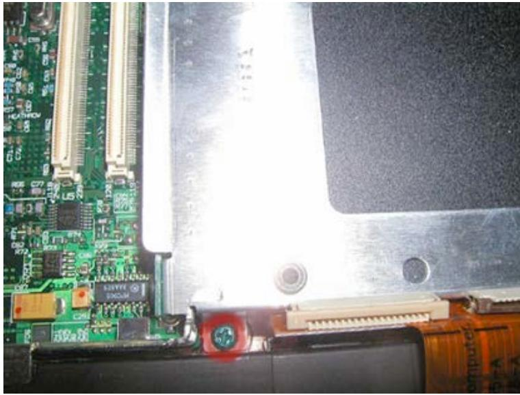
(Remove keyboard, heat sync, and processor first)
