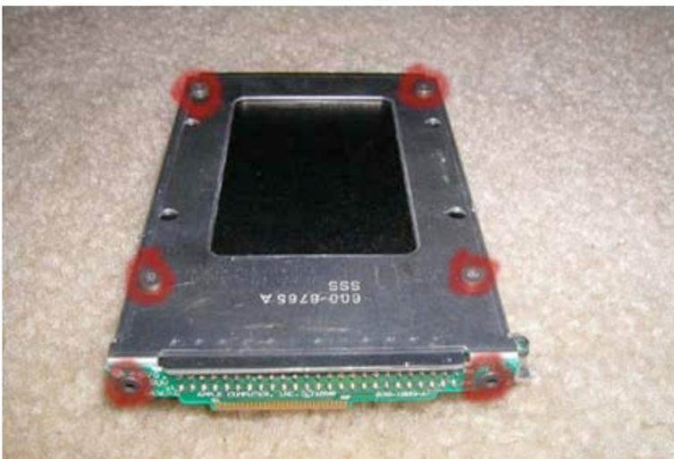
Remove the 6 Torx Screws as shown. Then, grasp the green motherboard connector by the sides and pull it towards you. It should come off easily. The hard drive will now easily come out of it's mounting bracket.
