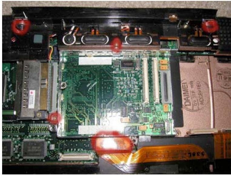
(Remove keyboard, heat sync, modem, processor, hard drive, and display first)
