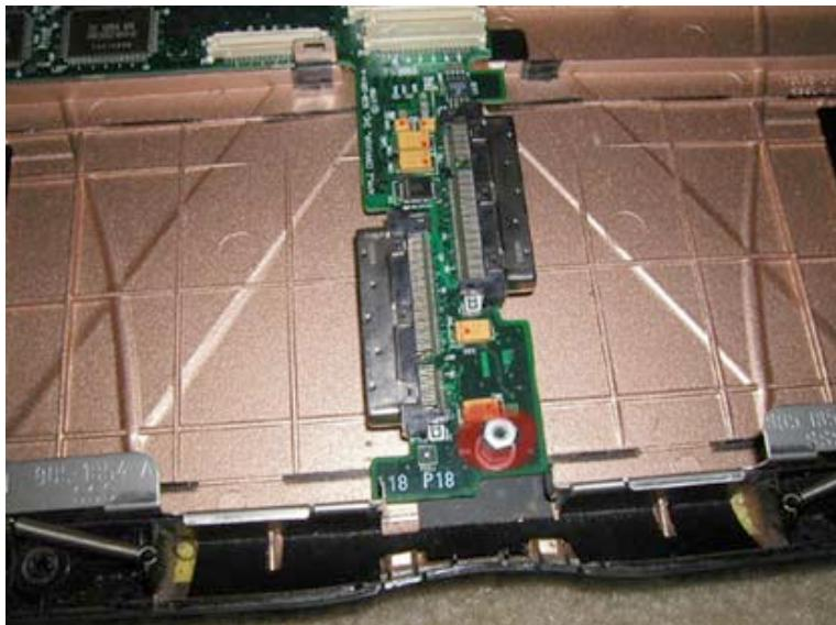
(Remove keyboard, heat sync, modem, processor, hard drive, display, trackpad, power board, and sound /AC board first.)
