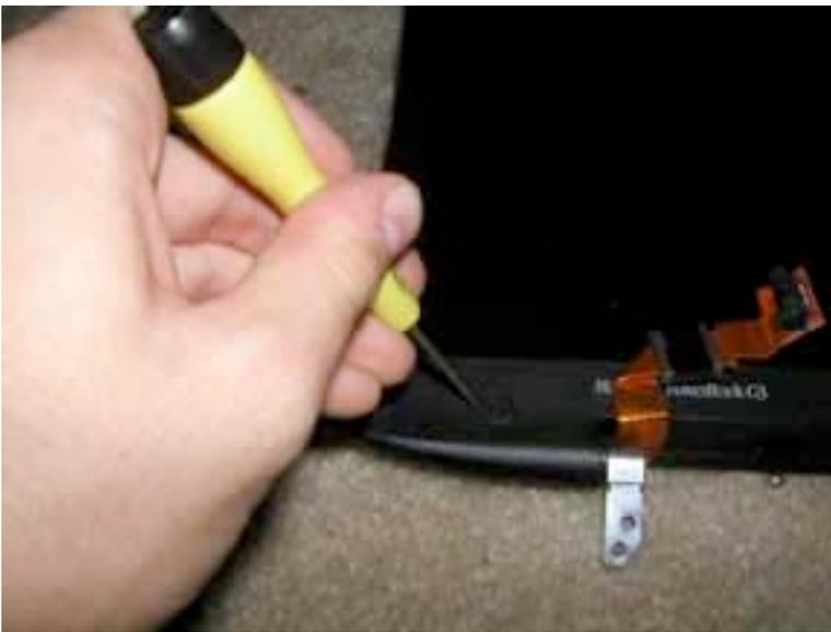
Using a flat head tool, pry up the flat plastic covering on the bottom of the display on either side of the cables. The left side is shown in the picture.
