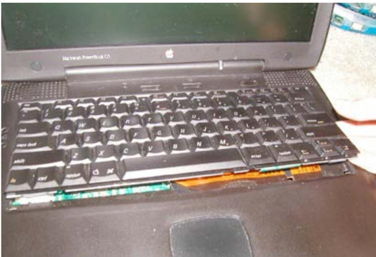
Lift the keyboard up and pull towards you to free the metal locks on the top of the keyboard. Then flip the keyboard out towards you.
