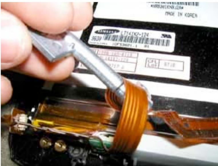
The inverter cable is wound around the hinge. You will need to unwind it from the hinge to remove it. When you replace the hinge or display cable, make your to wind it back around the hinge.
