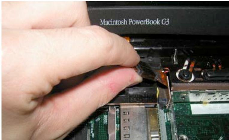
Grasp the orange display cable on the left of the laptop as shown. Gently pull up to undo it from the motherboard.
