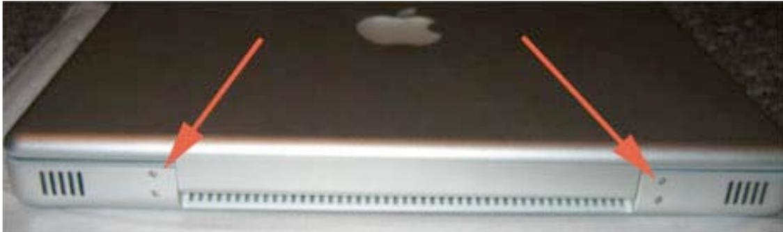
Now, go to the right hand side of the unit (with the optical drive slot) and remove the two 5.5mm silver screws in the location shown.
