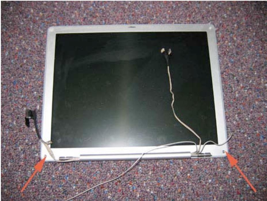
Use your flat tool to separate the front bezel from the back case. The back case includes the light grey plastic trim, so insert your tool on top of the trim between it and the front bezel as shown in the picture below. The hardest part will be separating the first corner.
