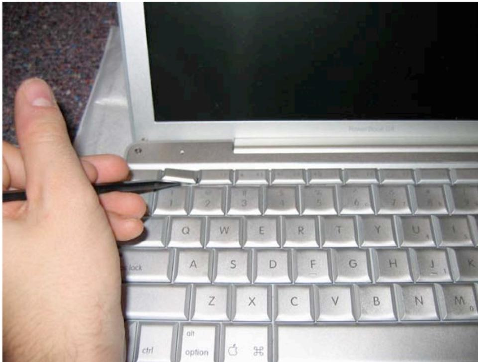
Next, remove the white round stickers located between the keys. These round stickers cover two screws that need to be removed. After the stickers are removed, remove the two Philips head screws.
