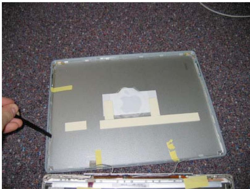
The end of each cable has a metal portion that is held in place by two clips. Use your flat tool to gently pry the clip free of the two receptors.
