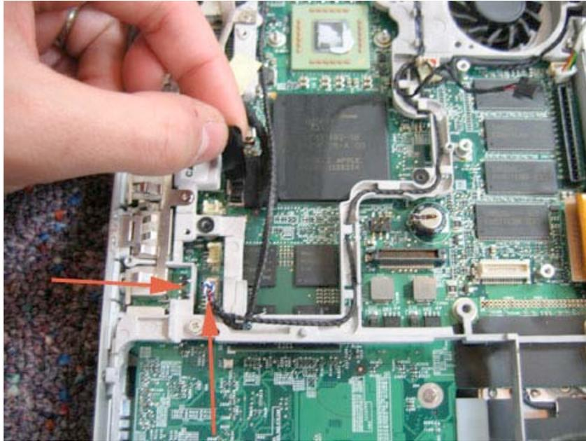
Near the fan (usually tucked away in the corner with the fan logic board connector) is the speaker wire connection joint as is shown in the picture below. Disconnect the two cables by pulling them in opposite directions.
