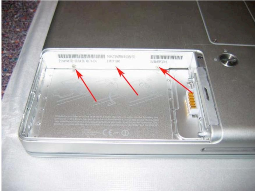
Flip the unit back over, and remove the 11 screws in the locations shown in the picture below. Also note the sizes of the screws for reassembly purposes.
