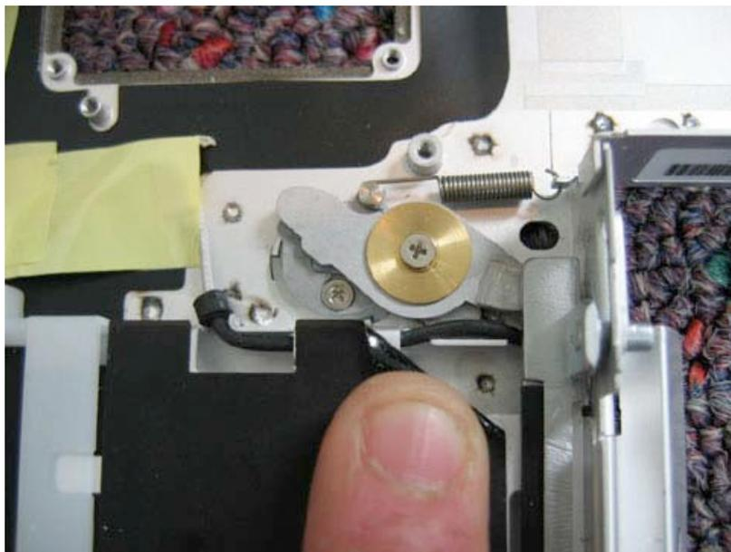
Next, use your flat tool to lift the cable up and over the metal divider, pulling towards you so that the cable ends up in the airport extreme slot. Next, pull the cable through the slot on the left hand side of the slot (not through the opening the card goes in.) This will free the airport cable.
