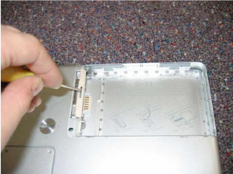
There is a plastic tab that is usually folded on the top of the card. You can use your flat tool to pull the flap towards you as shown in the picture below.
