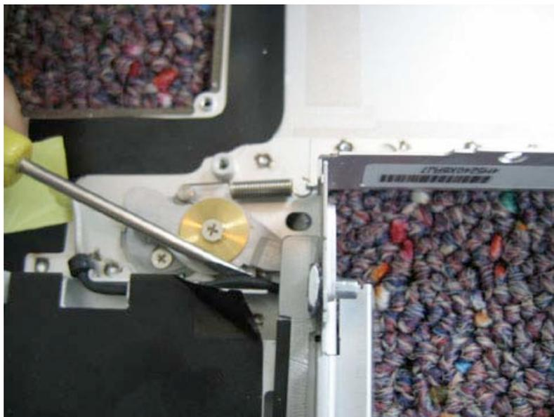
You will now be able to lift the display module up and out of the unit. If it does not come out easily, adjusting the angle of the display will help it to come free.
