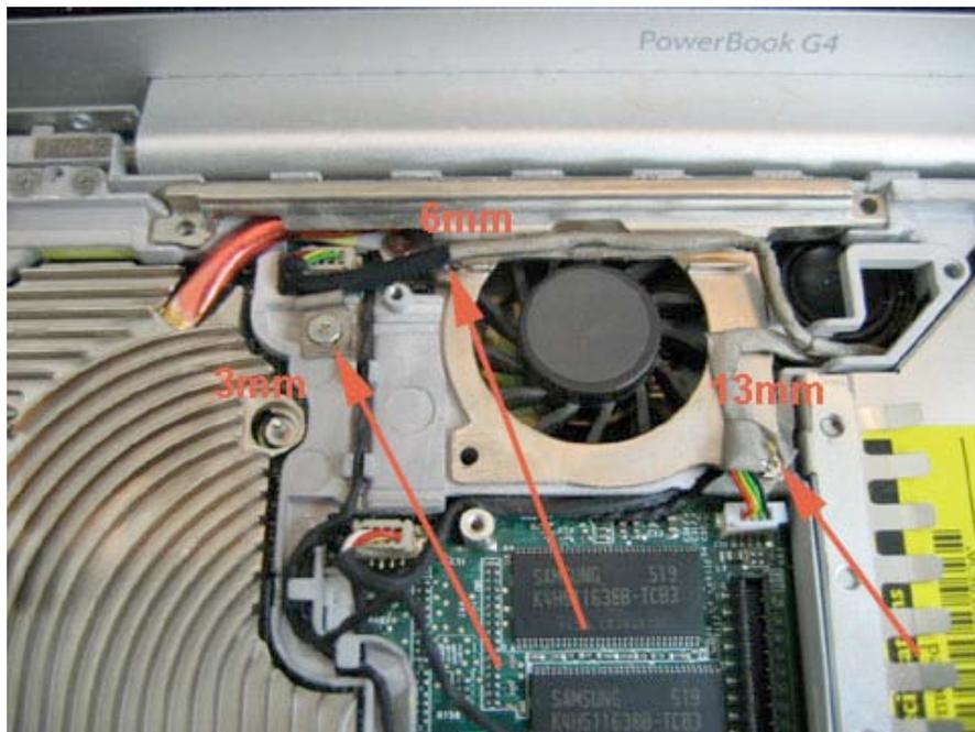
Next, following the same procedure as with every other logic board connector, disconnect the inverter cable from the logic board. Again, be very careful not to damage the connector.
