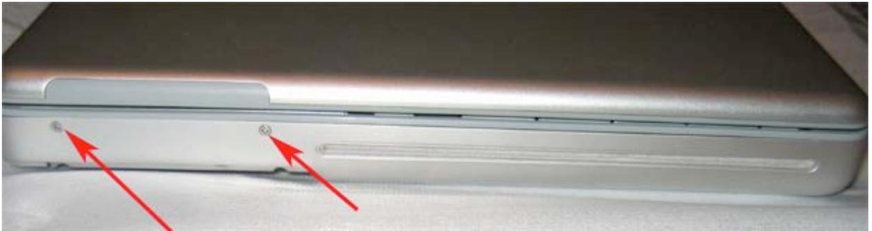
Now, go to the left hand side (with all the ports) and remove the two 3mm silver screws in the location shown.
