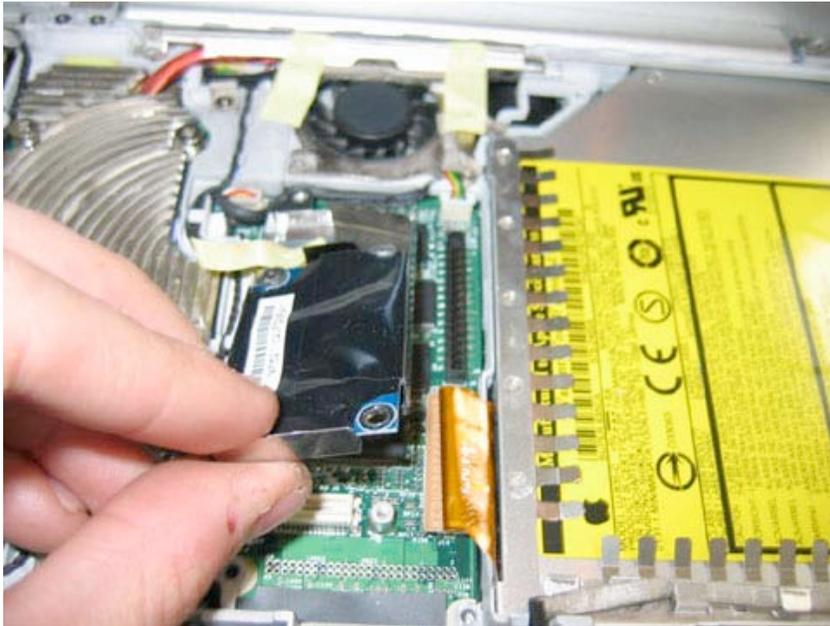
With the modem free, grasp the modem cable going into the modem and gently pull it out (away from the modem.) It should come out easily, and the modem will be free to set aside.
