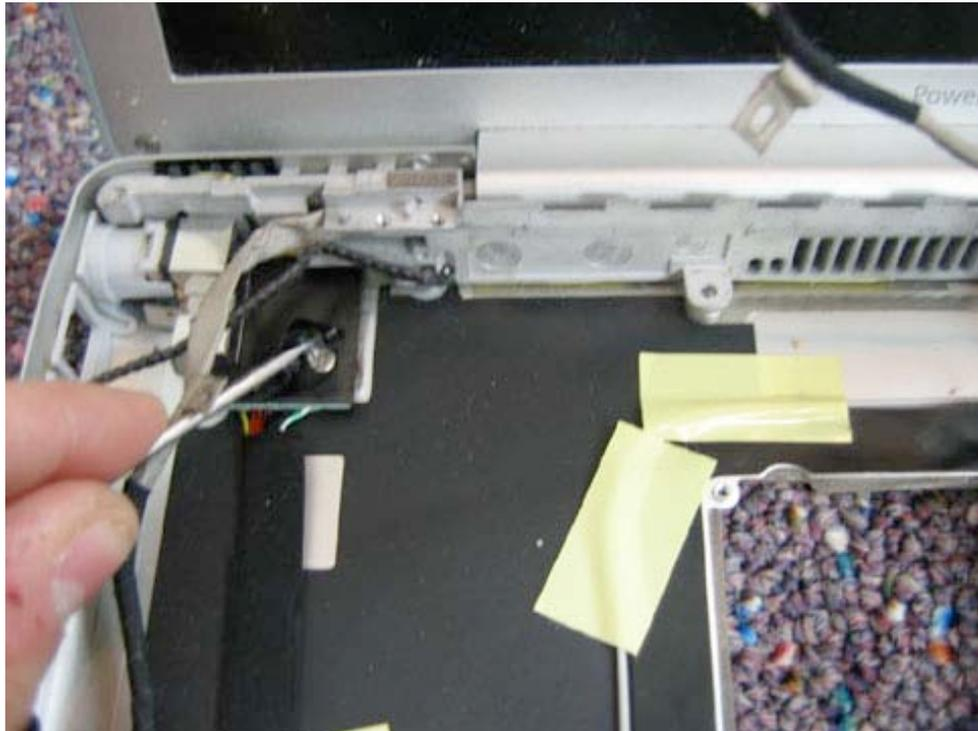
This will reveal a Philips head screw. Remove this screw.
