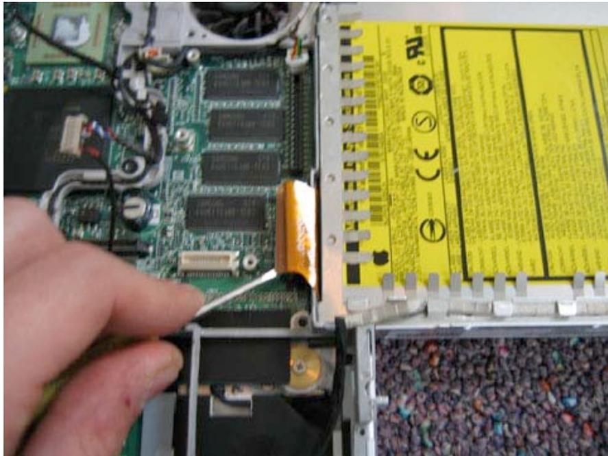
Use your finger to push the cable towards the optical drive (away from the rib frame) as shown in the picture below.
