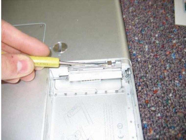
Now you need to undo the airport connector from the airport extreme card. This is most easily accomplished by grasping the connector with pliers and pulling out gently. Use only a little force, and be careful not to damage the connector or card.
