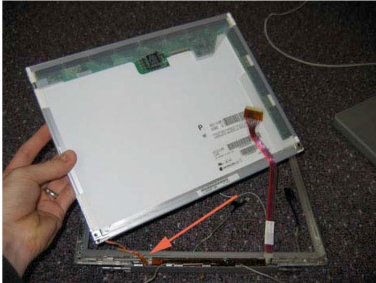
The inverter cable connects to the inverter board as shown. To disconnect the cable, grasp the board in one hand (you may have to slightly pry up the board using your pry tool) and the cable in the other, and pull the two apart. The cable may take a little force to come loose. The LCD will now be free to be removed.
