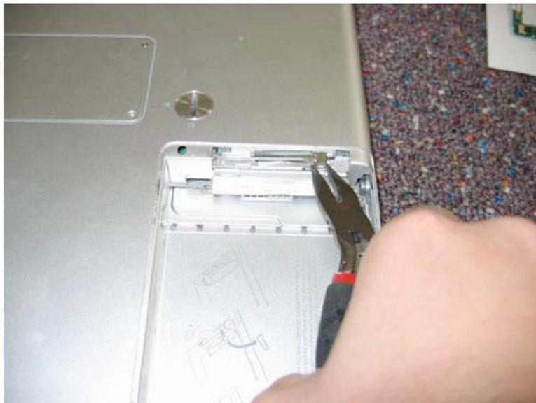
Next, using the plastic tab, gently pull the card towards you until it is completely free of the unit.
