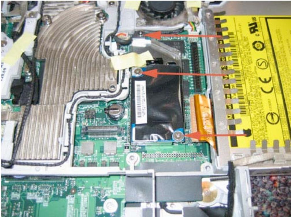
Next, lift the modem up from the front edge as shown. It should lift up easily. If it does not, use your flat tool to gently pry it up. The DVI model has a modem shield located under the modem (the silver tray) This piece should lift up with the modem. The VGA model does not have this tray. If there is any tape around the modem or cable coming out of the modem, remove it.
