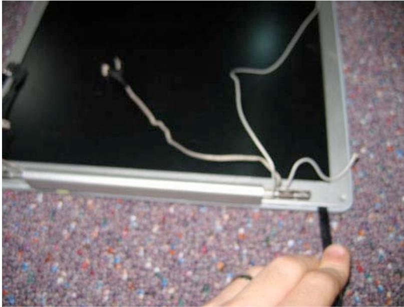
With the first corner separated, work your way around the entire display casing. The case should get progressively looser and easier to manage.
