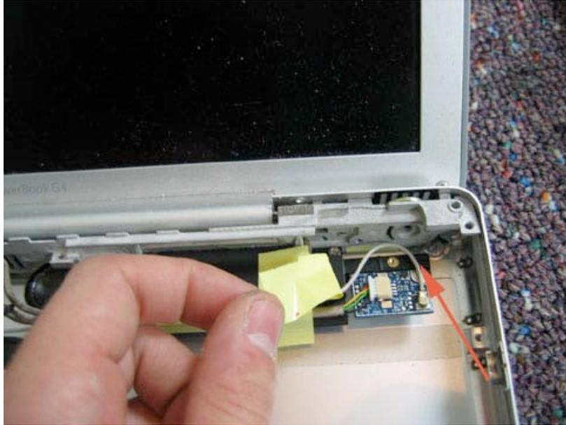
The multi color cable going into the Bluetooth board is the Bluetooth cable. Undo this cable by grasping the cable and pulling it gently to the left. The grey cable with the gold end is the Bluetooth antenna. Disconnect this cable by grasping the gold receptor and gently pulling up. To reattach, align the connector and push down until it is “snaps” into place.
