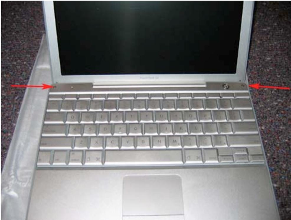
Next, shut the lid of the computer, and turn it around to the back. Remove the two Philips head 5.5mm silver screws as shown. (Note: If you only need to remove the trackpad, it is only necessary to remove the top screw on each side. The bottom screws anchor the display module.)
