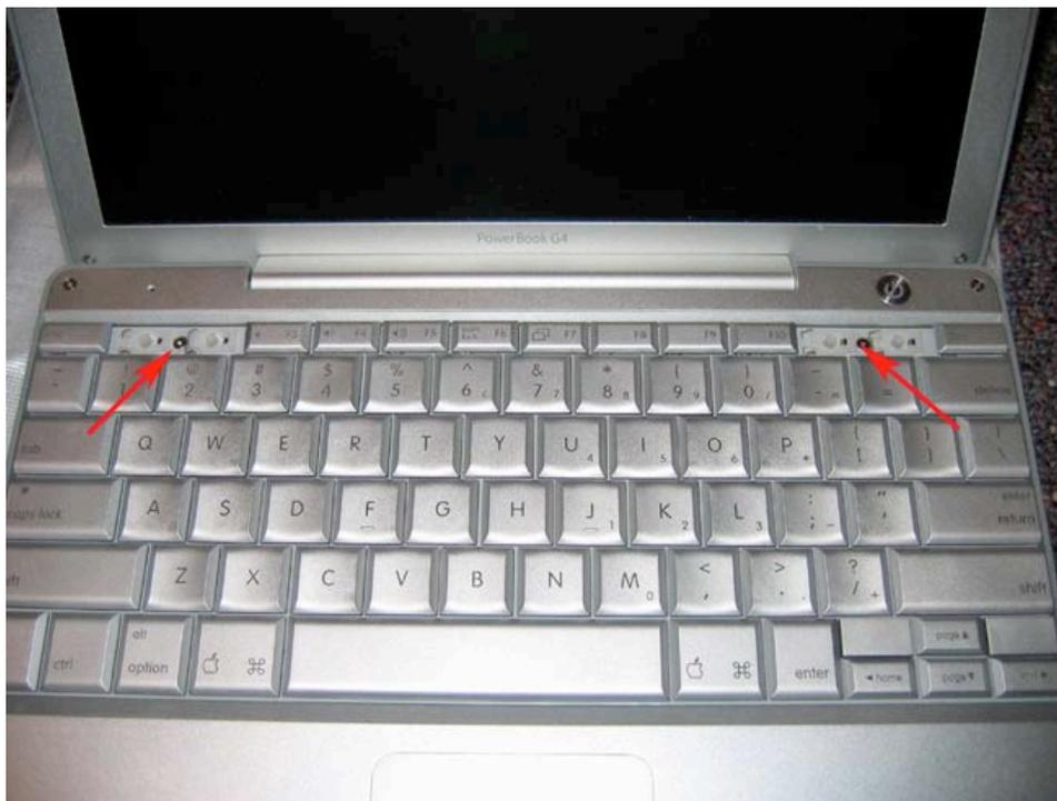
With the screws between the keys removed, Use a flat tool to pry up the keyboard (preferably from the back left or right hand corner as shown.)
