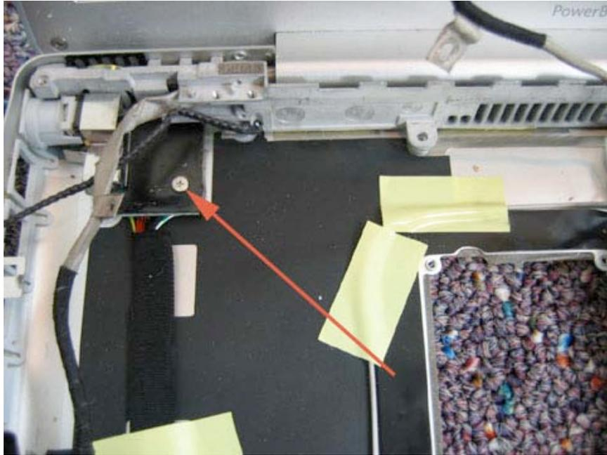
Grasp the DC-In board as shown and pull towards the optical drive. You may have to move the display to a different angle to let the cable come out easily. Note that there is a light grey cylindrical piece on the end of the DC-In Board. This may or may not stay in place on the case. If it does not, to reassemble, place this piece on the end of the DC-In board with the long tab on that part facing you.
