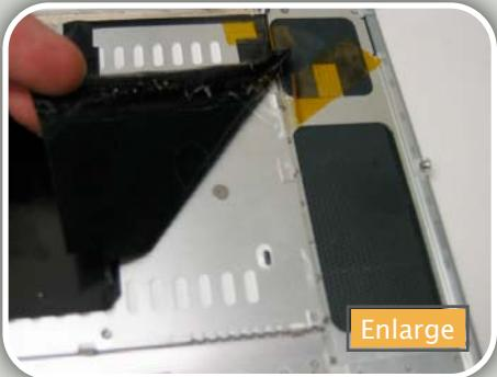
ing the backing from one of the corners. It is best to take it slow unless your new keyboard including a new backing. Just continue to slowly peel it towards the center. It is made up of two separate pieces. If your new keyboard doesn't contain a new package, place these two old pieces to the side with sticky side up. Take note of which side of the backing goes where, but it will later be explained how to match up the correct sides just in case you mixed them up.
