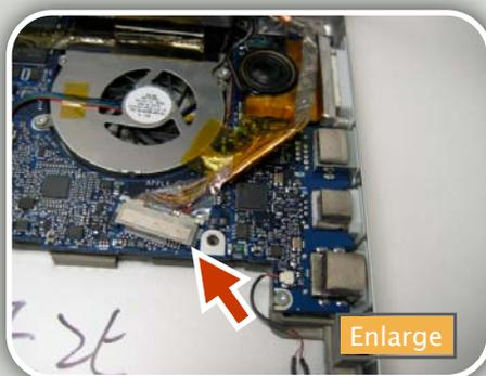
end. This cable controls the picture on the screen. It can just be pulled out of the connector.
