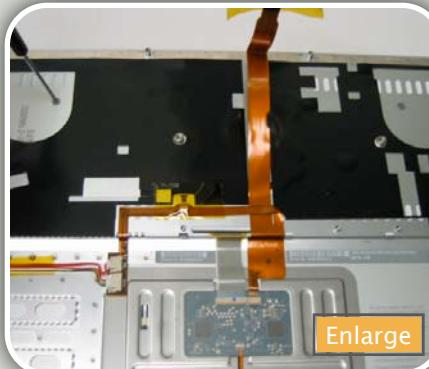
found in Apple products. The cable is locked in place by a small bar that needs to be flipped upright into the unlocked position. Be very gentle as breaking this could require a new top case. Once the bar is flipped up, you should be
