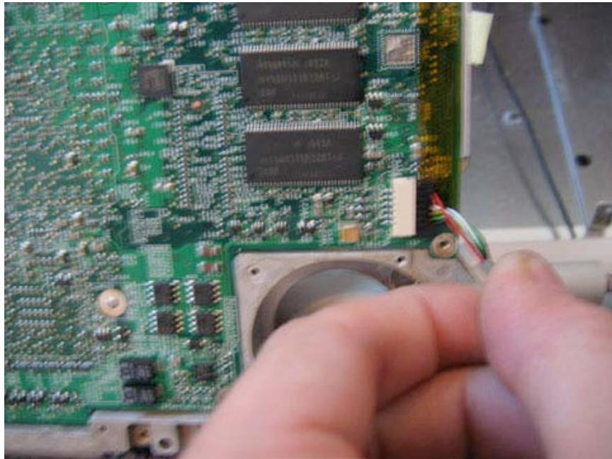
Remove the four Philips head screws from the locations shown. Note that the middle two screws hold on the vent cover that can be lifted out once the display module is removed.
