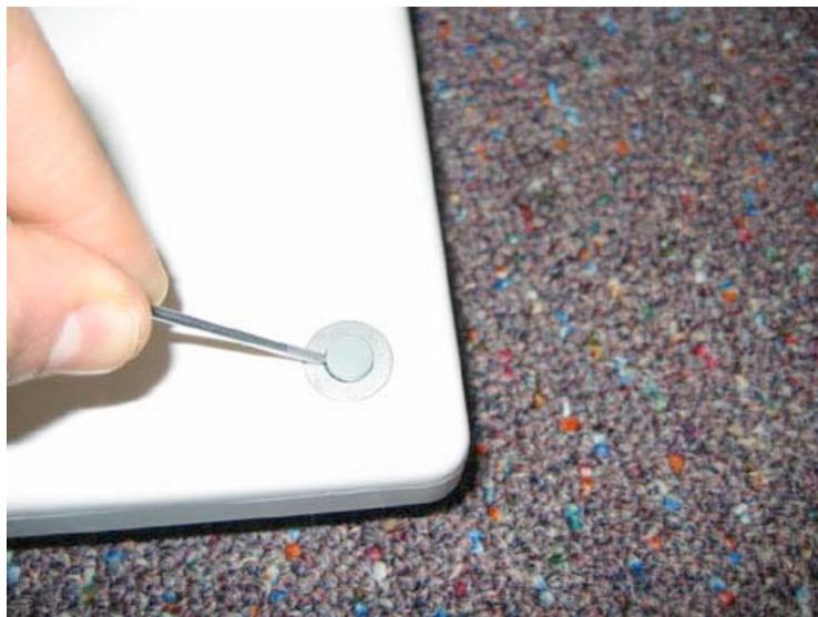
Unscrew the Philips head screw underneath the three feet, and lift out the metal foot socket as shown.
