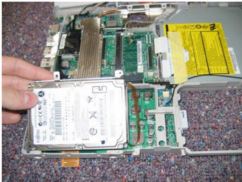
Pull the bracket off of the side of the drive as shown. It should come off easily.
