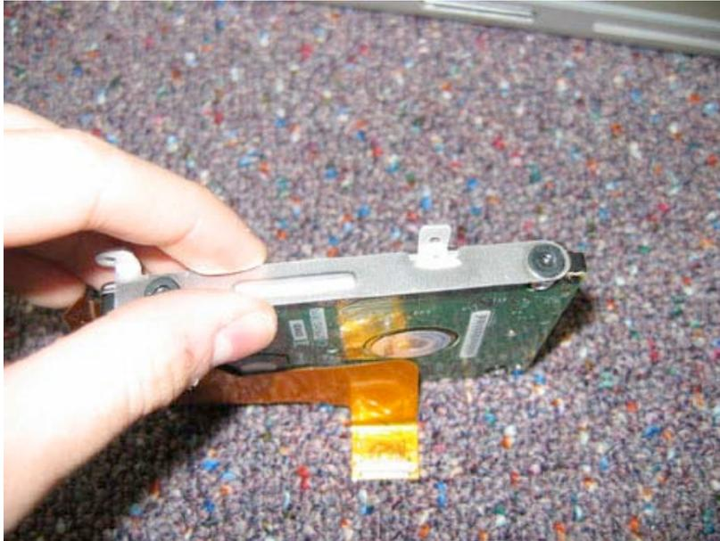
Disconnect the hard drive cable by gently pulling the cable away from the hard drive using the orange pulling cable as shown in the picture below. The cable should come free easily.
