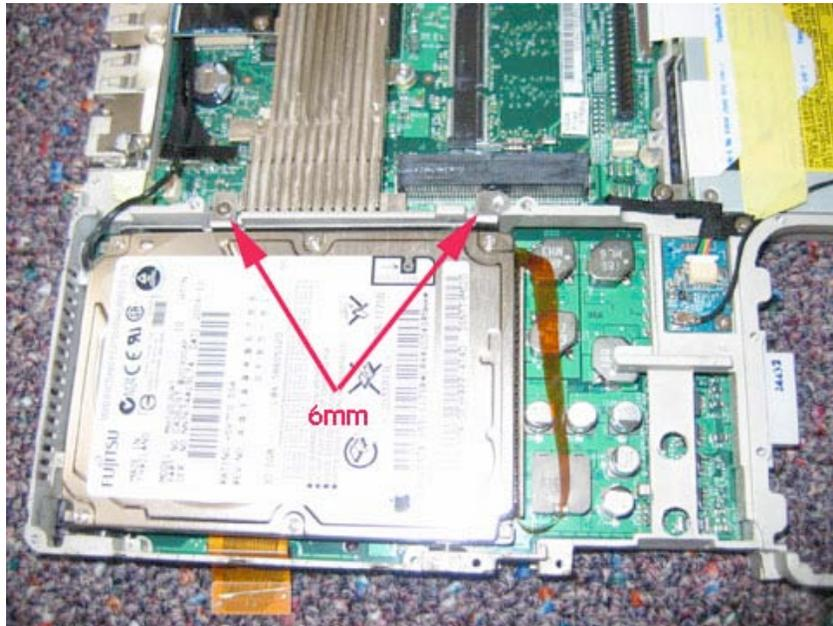
Lift the hard drive up and out of the unit as shown.
