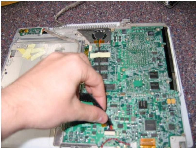
Grasp the Dc-in board as shown, and lift it up and out of the unit. It should come free easily.
