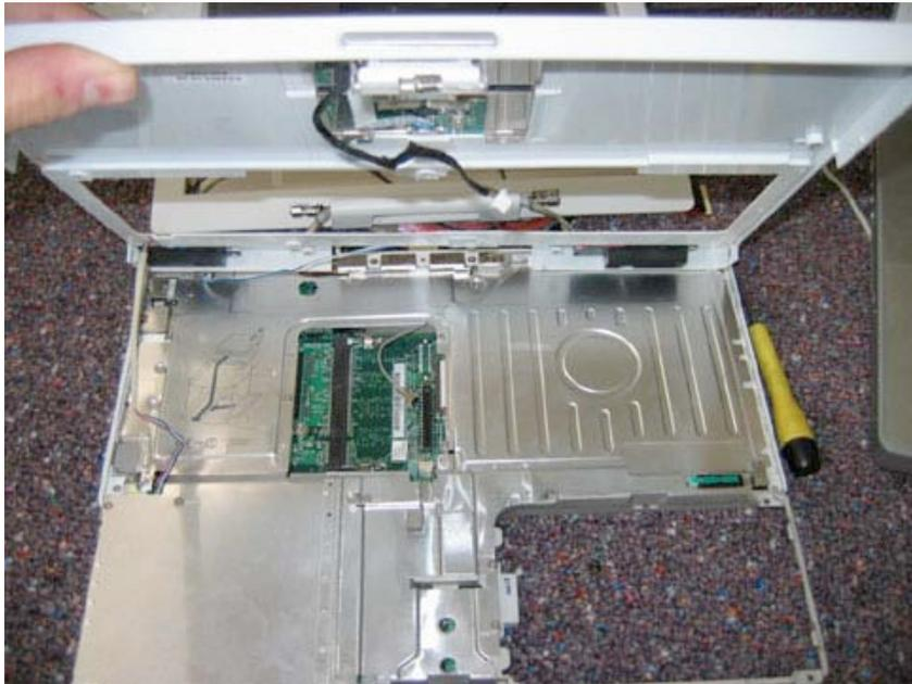
There are two cables attached from the top case to the logic board. You should be able to gently wiggle these free from their logic board connections. If they do not come out easily, then use a flat tool to gently pry up while pulling. \*Be careful! If you use too much force and the cable does not come easily, you could damage the connector to the logic board! Once the connections are undone, the top case will be free to be removed.
