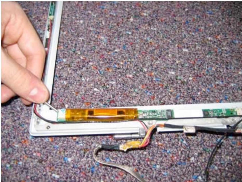
Lift the inverter board up and out.
