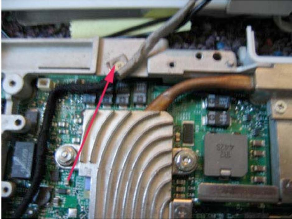
Next, disconnect the microphone cable by gently pulling up as shown. Remove any tape that may be holding the cable in place.
