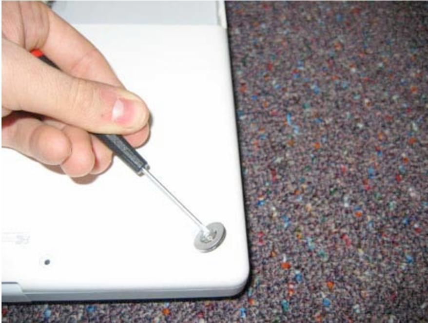
Inside the battery bay are two more Philips head screws in the locations shown. Remove these two screws.
