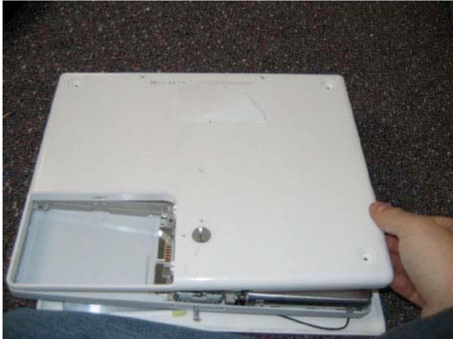
Notice that in the battery bay there are two springs with white rubber stoppers. You should remove these by simply lifting them up. Make sure to reinstall them during reassembly.
