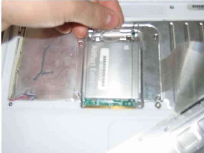
Locate the plastic tab on the airport card, and gently pull away from you to disengage it from its connector. Undo the airport connector from the card, and set the card aside on a static free surface. Note – To remove the airport connector from the Airport extreme card, use your fingers to pull it out. If it does not come out easily, use a pair of needle nose pliers to gently pull it out. Do not use too much force or you may damage the connector.
