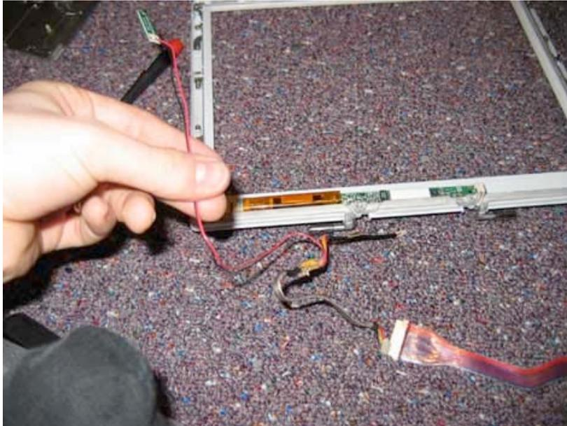
Next, remove the tape holding the inverter cable microphone cable together. It may take several attempts to get the tape off. Separate the cables. When replacing, it is not necessary to tape the cables back together, but you can do so if you have some yellow tape.
