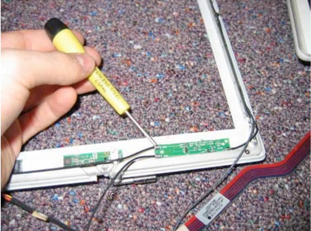
Remove the two Philips head screws in the locations shown below.
