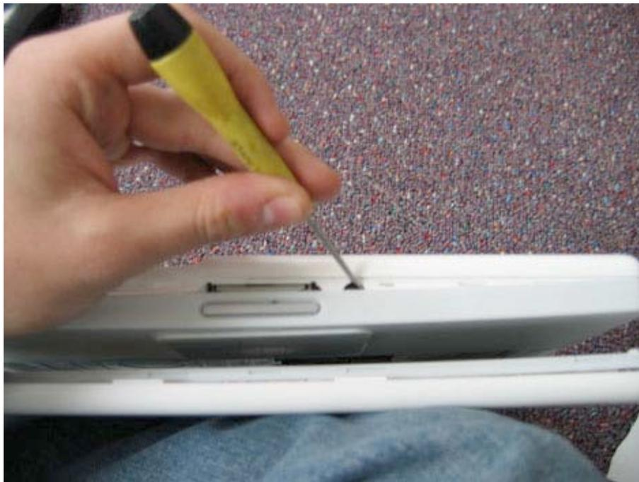
Disengage all of the latches all the way to the optical drive. The right hand casing should be free to lift up and to the left. Lift the bottom case up as shown to disengage the latches on the optical drive. The bottom case should come off easily.
