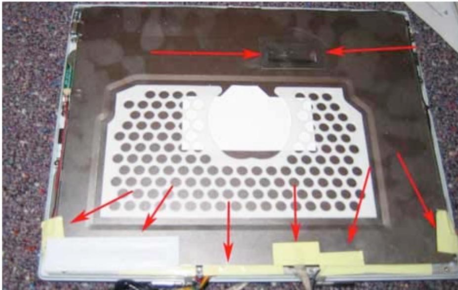
You can now lift up the back shield. Lift it completely off and place on a clean surface.
