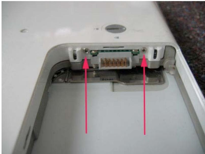
Beginning in the battery bay corner, Use your fingers to separate the corner plastics, and then undo the latch in the battery bay by using your flat tool to pry the latch out while lifting up.
