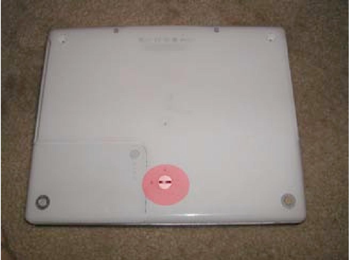
Using either a flat head screwdriver or a coin (anything with a flat surface) turn the security latch to the left as shown. Turn it until the notch is facing the “unlock graphic.”
