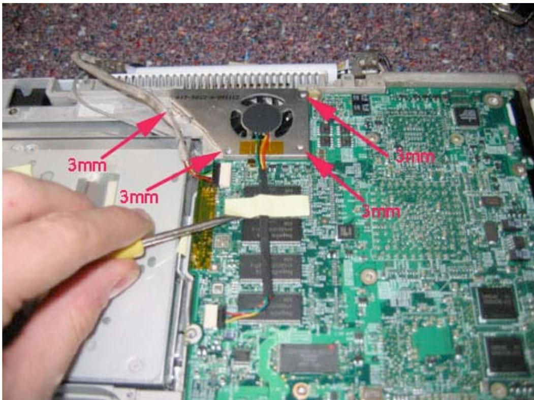
Disconnect the fan cable from the logic board, and lift the fan up and out as shown.
