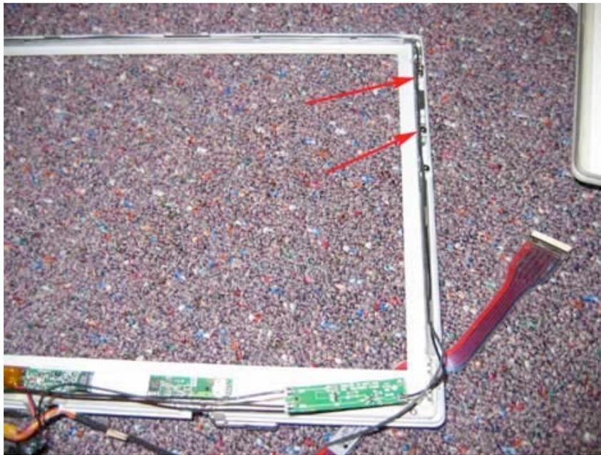
With the screws removed, tilt the metal piece with cable attached up and out towards you. Note that there is a cable that keeps going past this piece. That is the microphone cable and is not a part of the airport cable assembly.
