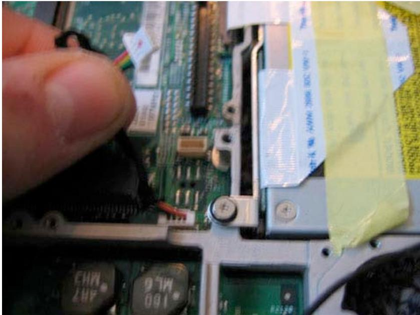
To remove the antenna, grasp the cable as shown, and pull to the left. It should easily slide out of the antenna holder.
