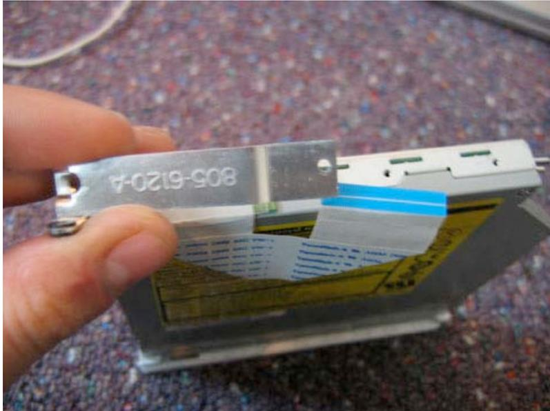
Use your flat tool to gently pry up on the optical drive cable connector as shown. It should come free with little force
