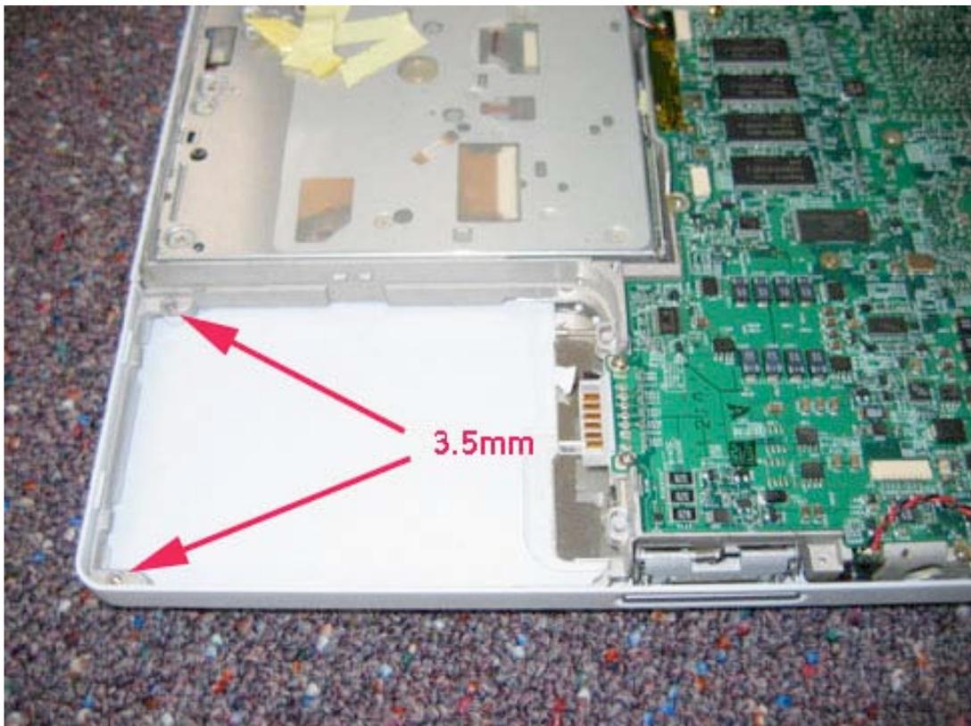
Remove the seven Philips head screws from the locations shown. Note that the 4.5mm screw is located under a magnet. Use your flat tool to pry the magnet up to reveal this screw. Do not forget to install this magnet during reassembly.
