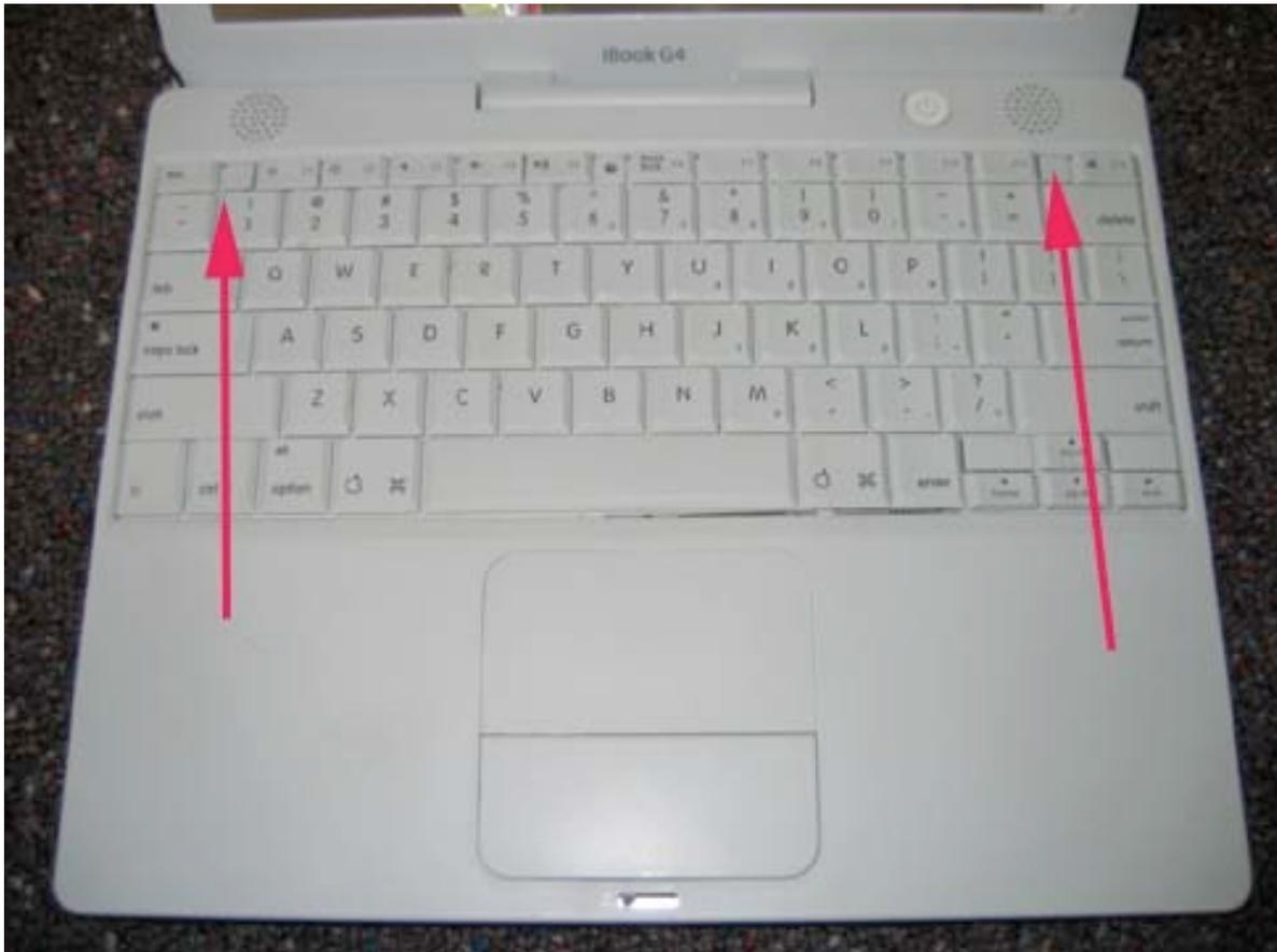
While depressing the tabs, pull the keyboard up, out, and flip it towards you as shown.
