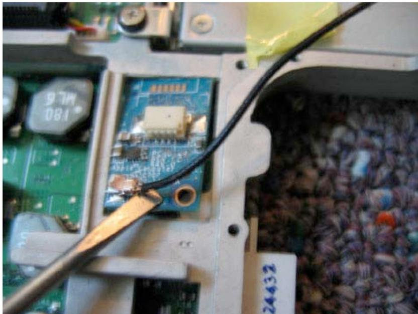
Grasp the Bluetooth cable, and gently pull it free from its logic board connector. The cable will now be free.
