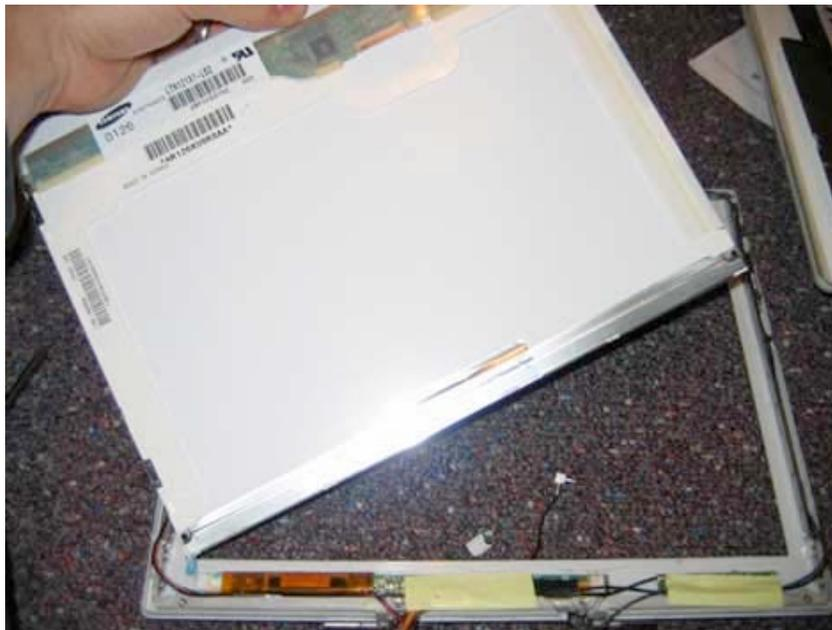
Pivot the LCD all the way to the left as shown, and disconnect the inverter cable connector from the Inverter board at the location shown.
