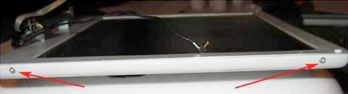
Next, you will need to pry the back panel (case with Apple logo) off. It is best to start at a corner as shown, and pull the casing in the opposite direction as the LCD. You may need to use a flat too to help you at first. After you get started, the casing will come off easily.
