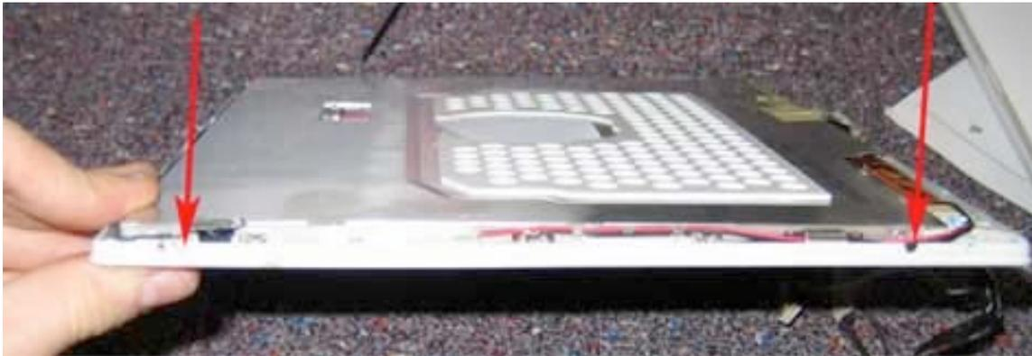
Remove all the pieces of tape holding the thin metal sheet in place. The location of the tape can vary from model to model, so use the picture below as a guide. Make sure to remove the Aluminum tape in the middle of the cover as well.
