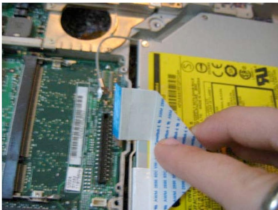
You can now lift the drive up and out of the unit as shown.
