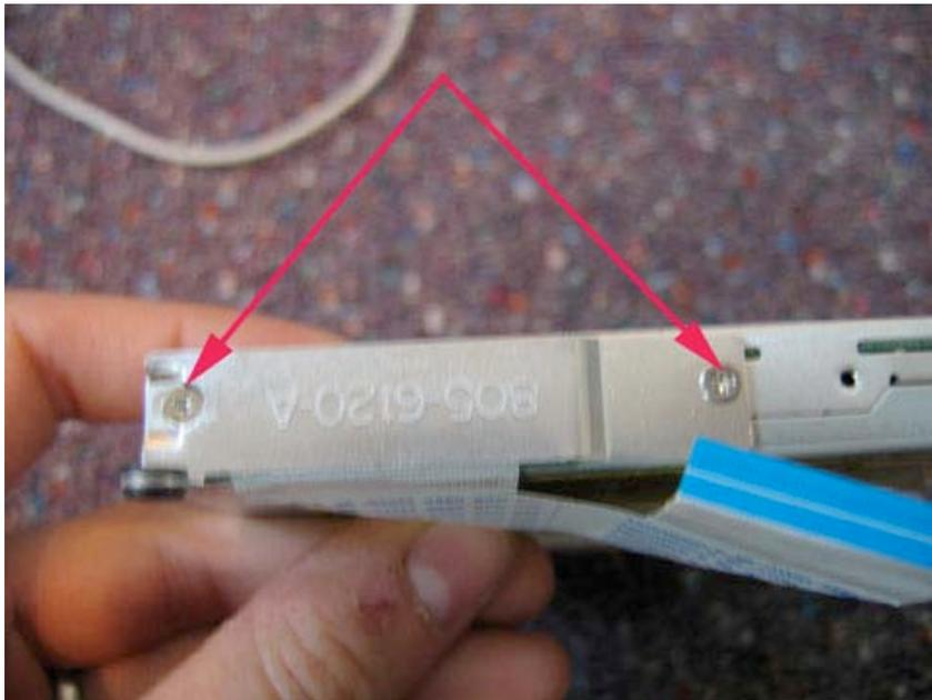
This will release the back bracket. Remove it as shown.
