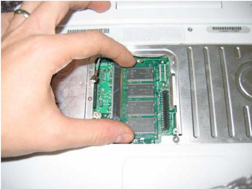
To install, simply line up the chip with the ram slot and push the chip down so it engages the ram clips
