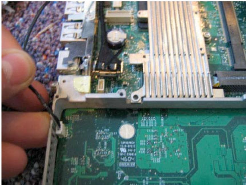
From the bottom of the unit, disconnect the inverter cable from the logic board, by gently grasping the cable as shown and pulling away from the connector.
