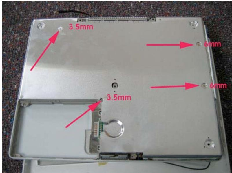
Next, simply lift the bottom shield up and away from the unit. It should come free easily.
