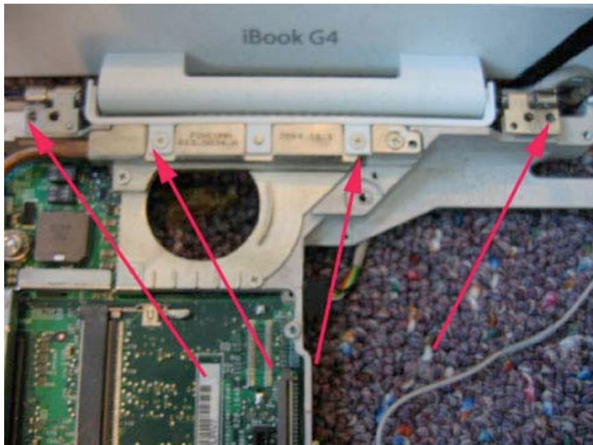
Lift the display module up and out as shown. Make sure all cables are routed properly and come out easily.
