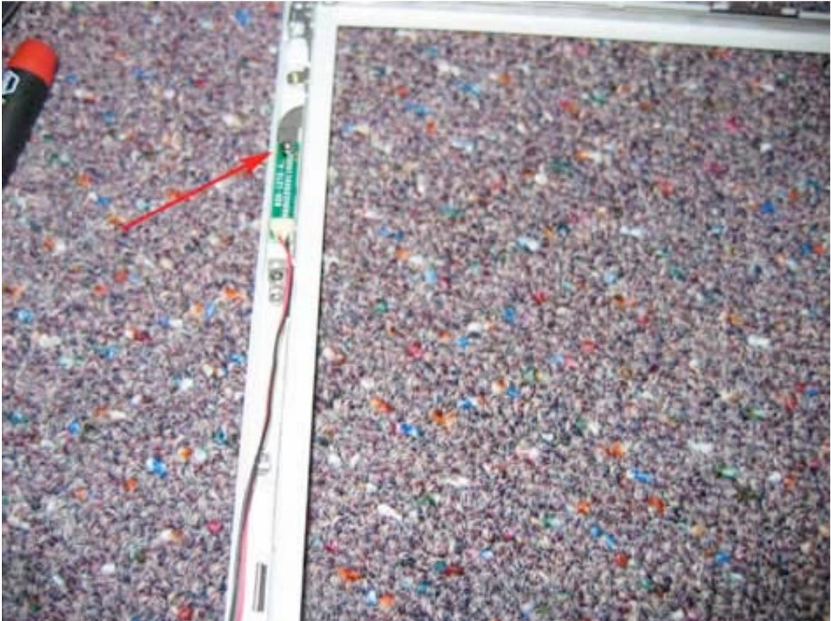
Guide the reed switch cables out, and if held in place by any tape, remove the tape.
