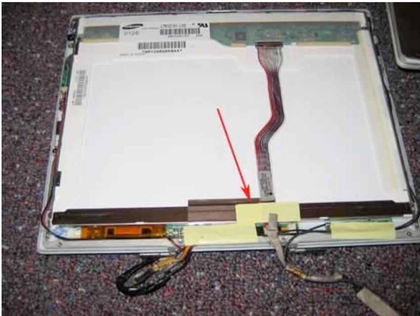
Disconnect the display cable from the LCD by gently grabbing it as shown and then pulling it towards you. It should come out very easily.
