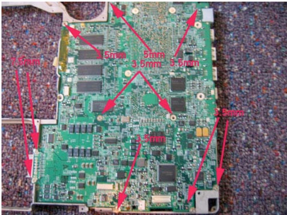
Lift the board up and out as shown.
