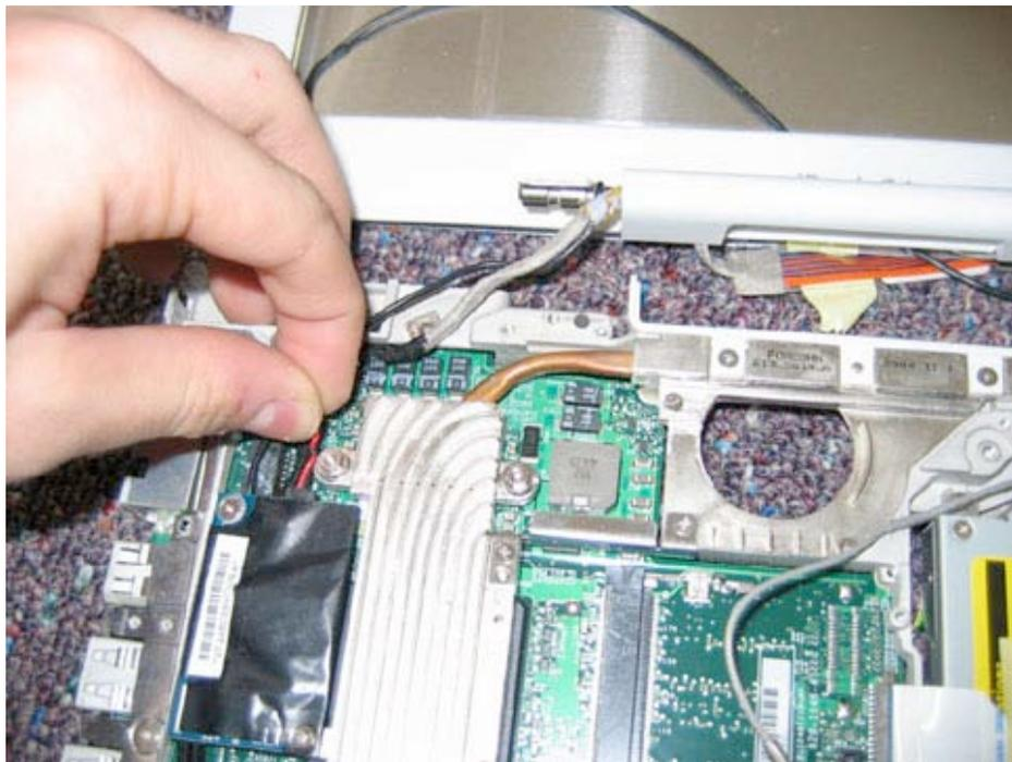
Using your finger, push the modem port away from the unit. You may have to use a minimum amount of force to guide it off the logic board. The port will now be free.
