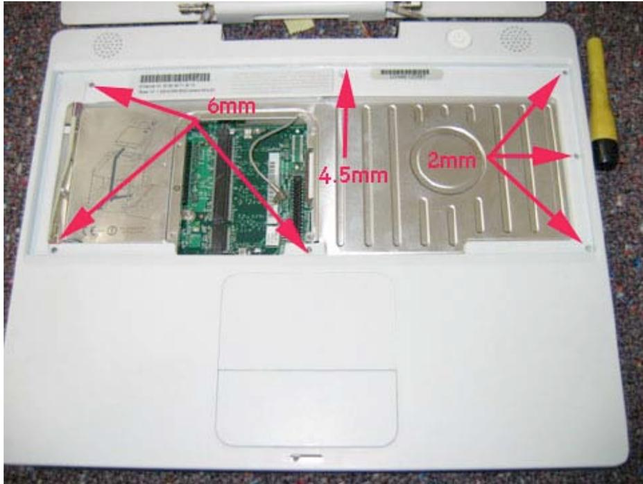
Starting at the battery bay gently pry the top case away from the frame of the computer.
