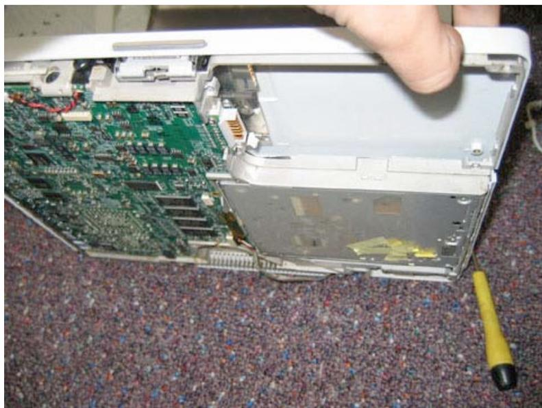
Make your way around the top case until you can easily flip it up as shown (with cables still attached!)
