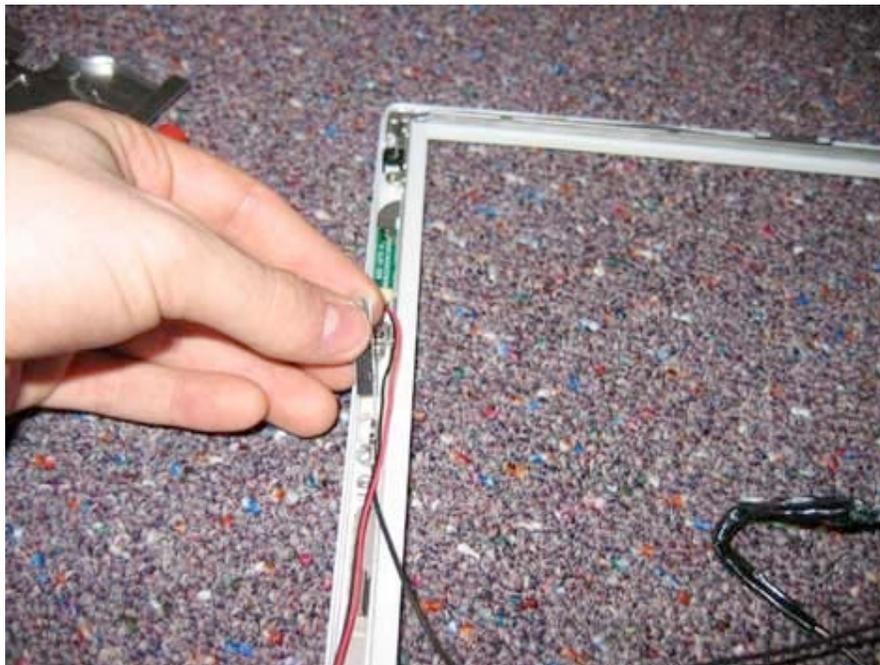
The cable assembly should now be loose. If it is not, make sure you have removed any tape that may be holding the cable in, and make sure the cable has been guided out of all of the metal clips that hold the cable in along the side of the display. (Just pull up on the cable to release it from the clips)
