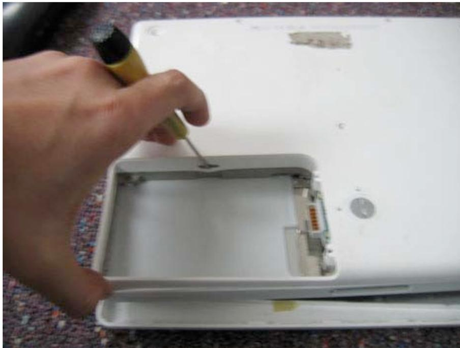
Work your way around the front edge of the casing with a flat head screwdriver or pry tool while pulling up on the case to disengage the latches around the unit.
