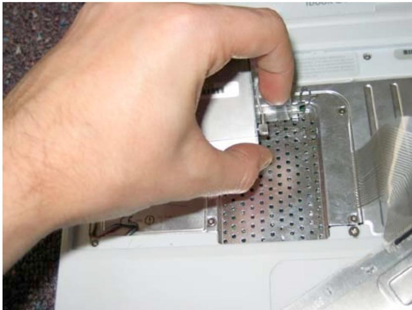
Remove the four screws from the airport retainer in the locations shown, and lift the airport retainer up and out of the unit.
