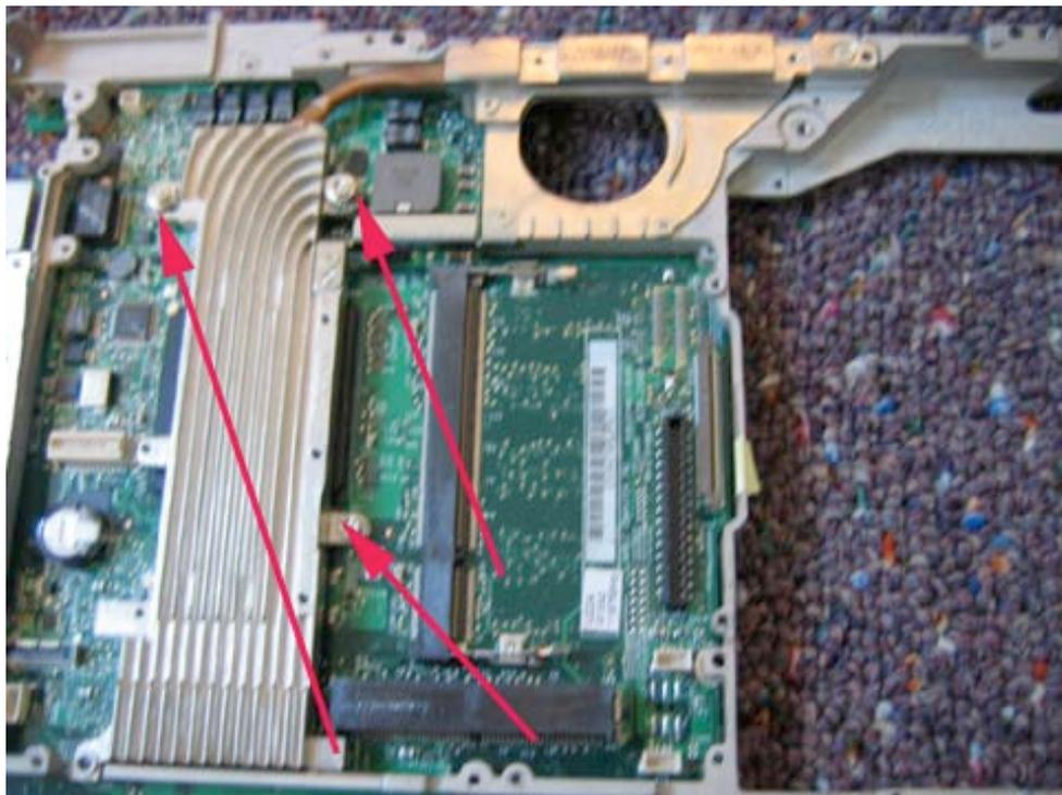
Lift the heatsink up and out of the unit as shown.
