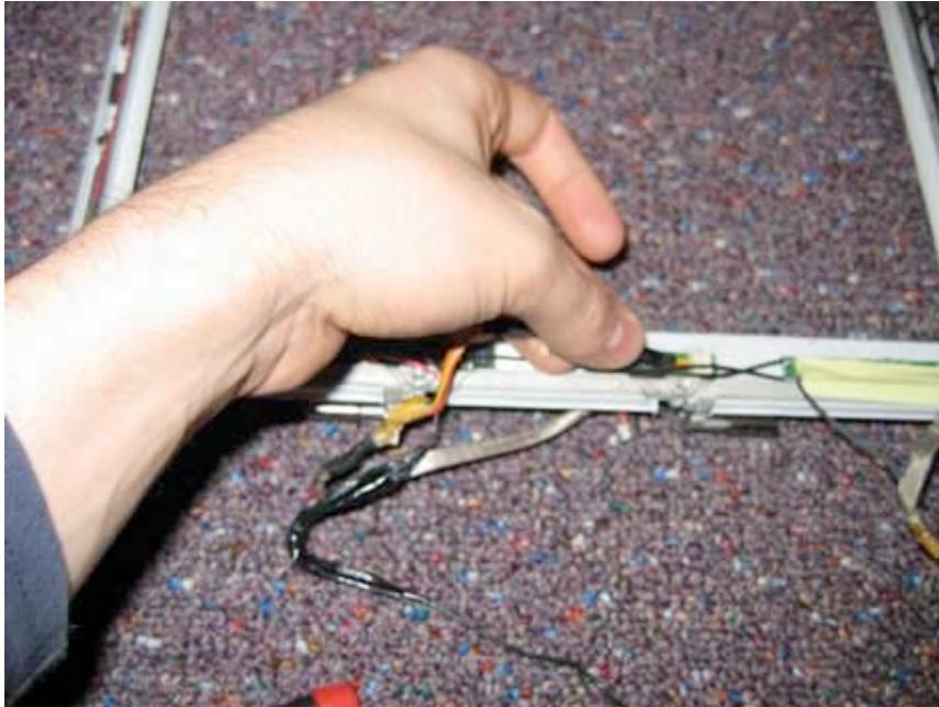
The inverter board is held in place by adhesive tape. You will need to use a flat tool to pry up the board. It is best to do this from the left hand side of the board. Put a flat tool under the board, and gently pry up.
