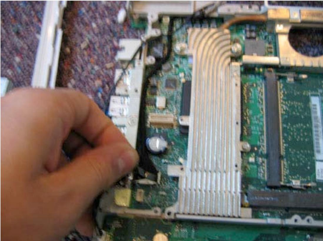
Remove the screw holding down the LVDS cable in the location shown.
