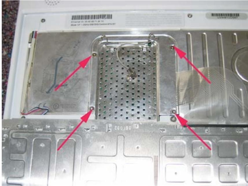
To remove the keyboard, gently lift up on the cable as shown. The connector should easily come free. Set the keyboard aside.
