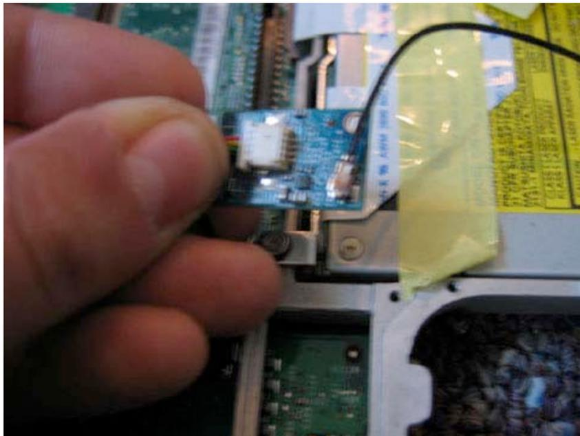
Use your flat tool to gently pry the Bluetooth antenna connector from the Bluetooth board. It should come off easily. If it does not, try it from a different angle. The Bluetooth board will now be free.
