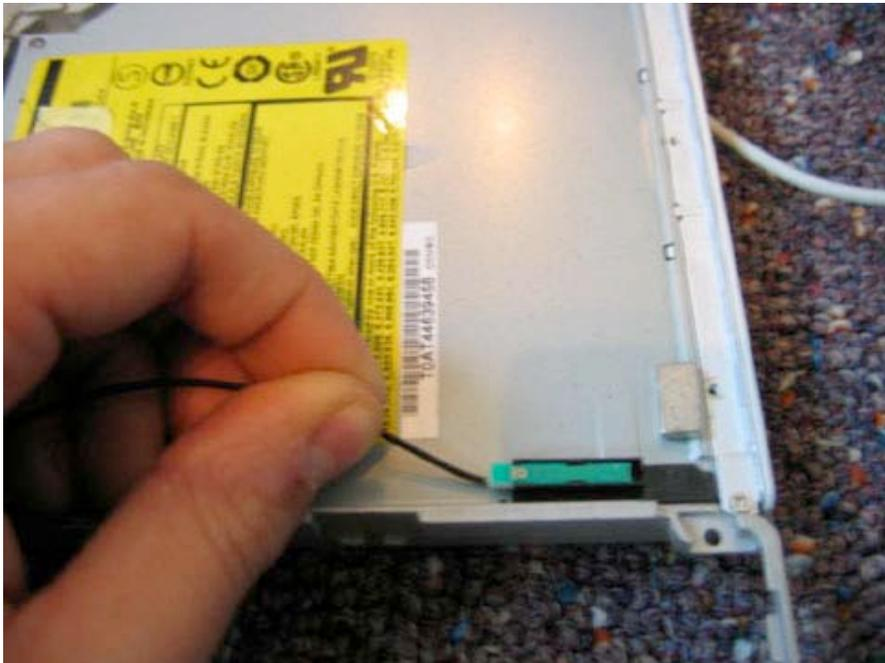
The antenna holder is held in place by a very light adhesive. Use your flat tool to pry the holder off of the optical drive. It should come off easily.
