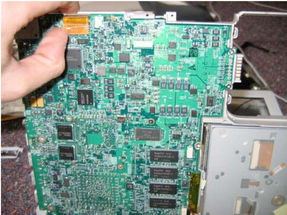
Flip the unit back over and remove the two 6mm Philips head screws from the locations shown in the picture below.
