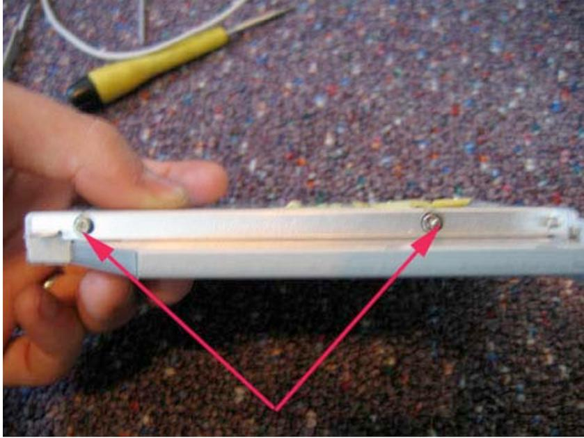
Remove the one Philips head screw on the front of the drive. The bracket should fall off.
