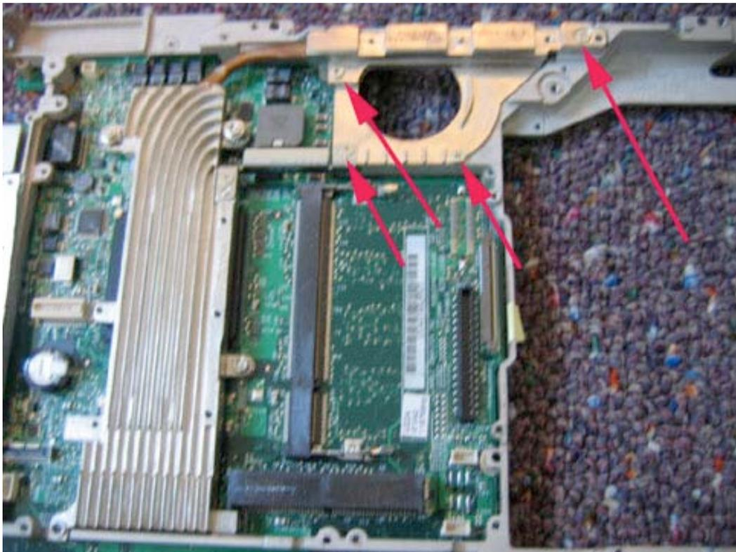
Remove the 3 hex nut screws from the locations shown. Use either pliers or a hex nut screwdriver to remove the screws.
