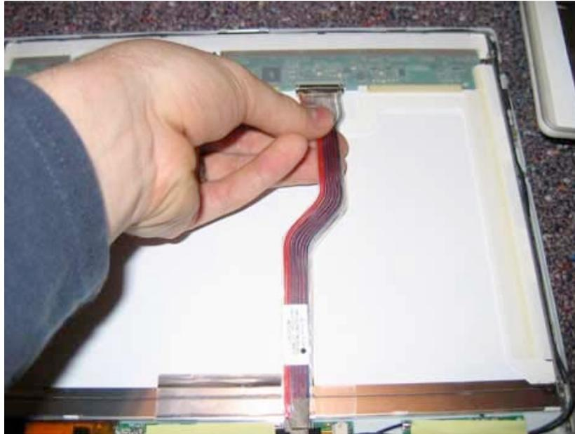
The LCD panel will not be free to be moved. Lift up the display, and pivot it towards the left hand side where the inverter cable enters the LCD.
