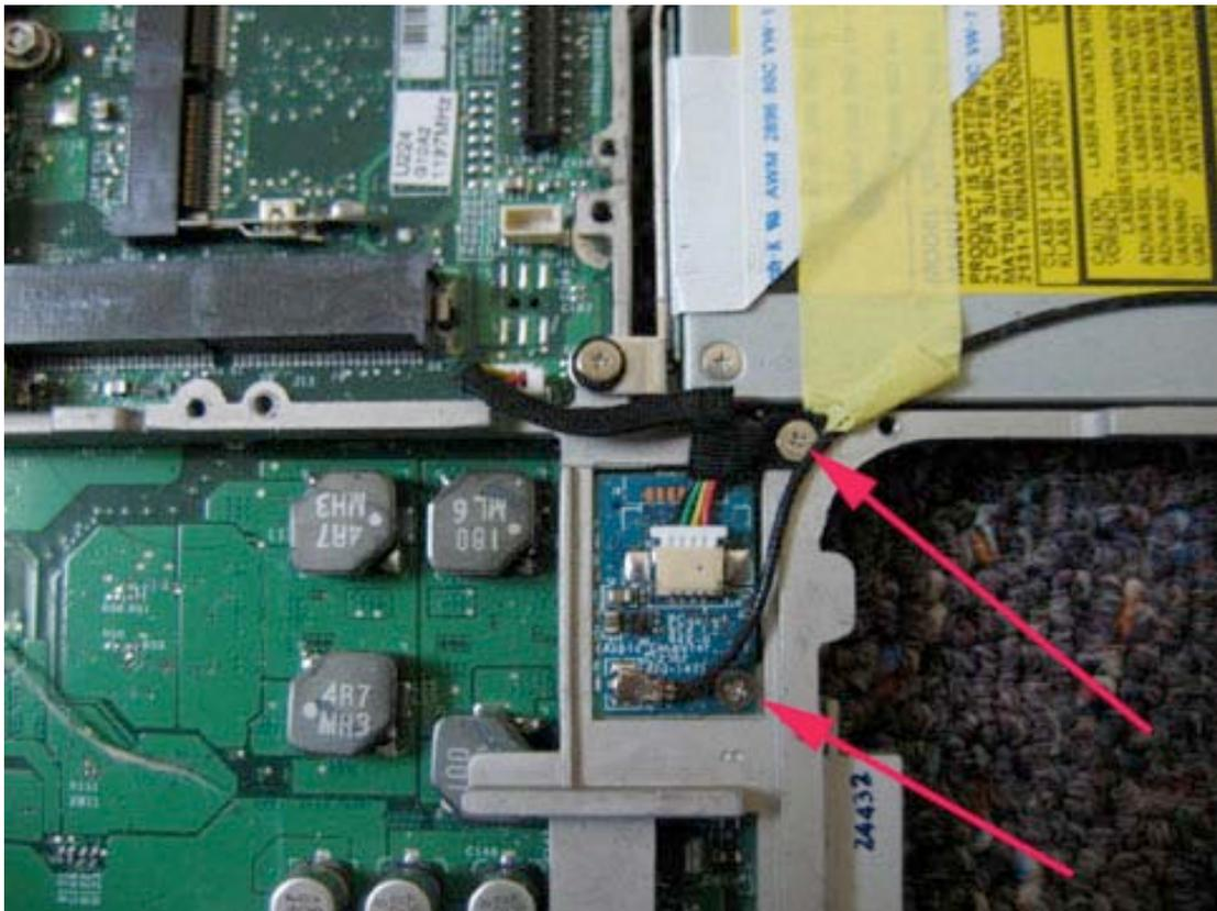
Grasp the Bluetooth cable as shown and gently pull it free from its Bluetooth board connector. It should come out easily. If it does not, Use your flat tool to aid.
