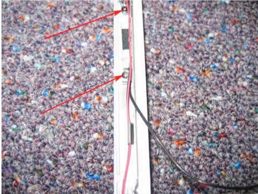
With the screws removed, tilt the metal piece with cable attached up and out towards you.
