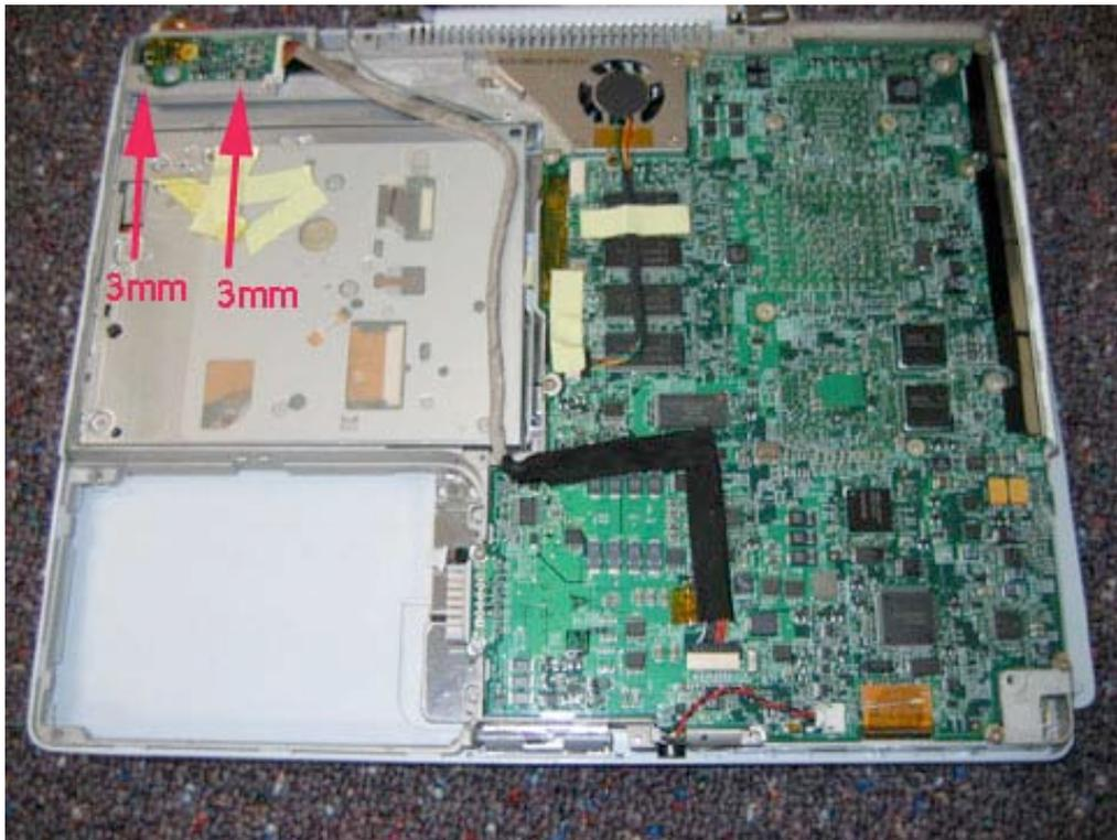
Disconnect the DC-In board connector from the logic board by gently grasping the cable and pulling away from logic board connector,
