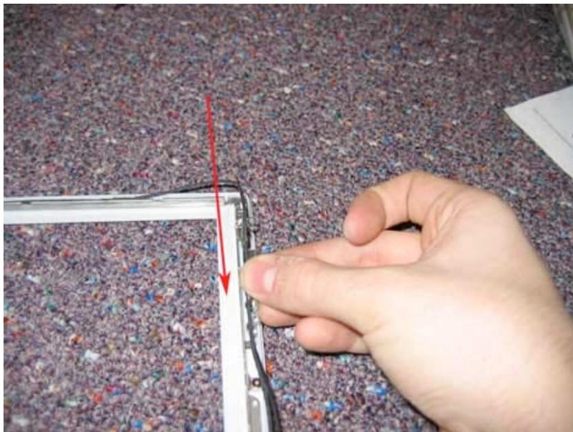
Now, on the left hand side, repeat the procedure. Remove the two Philips head screws from the locations shown below.
