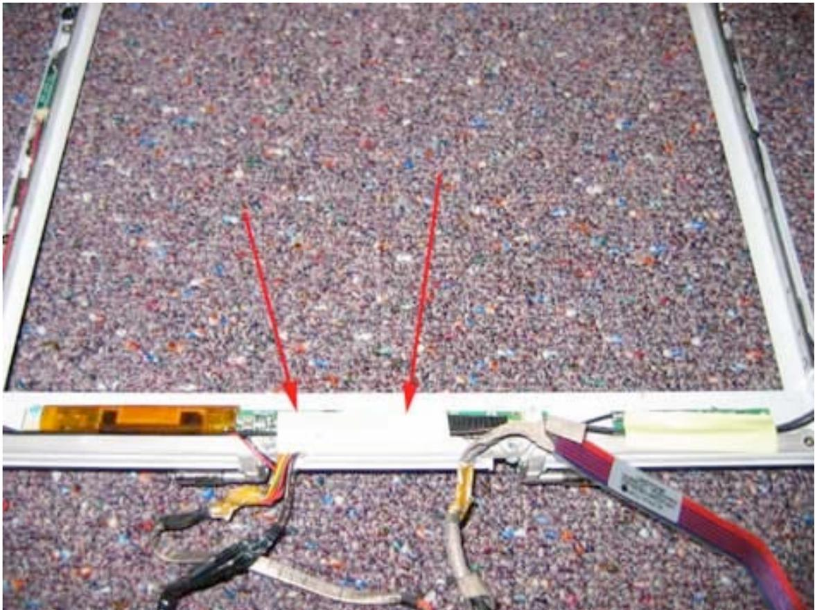
Undo the inverter cable connector from the inverter board by gently pulling the cable out.
