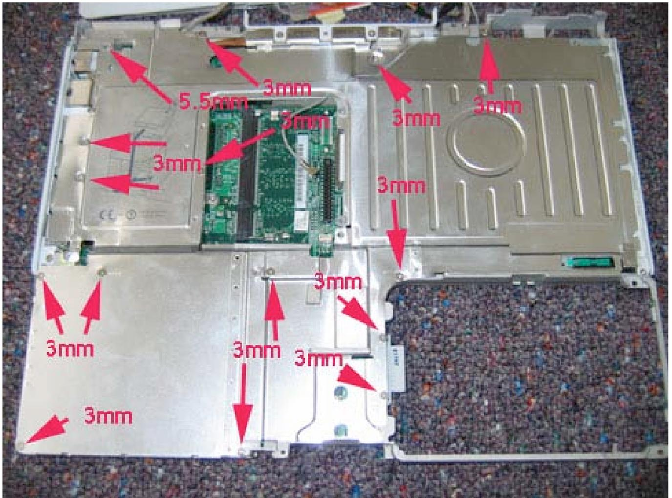
The top shield can now easily be lifted up and out of the unit as shown.
