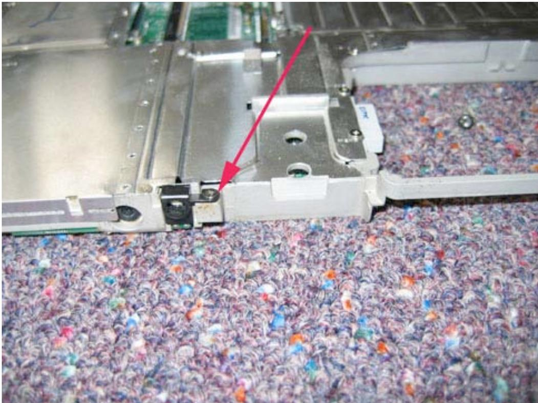
Flip the unit over and locate the cable going from the sleep light to the logic board. Gently pull this cable to free it from the logic board, and set the sleep light should come free easily.
