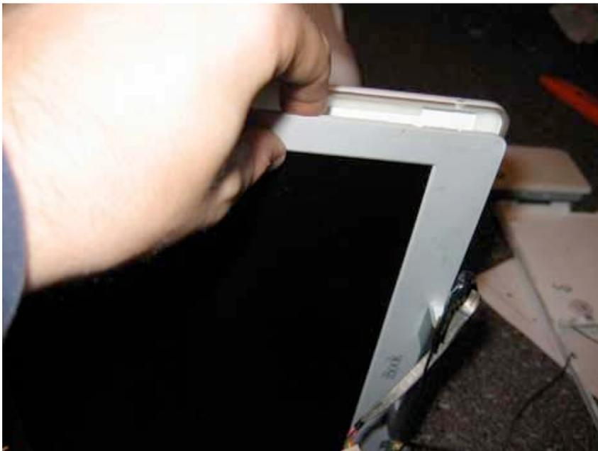
Lift the back casing off and away from the rest of the display module, and place it on a clean surface.
