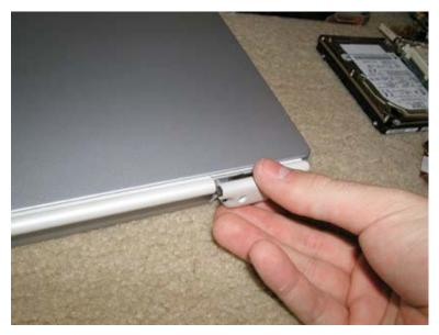
Gently pry the clutch covers off of the frame. If you use a flathead screwdriver be sure not to chip your paint. They should come off easily.
