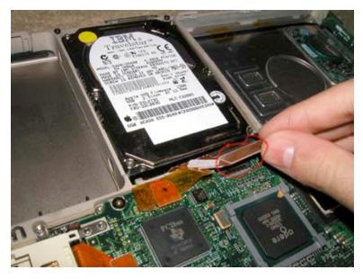
Disconnect the orange hard drive cable from the motherboard as shown.
