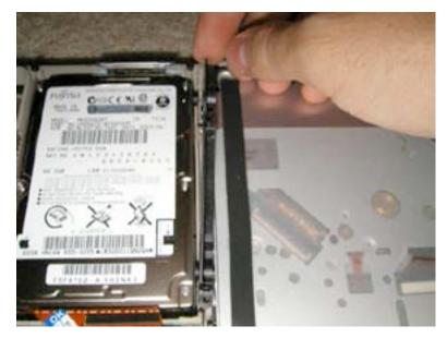
Lift the black plastic piece that was held on by the torx screws, up and out.
