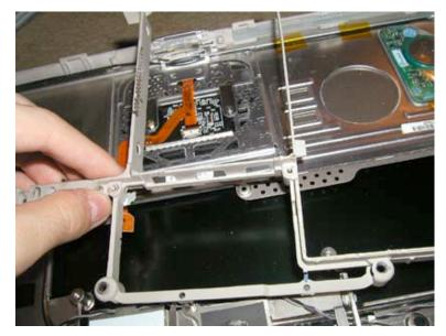
Gently lift the rib frame up and out.
