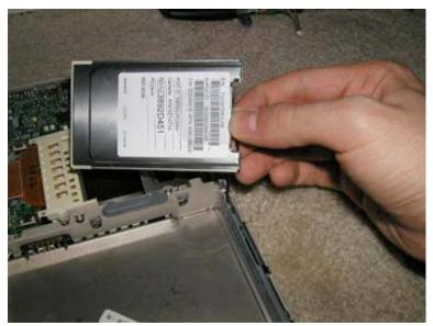
Using your fingers, pull the cable connector from the card. (If it is hard to pull the connector out, you can use a pair of needle nose pliers to gently pull the connector out while holding the card. If you do this, don't use much force at all or you risk breaking the card and connector.)
