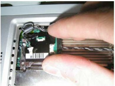
Pull the modem filter up, and remove the two cable connecting it to the computer.
