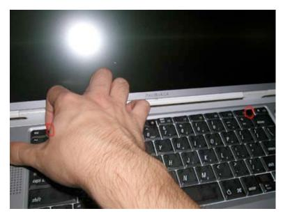
After you have removed the battery, turn the computer over and open up the display. Then, depress the two keyboard tabs as shown in the picture. Holding the tabs in, flip the keyboard up and towards you. (If the keyboard does not easily come out, check to make sure you have not locked the keyboard.)
