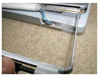
Line the epoxied hinge up with the hinge hole.
