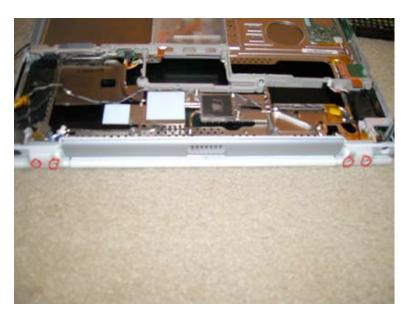
Remove the 4 Torx T8 screws on the clutch covers as shown.
