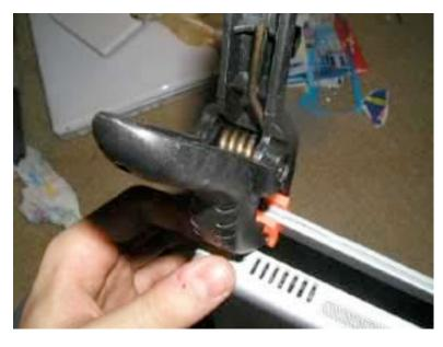
Use a strong spring clamp (available at Wal-mart) to clamp the display shut. Only clamp the edge of the display! Do not put the clamp on the actual LCD or you will break it. Let the epoxy sit for 24 hours or as the instructions say. 24 hours is a good time to let the epoxy sit however.
