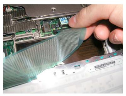
To remove the keyboard connector, grasp the cable as shown and gently pull up. You can gently wiggle the cable from side to side if it doesn't come off easily. Do not use much force. It should come off relatively easily.
