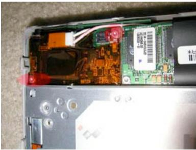
Remove the two Torx T6 Screws as shown.
