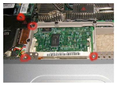
Remove the four Torx T8 screws as shown.
