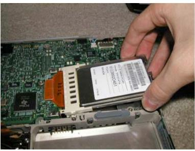
Lift up on the card as shown. Then pull the card out of its connector. (You may gently rock the card side to side to ease it out of the connector.)
