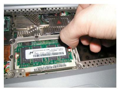
To remove currently installed ram, pry back the metal or plastic fasteners holding in the ram as shown. Do this on each side. It's easier if you do them at the same time.
