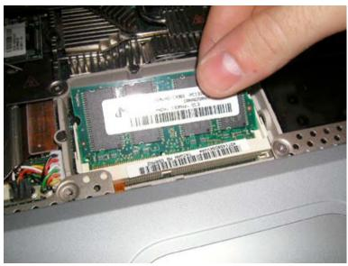
The ram chip will pop up. Just slide out to remove it. To install a new chip, just align the new chip in the grooves, press in, and then press down until the fasteners clip on both sides.
