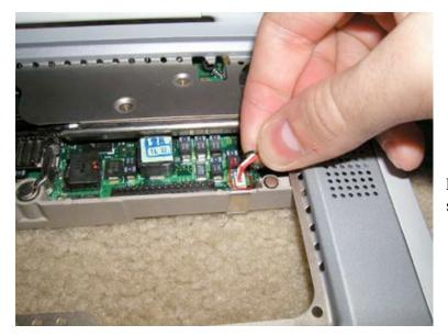
Remove the backup battery cable as shown by gently pulling up.
