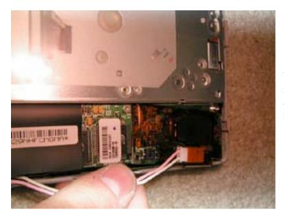
Unplug the inverter cable from the inverter board. Lift the board up and out and place on a static free surface.
