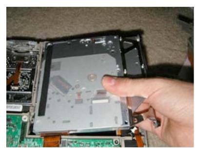
Grabbing the drive from the sides only as shown, lift the drive up and out.
