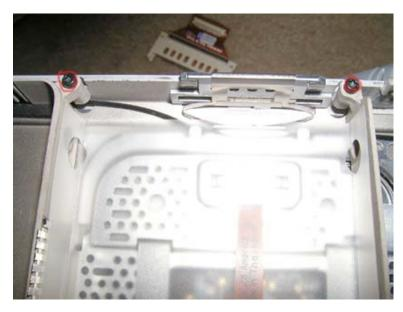
Along the rib frame there are 4 small torx T8 screws. The two shown to the left are in the hard drive cage. The one in the picture below is under the airport cable near where the airport card goes. The last picture is hard to tell, but it is near the inverter board on the left hand side of the casing.
