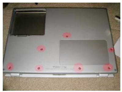
Remove the 7 Torx screws from the bottom case with your Torx T8 Screwdriver. (Available from www.powerbookmedic.com)
