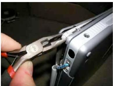
Use a pair of need nose pliers to pull the hinge towards you and out. Note: Do not use much force. You want the hinge to come out easily. If you use too much force the hinge will break and extraction will be much more difficult.
