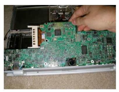
Grasp the logic board as shown and gently pull up. Then gently pull the board out and place it on an anti-static surface.
