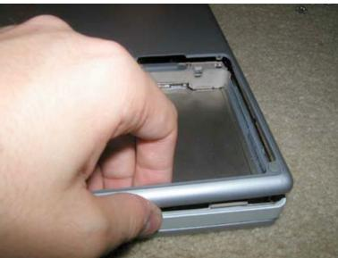
Gently lift up on the case as shown. Do not use much force at all or you will break the trackpad casing. Gently work your way around the casing.
