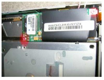
Turn the computer back over and remove the two torx T6 screws holding the modem as shown.
