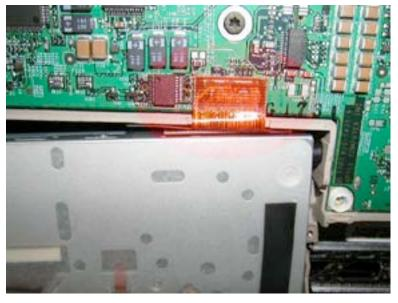
Remove the orange cable connecting the optical drive to the motherboard as shown.
