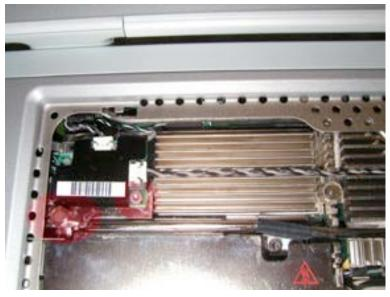
To remove the modem filter, you will need either a pair of pliers or a 5mm hex nut screwdriver or wrench. Undo the hex nut as shown.
