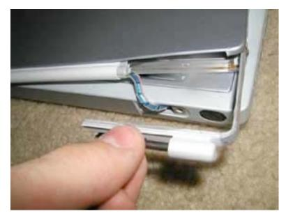
Guide the hinge into place. Make sure the hinge goes all the way back and then fits snugly into its corner.
