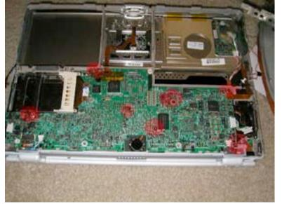
Remove the 7 Torx screws as shown \
