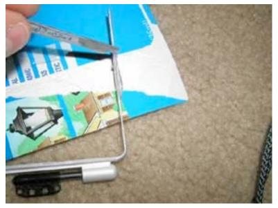
Apply the epoxy to the hinge. Apply enough to thoroughly coat the hinge, but not enough so that it drops off the hinge or that there are big gobs. If you use too much you could damage the display. Also, BE CAREFUL with the epoxy. Do not get the epoxy on your display or you will damage it. Make sure you only get it on the hinge and the area it needs to go in.
