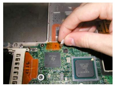
If a strip of orange tape is covering the trackpad connector, remove it as shown and disconnect the trackpad cable from the motherboard. If you have not already done so, remove the hard drive cable from the motherboard as well. (It is located next to the trackpad cable.)
