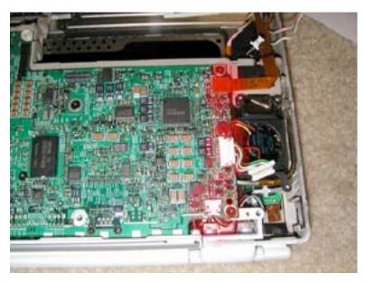
Remove the inverter cable, modem cable, and DC-In cable, as well as the black and grey cable on the bottom right of the logic board. if you haven't done so already.
