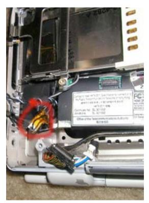
Disconnect the audio cable on the left hand side and right hand side of the unit. If it is wrapped in orange tape, remove the orange tape.
