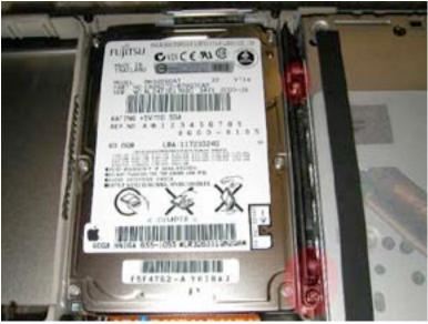
Remove the two Torx T8 screws shown in red.
