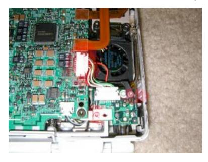
Remove the DC in board cable connected to the logic board, and the two torx T6 screws as shown.
