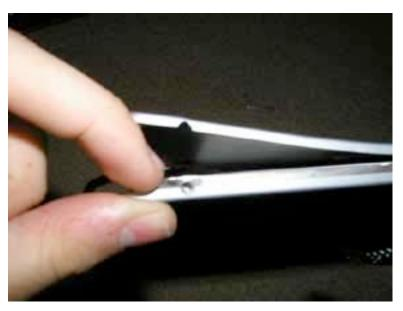
A lot of times, you will damage the thin piece of metal that connects the top casing to the bottom casing. When you close your display back, it will normally go back into position, but you may have to prod it in certain places with a flat head screwdriver to allow the casing to close correctly.
