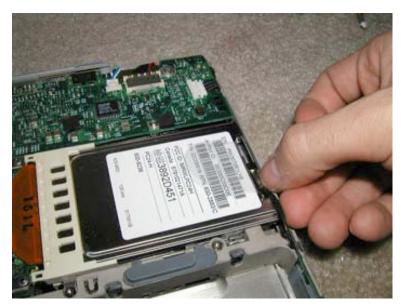
To remove the airport card locate the metal clip that holds the cable connector in place. Gently pry this back with your finger and pull up on the cable to release it from the connector.
