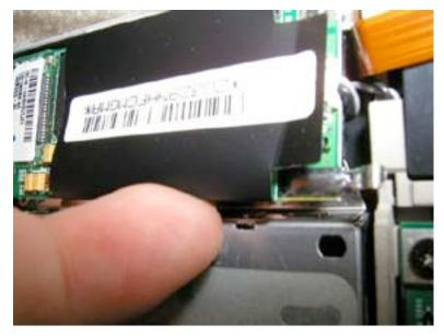
Gently lift the modem up from the side to allow access to the grey and black wire going to the modem. Then undo this cable from the modem.
