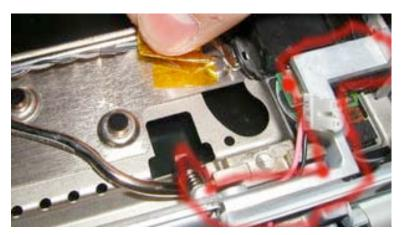
On both sides of the casing is the piece shown in red. This piece pivots up and "folds" over.
