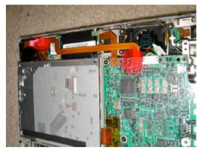
Remove the inverter cable from the places shown simply by lightly prying up on the cable at both ends.
