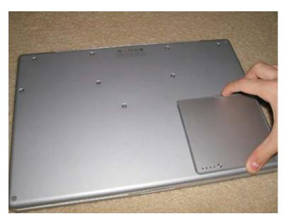
Turn the computer over with the bottom up as shown. Push the battery latch to the right as shown. The battery will then "pop" up and you will be able to remove it from the laptop as shown in the second picture.
