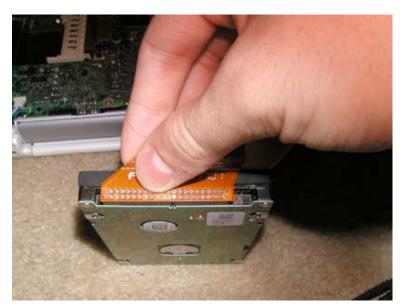
Remove the orange cable from the hard drive by pulling the cable straight up as shown. Do not use excessive force or you will bend the connector pins.
