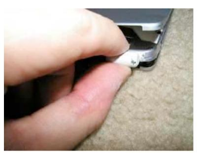
If you haven't done so already, follow the instructions above to break the bond on about 3-4" of the casing on the side of the casing of the hinge you need to replace.
