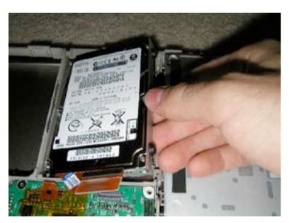
Tilt the hard drive as shown, and lift up and out.
