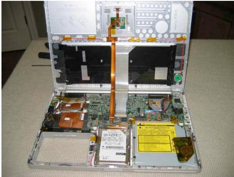
Undo the keyboard connector and trackpad connector by carefully pulling them out of their logic board connectors. They are located in the middle of the logic board as shown in the picture below.
