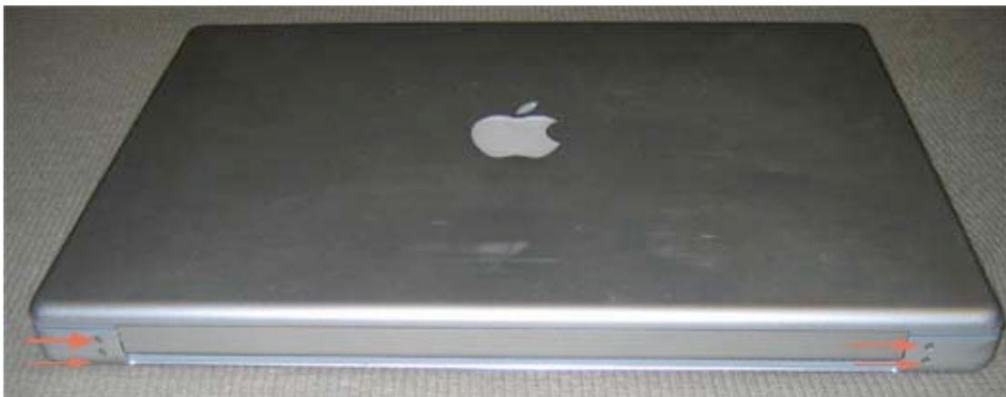
Now, make sure the display on your unit is closed, and flip the unit over with the display side on your work area. Remove all of the screws in the locations shown. The screws are as follows: 2 Philips silver 1/8" screws inside battery bay, 4 Philips 5/8" screws on the top lined in a row, and 4 Philips 1/8" screws on the ram cover.
