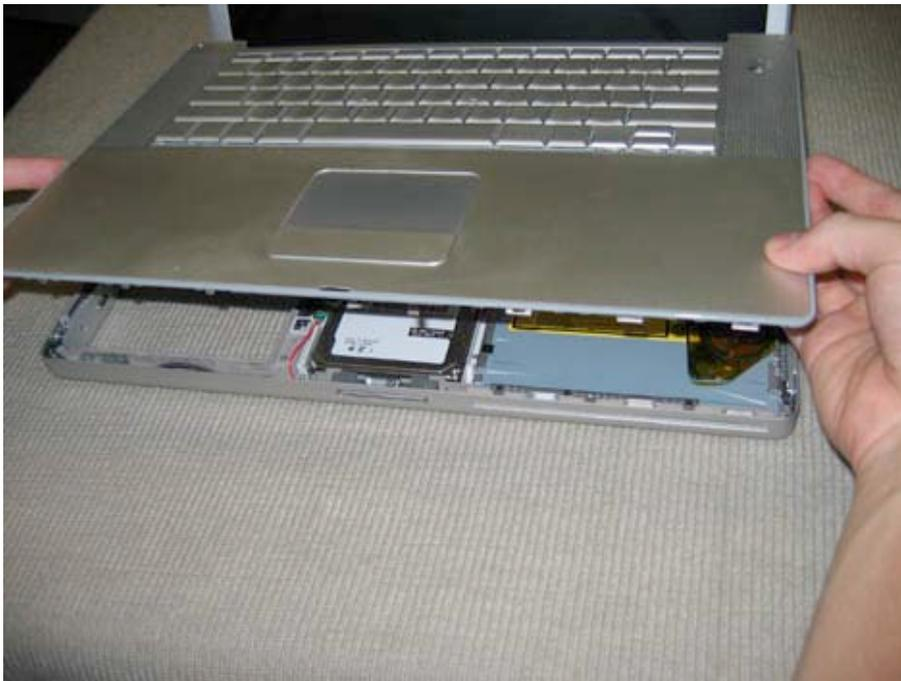
If you are having problems with the bottom right hand corner, then you may need to unlatch 3 latches located in the drive bay. You unlatch these by placing a flat plastic tool in the latch locations and then pulling the latch towards you. You can notice the locations of the latches by the slits in the drive bay dust shield (the gray cloth) The locations are shown below as well.
