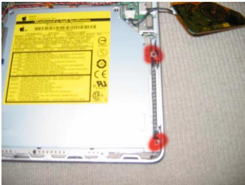
Grasp the drive from the back left hand corner, and gently lift the drive up and out and place it on a static free surface. The drive should come out very easily.
