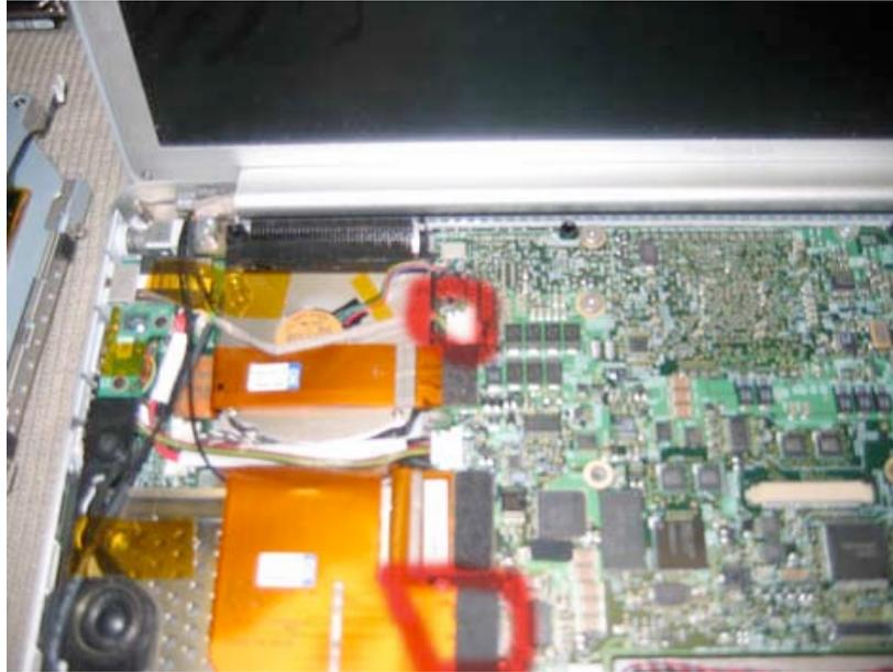
Next, pull back the orange cable as shown in the picture below to reveal the airport cable connection. You'll notice a fat spot in the cable. This is where the two airport cables connect. Pull on either side of the fatter spot in the cable to undo the cable.
