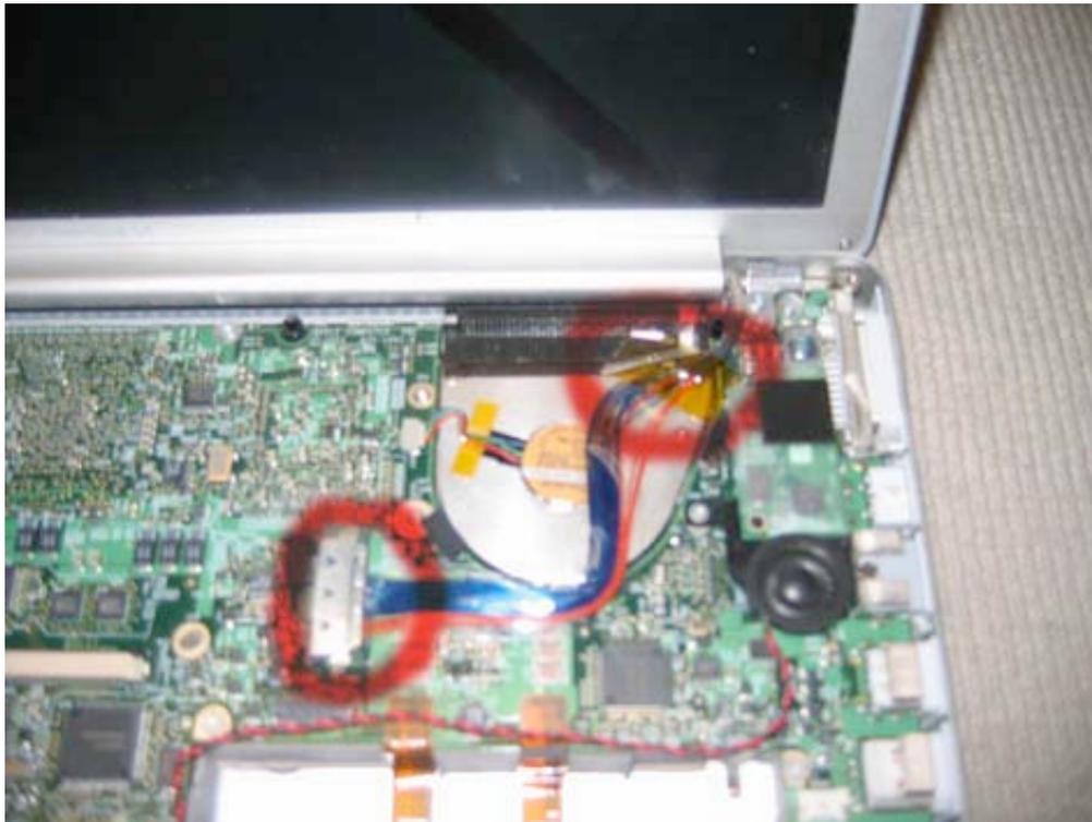
Next, locate the two torx T8 screws on the display hinge as shown in the picture below, and remove both of them. The hinge in the back is 3/8", and the hinge in the front is 1/2".
