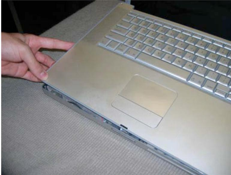
Now lift up on the right hand corner of the palmrest, and the whole assembly should easily lift up.
