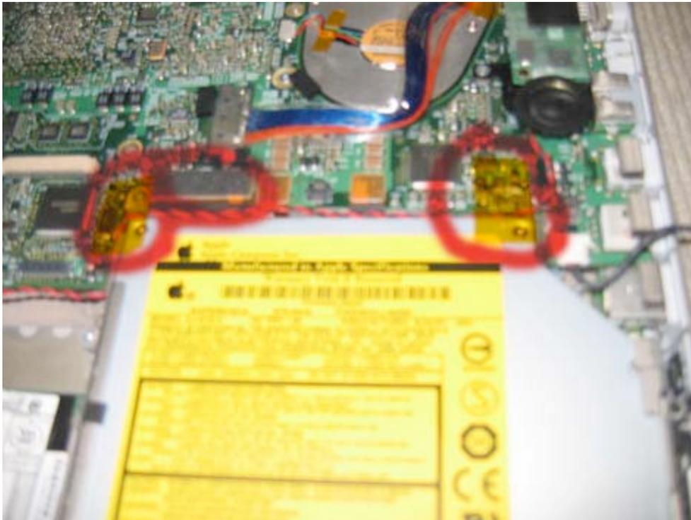
Next, remove the two black 1/8" Philips head screws from the side of the drive (casing side) in the locations shown by red circles in the picture below.
