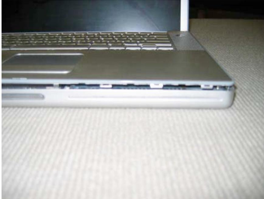
Flip the Palmrest assembly up and back, and gently rest it on the LCD
