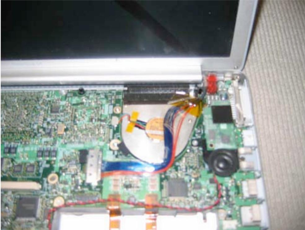
On the left hand side, begin by removing the two pieces of orange static tape in the locations shown in the picture below.
