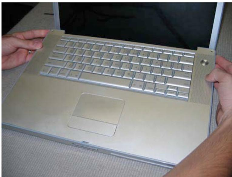
When the two back corners are freed, work around to the bottom left hand corner, and pry it up in the same manner as the back two corners.
