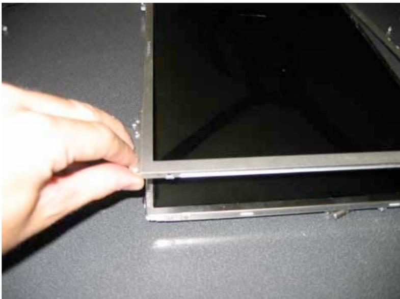
Now you must remove the display front bezel from the LCD. The bezel is held on by a semi-strong adhesive. You have to pull up on the bezel with slight force to remove it from the LCD.
