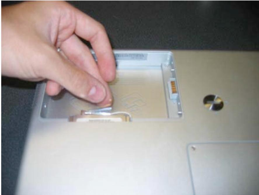
Now you need to undo the airport connector from the airport extreme card. This is most easily accomplished by grasping the connector with pliers and pulling out gently, but can also be accomplished with your fingers as shown in the picture below. You need to be as careful as possible with this cable.
