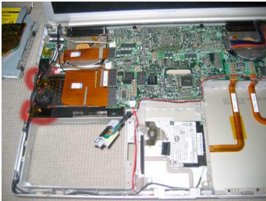
Now, follow the black cables around the corner of the battery bay and notice that in the crevice there is a green circuit board covered in clear plastic. This board is the Bluetooth connector board, and it will easily pry out by placing a screwdriver underneath the board and lifting up as shown in the picture.
