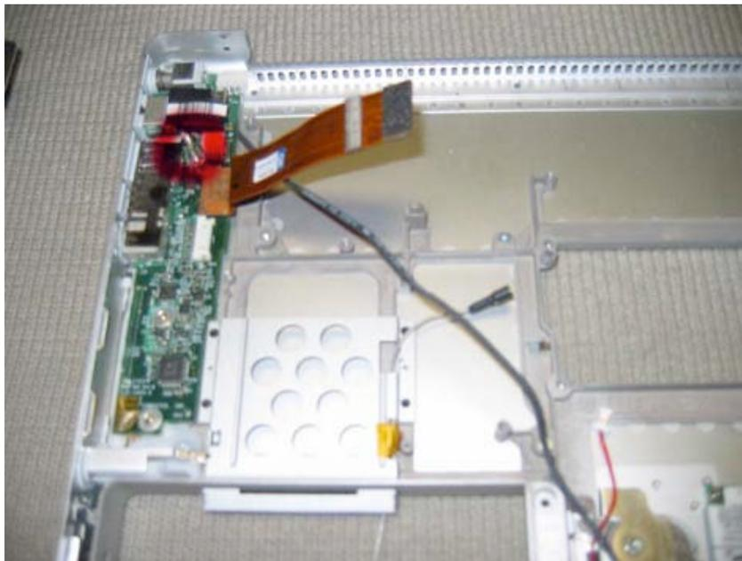
Now, lift the DC board up, and rotate it so you can view and remove the connector cable attached to it as shown in the picture.
