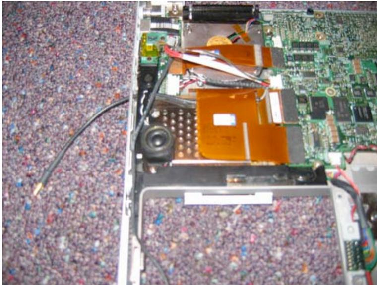
Connect the other cable in the QuickerTek Package to the one you just installed. (The connection is circled in red in the picture below.) Then adhere the antenna to the top corner of your display as shown in the picture below. Close up your unit, and you're ready to boost your reception!
