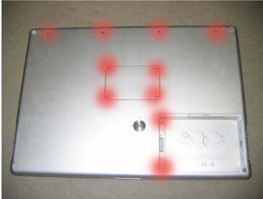
Lift the ram door cover off, and remove the two Philips head silver 3/8" screws in the locations shown. These screws will require a larger Philips head screwdriver than used for the screws in previous steps.
