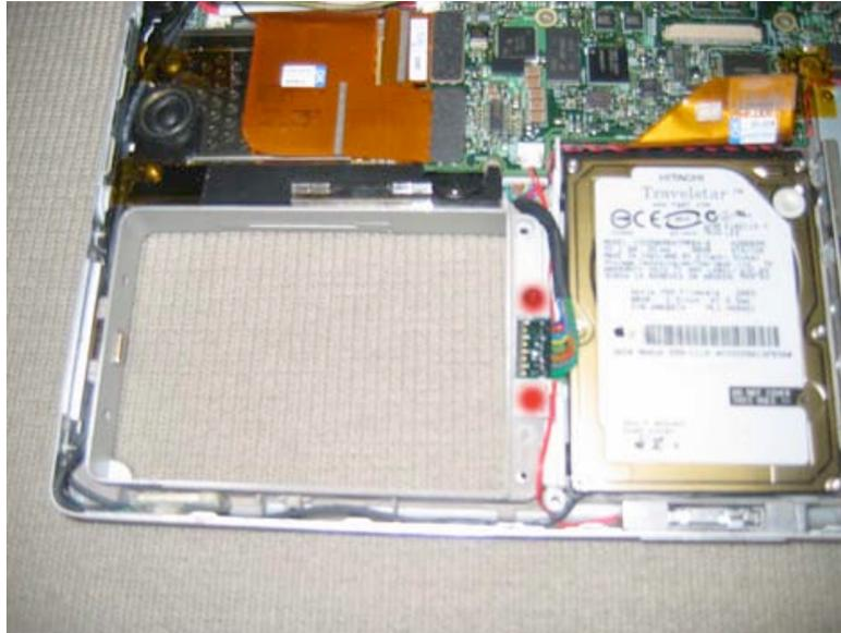
Pull the battery connector cable up and out of the way as shown in the picture. This will reveal two silver Philips head 1/8" screws in the locations shown by red dots in the picture. Remove these two screws.
