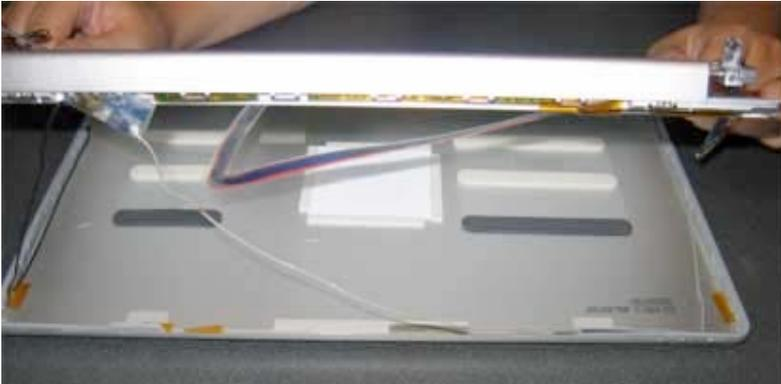
Once you separate the back case from the front bezel, lift the display off of the back bezel as shown, and flip it over. The grey cable and black cable will still be holding the two pieces together.
