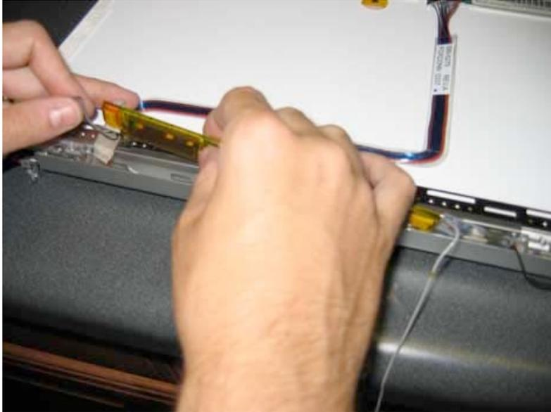
In the groove in the bottom of display is a long green board (the inverter board) Lift the inverter board out of the groove as shown.
