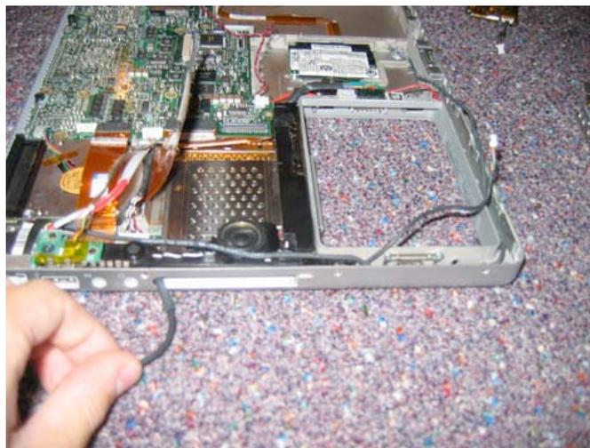
Reattach the orange cable to the logic board, and you should be looking at a similar picture to the one below.
