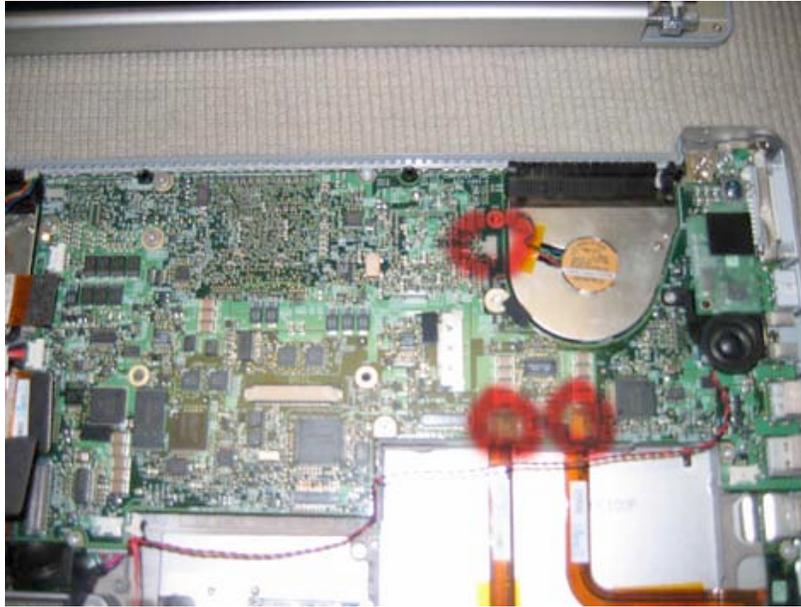
Now for the screw removal. Remove the 3 Philips 1/4" large head screws in the top left hand corner, one 1/8" silver Philips head screw in the bottom left corner, one 1/8" silver screw in the middle bottom and one in the middle top, one next to the right hand side fan, one in bottom right hand corner, one 3/8" silver screw in the top right corner, and one 1/4" silver Philips screw on the right hand side of the logic board next to the speaker. There should be 10 screws in total.
