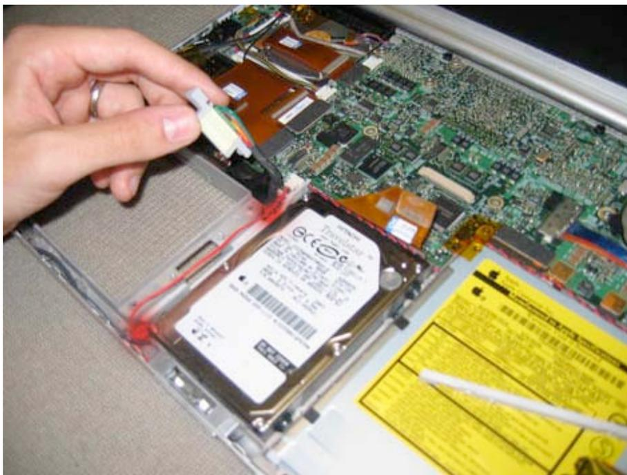
Carefully lift up on the hard drive and the plastic divider that you just remove the screws from. Guide the hard drive cable UNDER the speaker wire cable as shown in the picture. The drive should come out easily after the cable is guided under the speaker cable. If the drive does not come easily, do not force it as it is probably caught on the speaker cable.
