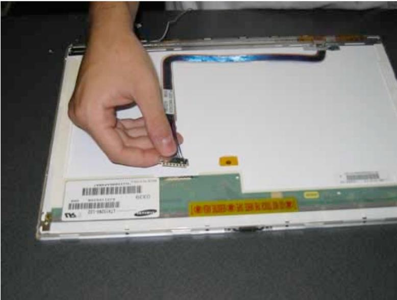
Undo the display cable from its connector by gently pulling it towards you. It should come out very easily.
