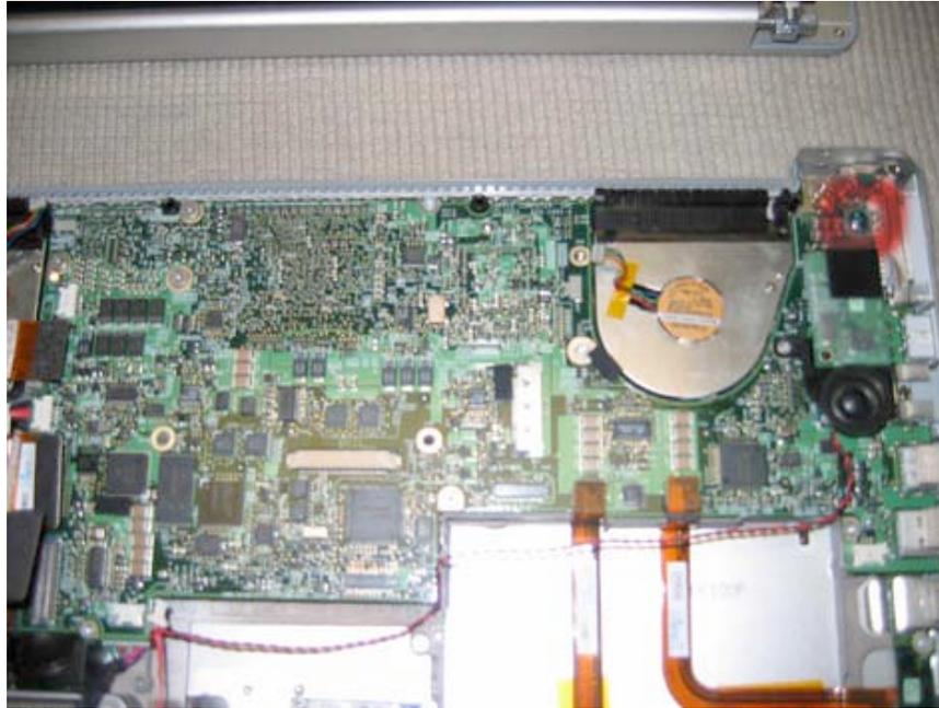
Now, on the left hand side of the logic board, unplug the double black and double red wire from the DC in board. It isn't necessary to undo this cable from the logic board.
