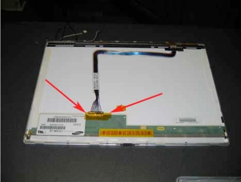
Remove the piece of orange static tape holding the display cable in place.
