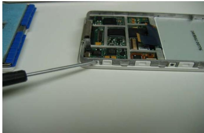
The rest is just putting the screws back in, connect the LCD, the headphone ribbon cable, the hard drive, and then the battery in reverse order of taking it apart. Once all that is connected, just take the back case, make sure it is right side up and snap it back to the top, and you are done.
