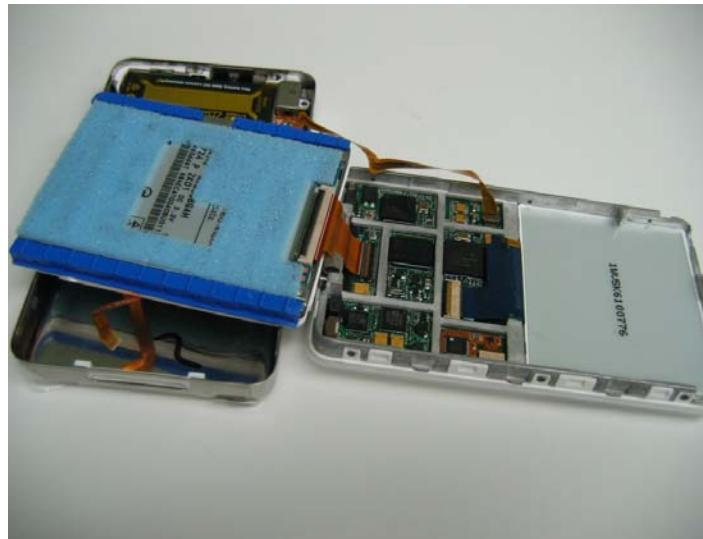
You can then flip the hard drive straight back towards the docking port. This will reveal the rest of the ribbon cables and the logic board.
