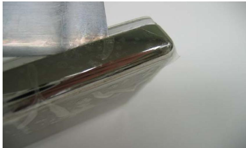
Get your tool in between the front plastic casing and the back metal casing. The thinner the tool the better you will be. Thin flathead screwdrivers and small putty knives tend to work best. You may need to use a lot of pressure to make sure the tool doesn't slip.
