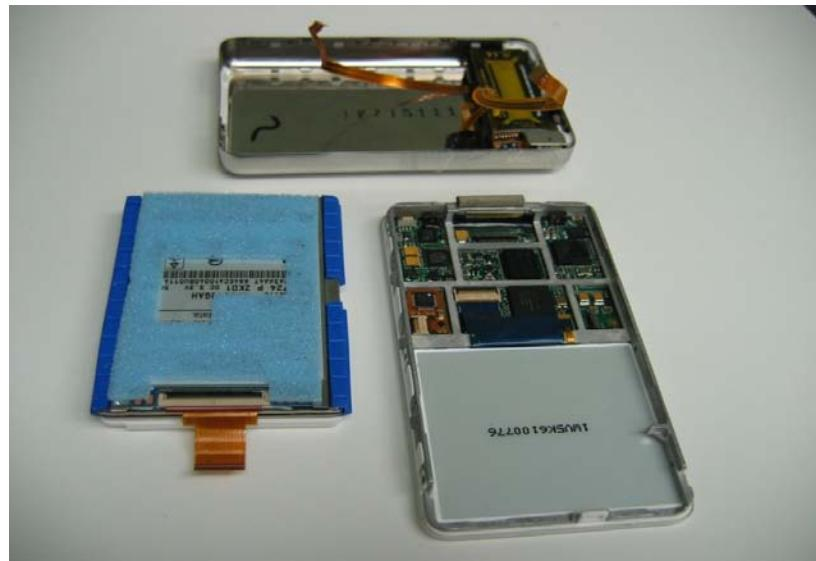
You should now have three separate pieces. The back case, the main body, and the hard drive.
