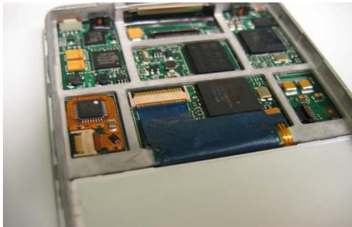
The cable (blue in the picture above) can be removed the same way as the others. Flip up the clip (black in this case) and slide the cable out.
