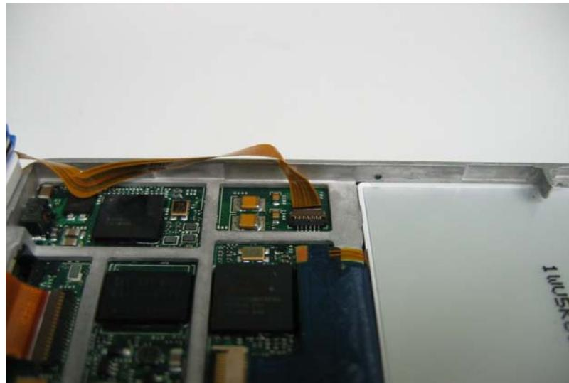
Disconnect the headphone module ribbon cable by flipping up the clip (brown in the image above) and pulling out the ribbon cable.
