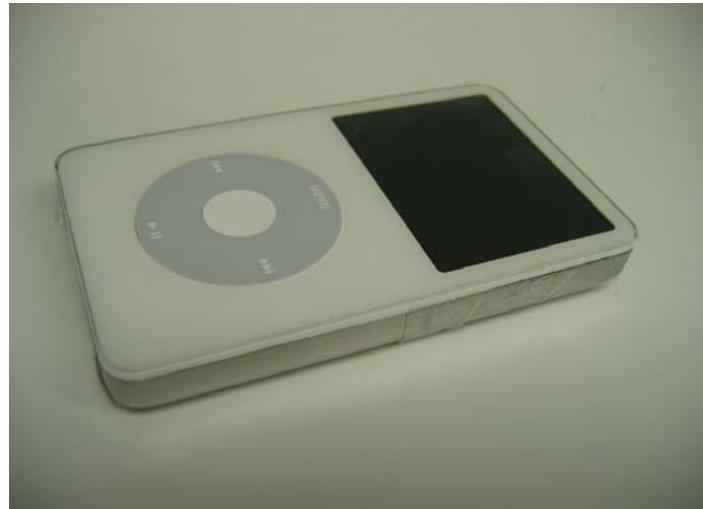
The metal bottom casing is very easy to scratch, so I recommend covering the area with tape so you won't damage the case if your tool slips. You should be able to see the tape in the picture above to the left of the iPod's LCD screen. This is the best place to begin opening the case.
