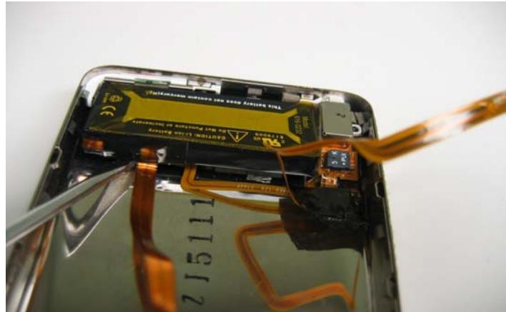
Use a flathead screwdriver and pry up underneath the battery. It is only held down with adhesive and should pop out. Make sure not to damage the ribbon cables.
