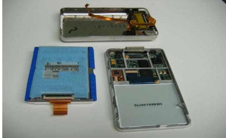
You should have the back case and the hard drive separated from the logic board as shown in the picture above before starting this section.
