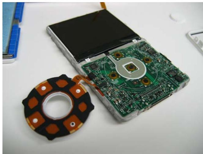
The front case should now be removed and you can now see the click wheel mechanism and the front side of the LCD and logic board. The click wheel has a little piece glued to the frame, you should be able to peel this off with no problem. You should now be able to push the logic board from the back and get it separated from the frame. The logic board does have some adhesive so it may take some more force to get it separated.
