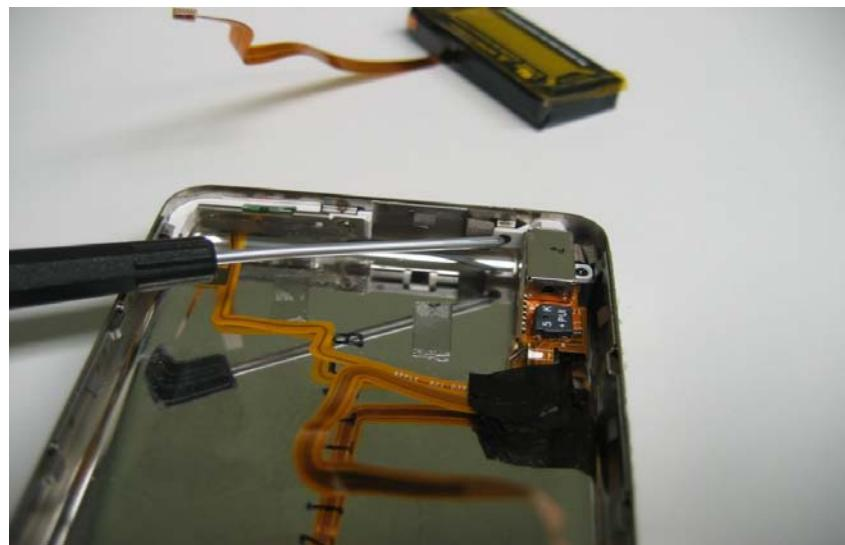
There will be five screws holding the headphone module in place. There are two on the headphone jack side and three near the hold button. Once those are out the module can be removed and the back case should be empty.
