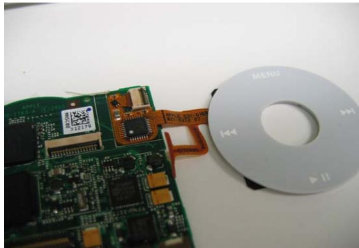
Once the logic board is separated from the frame, you can remove the click wheel ribbon cable from the logic board by flipping up the lock mechanism and pulling the cable out.
