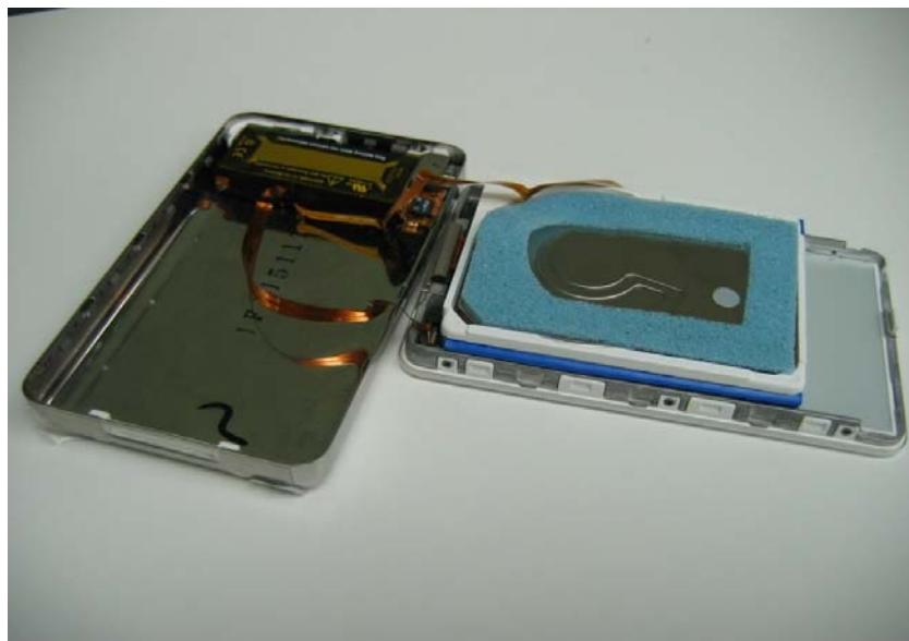
Once it is separable, you should be able to rotate the back casing around 90 degrees and be able to lay both flat like in the image above. Congratulations, you are now inside your iPod.
