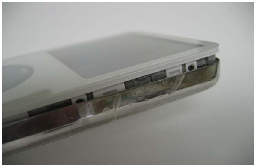
Work the tool down the side until it pops out like the picture above. Once it is at this stage just continue gently prying it open until you can fold the top case away from the back casing.
