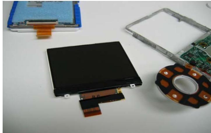
With the Front Case separated, the LCD should just come out easily. There may be some tape connecting the LCD to the frame/logic board. You can just peel the tape off.
