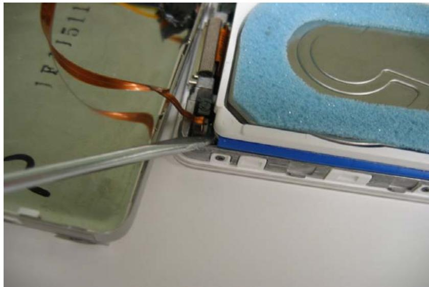
Use a flathead screwdriver and gently lift the clip around the battery ribbon cable to unlock it. Once the clip is lifted, you can easily pull out the ribbon cable disconnecting it from the logic board.
