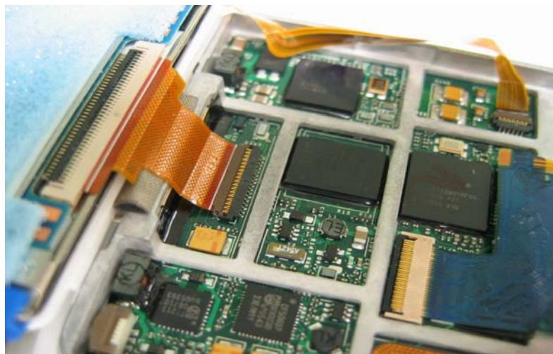
The picture above shows the ribbon cable from the hard drive to the logic board. The rest of the cables in the iPod uses this clip mechanism or a similar style. You need to flip up the brown clip to unlock the cable and then you can pull the cable out. If you are replacing the hard drive, you will also need to remove the ribbon cable from the hard drive. This is done in a similar fashion. Flip up the plastic clip (black in color in the image above) and pull the ribbon cable out.
