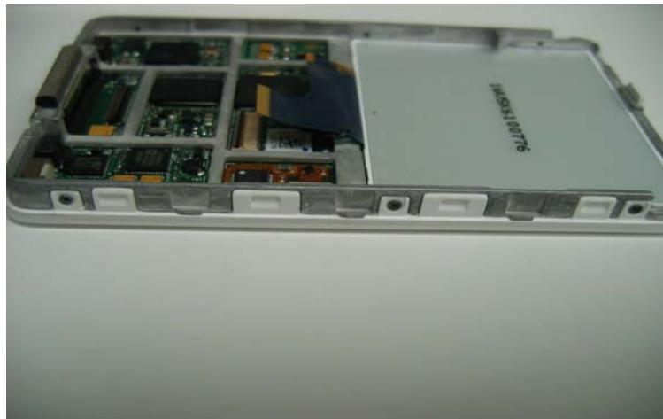
We now need to separate the front casing. There are a total of 6 philips head screws on both sides of the frame. (3 on each side) You can then pull the front case away from the frame, logic board, and LCD. There can be some adhesive so it may take a little more force. The click button from the click wheel may fall out at this point so make sure you are performing the repair where it won't be lost.
