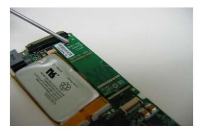
Remove the two screws and pull up on the module. There may be some adhesive on the board so you may need your flat tool to gently pry up the board.
