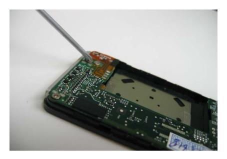
There are four screws that need to be removed on the logic board. There are three near the sync port and headphone jack. They may be covered with a sticker or tape.
