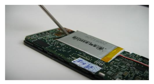
The first step is to dislodge the battery. It is held on by some adhesive along the sides. Just use your flat tool and gently pry up on the battery until it comes loose.
