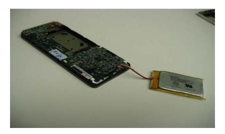
Once it is unstuck, you should be able to just flip the battery out. Be careful with the wires on the battery. They are soldered onto the logic board. If you pull to hard you could rip the cables and have to resolder.
