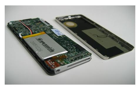
You should now have the back case removed. There aren't any cables connected to the back case. You can now see the back of the logic board.
