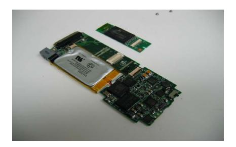
The daughterboard can now be separated from the logic board. Be careful on the socket connector. You can easily bend pins so remove it as straight up as possible.
