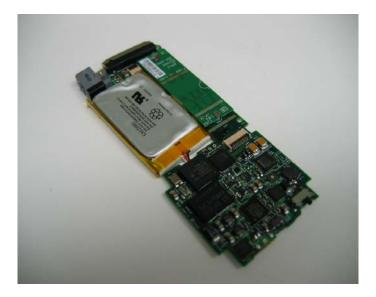
A 2GB model is pictured above. As you can see there is a daughterboard connected near the sync port. This daughterboard has the RAM on it. There are two screws holding it down.
