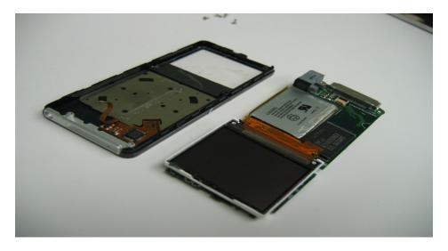
You should now be able to remove the front case from the logic board.
