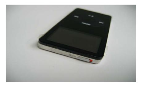
It is a good idea to stick some tape around the edge of the metal back casing right up next to the groove between the metal back casing and the plastic top case. It is quite easy to slip while you are using your flat tool and scratch the metal case. The tape will help shield the case from most accidental slips. The best place to start is wherever you feel most comfortable. It is recommended to not start near the headphone jack, hold button, and data port.
