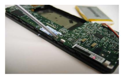
The fourth screw is near the middle of the board from top to bottom. It may also be covered by a sticker or tape. Once those four screws are removed, you can begin gently lifting the logic board. Be aware, there are some connections on the underside that can be easily torn.
