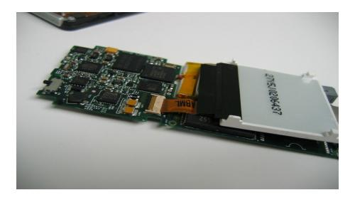
Disconnecting the LCD is the same way you disconnected the previous cable. Flip up the black locking mechanism, and gently pull the cable out.
