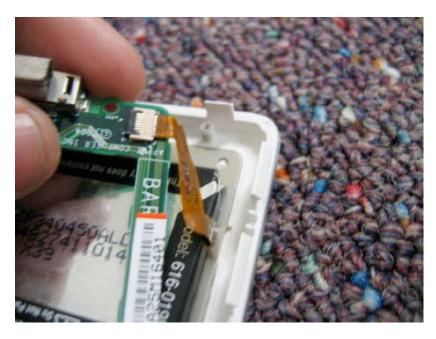
The logic board will now easily come free from the case. The LCD will still be attached to the logic board.
