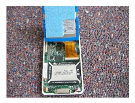
To remove the hard drive, grasp the cable as shown (thumb on top index finger on bottom) and gently pull the cable out (away from you and the connector)
