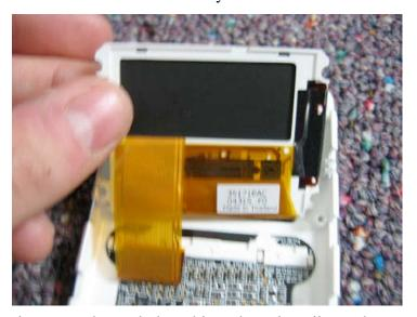
Use your flat tool to get underneath the cable and gently pull up. The connector should come free easily and the LCD will be free to be replaced. \*\* Note – Do not use your fingers to pull up on the cable as you may damage the display cable!
