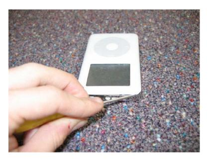
Continue separating the casing by gently prying up all the way around the unit. It should be much easier to pry the casing apart after you get the initial corner started.
