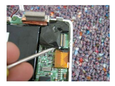
Use your flat tool to gently pry up on this cable to release it form its logic board connector. With the connector released, you will be able to remove the logic board from the body of the unit by simply lifting it up.
