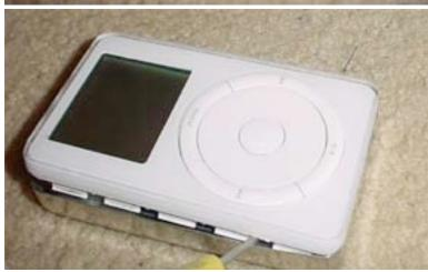
Use your flat tool to gently pry the casing up all along these notches to release the plastic casing from the metal pan.
