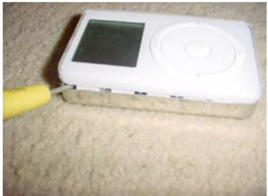
The case should open in a similar way to the picture on the left. Notice that the case has notches in the plastic.
