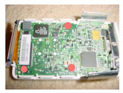
In the locations marked with red circles are 3 Torx T6 screws. Remove these 3 screws.
