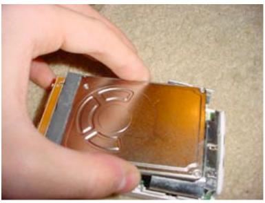
Immediately underneath the battery is the hard drive. Grasp the hard drive as shown and lift up.
