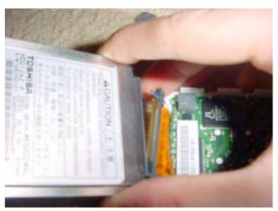
The orange cable going into the hard drive is the hard drive connector. Grasping the cable in one hand, and the hard drive in the other, the connector will easily come free from the hard drive.
