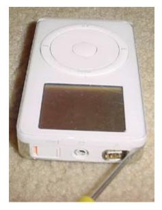
The initial step in the Ipod disassembly is the most difficult. We highly recommend using a flat blade nylon tool for this step to avoid scratching your casing.
