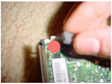
Right next to the hard drive connector there will be a rubber stopper in the shape of a square. Lift the stopper up as shown. This will reveal another Torx T6 screw that will need to be removed.
