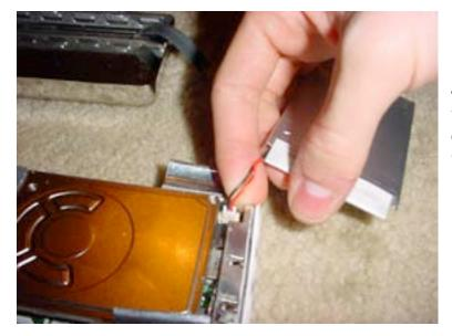
The battery is held on to the main board via a black and red cable. Gently grasp the cable and pull up to undo it from its connector.
