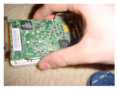
You can now lift the main board up and out of the plastic casing as shown.
