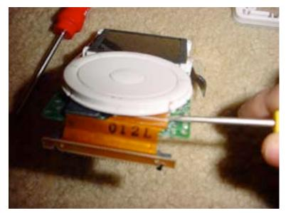
To remove the hard drive cable, use your flat tool to pry up on the other end of the connector cable as shown. The cable should come off easily. Be careful not to allow the screwdriver to slip as you do not want to damage the navigation device.
