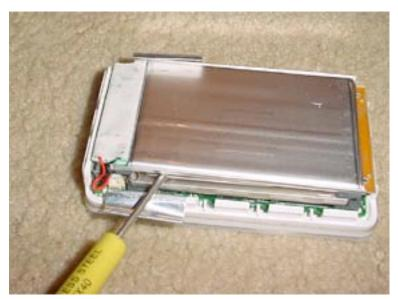
With the part flipped over, you will notice a thin shiny part. This is the battery, and it is adhered to the hard drive by two sticky strips, one on both ends of the battery. Use your flat tool to separate the battery from the sticky strip on both ends.
