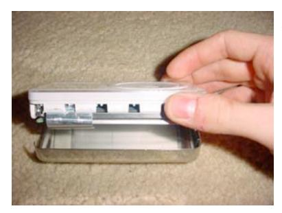
Tilt the plastic body up and out from the metal pan as shown.
