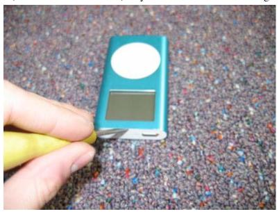
The plastic insert should come up and out as shown in the picture below.
