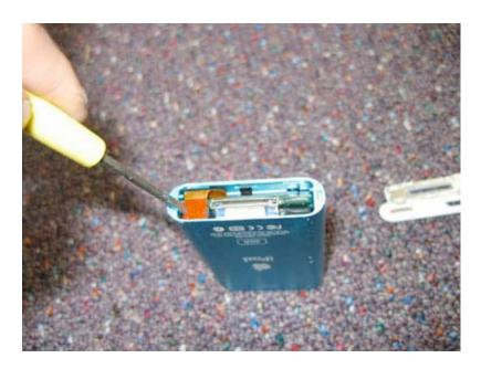
Place your flat tool in such a position that you can use it as leverage to pull with, from the top gently pull towards you until the whole assembly slides out of its shell. It should slide out easily.
