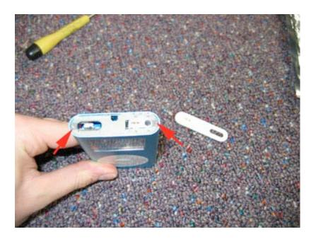
Repeat the procedure you used to remove the top insert to remove the bottom insert. It should come off easily as it is not held on by an adhesive.
